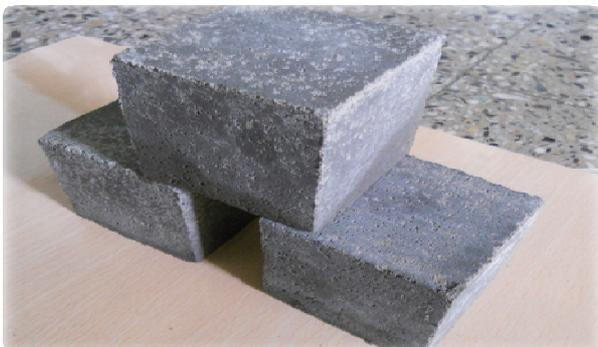
Fig. 2 Cube Specimen for Compressive Strength
