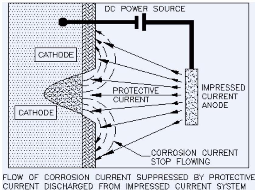
Figure 3.24: Impressed current system.
