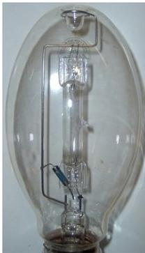
Figure 3.9: Mercury-vapor lamp.
