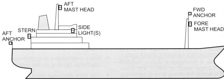
Figure 3.15: Ship's navigation lights arrangement.
