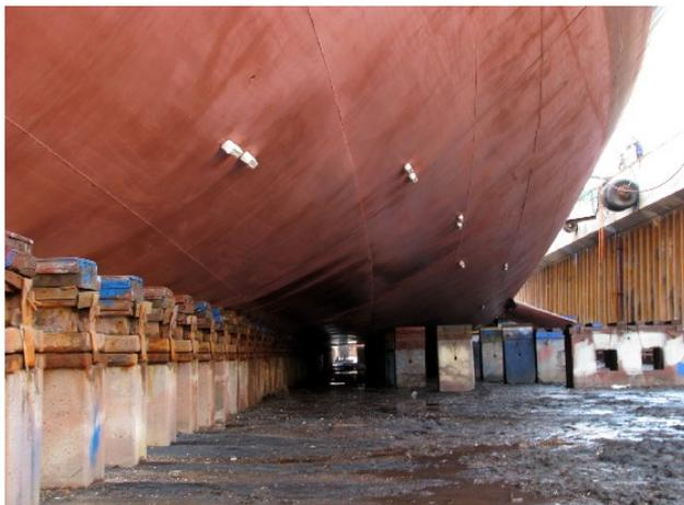
Figure 3.23: sacrificial anodes on a ship's hull.
