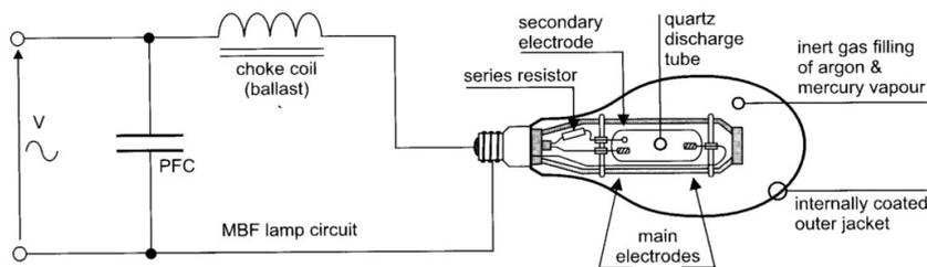
Figure 3.10: HP mercury-vapor lamp and circuit.
