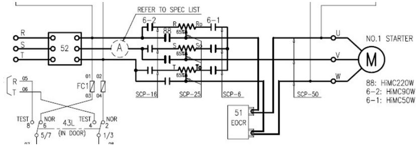
Figure 2.2: autotransformer starter main circuit
