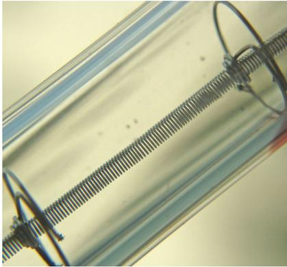
Figure 3.2: Tungsten-halogen lamp.
