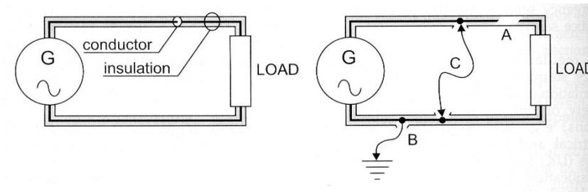
Figure 1.2: circuit faults
