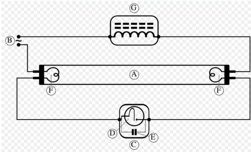
Figure 3.7: The preheat starter circuit.
