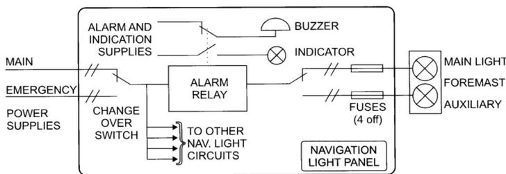
Figure 3.16: Navigation lights circuit.
