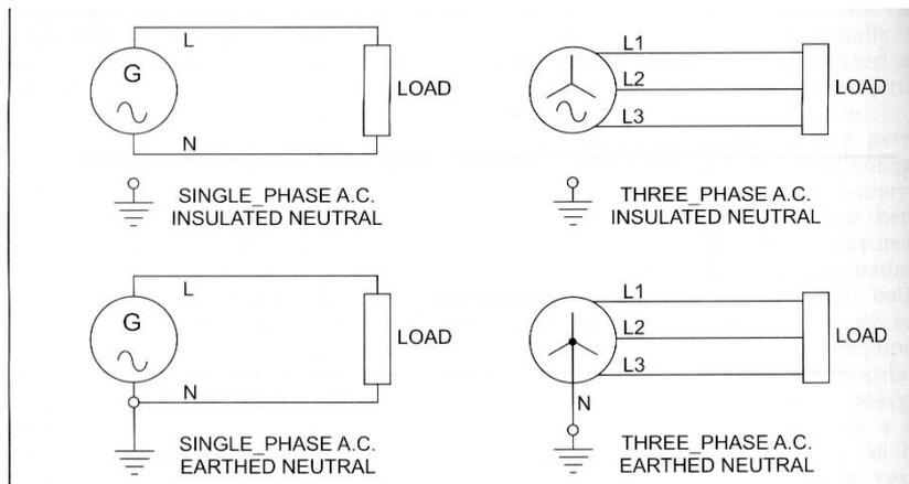
Figure 1.1: Insulated and earthed neutral systems.
