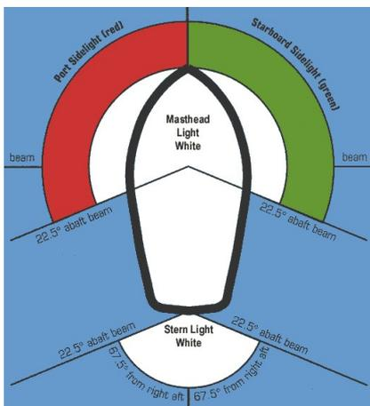
Figure 3.13: Ship's navigation lights requirements.
