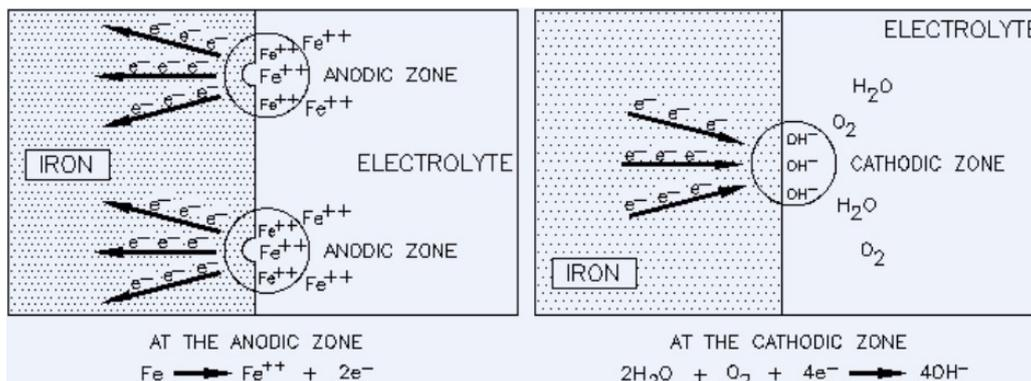
Figure 3.19: anodic reaction and cathodic reaction.
