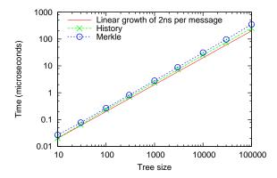
Figure 8: Time required, in microseconds, to build a Merkle or history tree, required before any signatures can be generated.
