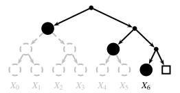
Figure 7: A pruned tree that authenticates message  $X_6$  that was generated during the batch ending in version  $X_6$ . Solid black circles are included in the proof. Grey circles need not be included because they are not relevant to the proof being constructed. Small dots can be recomputed from their children, so they need not be included.
