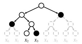
Figure 1: Graphical notation for a Merkle tree demonstrating the necessary hashes (solid black circles) to verify a Merkle signature on  $X_2$ . Open circles represent values that can be recomputed from the values below them. Grey circle nodes are unnecessary for the proof.
