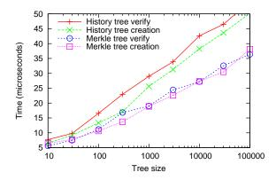
Figure 9: Amortized time, in microseconds, to generate and verify a membership proof in a Merkle or history tree as a function of the number of elements in the tree.
