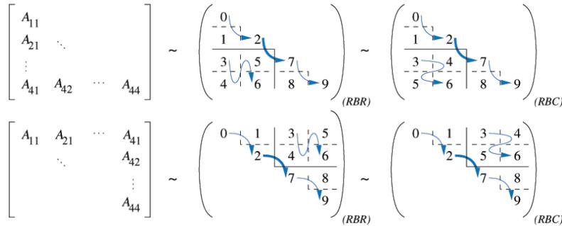
**Fig. 2.6** The mapping of a  $4 \times 4$  block triangular matrix in block column (BC) order, recursive block row (RBR) order, and recursive block column (RBC) order. Two levels of recursive splitting are used.
