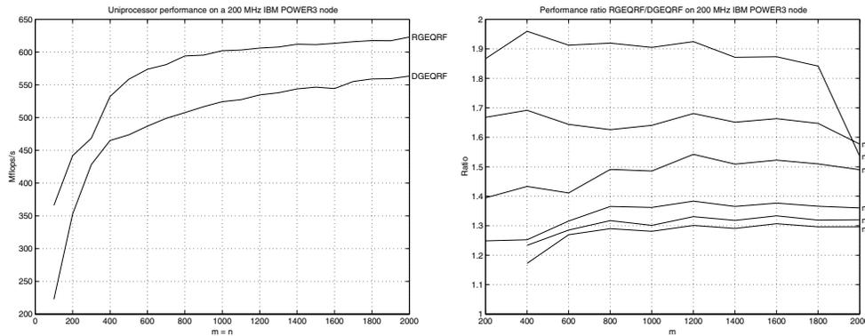
**Fig. 4.1** Performance results in Mflops/s for square matrices (left) and performance ratio for tall, thin matrices (right) for the recursive algorithm RGEQRF and DGEQRF of LAPACK on the 200 MHz IBM Power3.
