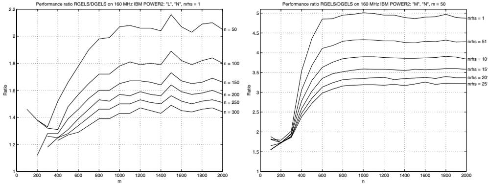
**Fig. 4.3** Performance ratio of RGELS to DGELS for computing the least squares solution with one right-hand side and varying  $m$  and  $n$  (left) and the minimum norm solution with  $m = 50$  and varying  $n$  and number of right-hand sides (right) on the 160 MHz IBM Power2.
