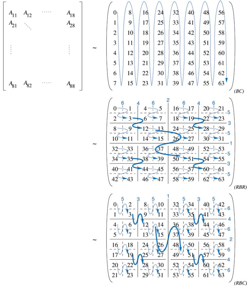
**Fig. 2.5** The mapping of an  $8 \times 8$  block matrix in block column (BC) order, recursive block row (RBR) order, and recursive block column (RBC) order. The three levels of recursive splitting are labeled 1-2, 3-4, and 5-6.
