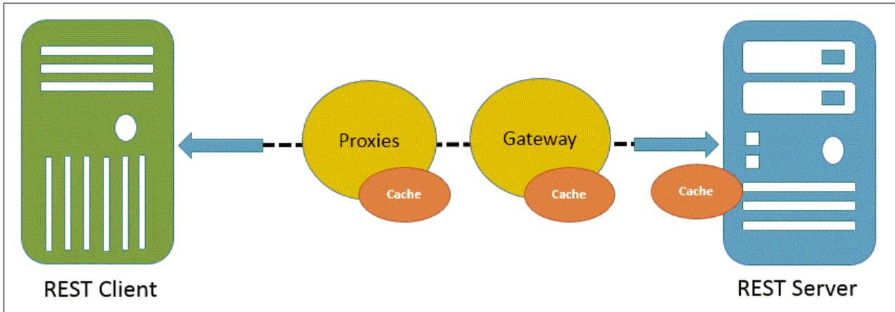
Figure 2-2 REST architecture with intermediary caches
