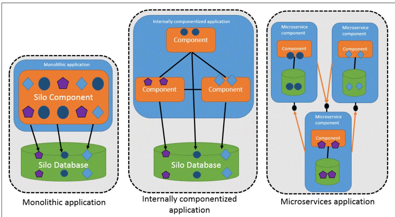
Figure 2-4 Monolithic and microservices application
