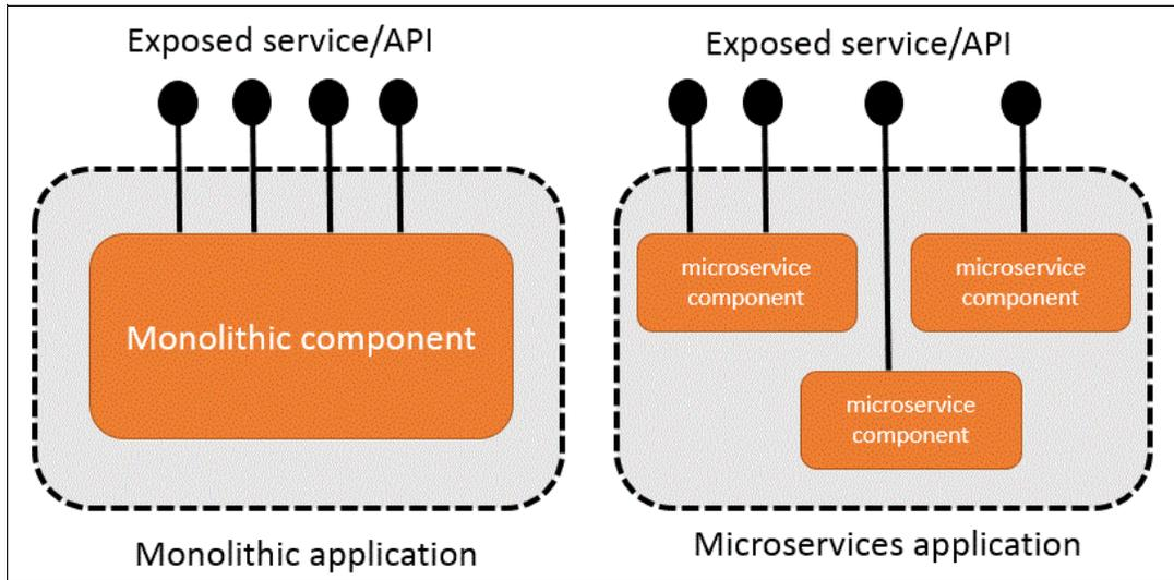
Figure 2-3 Monolithic versus microservices application
