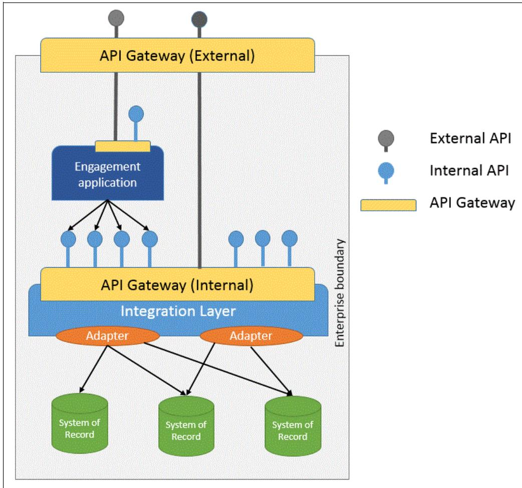
Figure 2-1 Exposing APIs externally and internally
