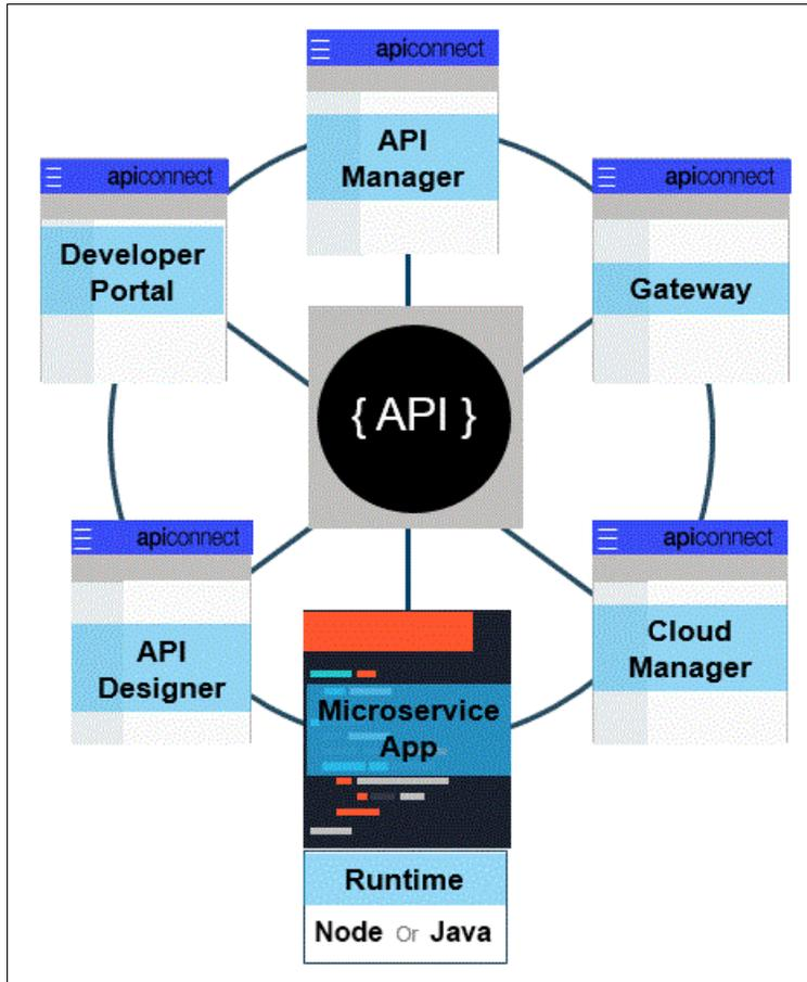
Figure 3-1 The components of API Connect in the API management platform
