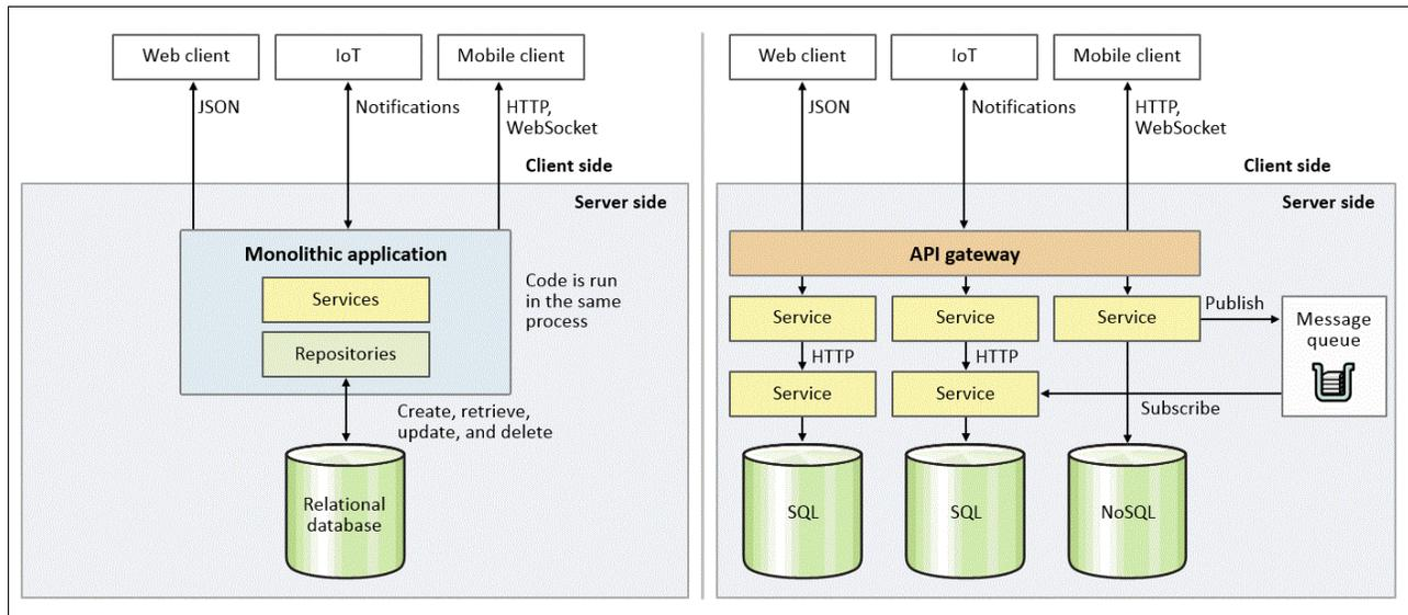
Figure 2-5 Monolithic versus microservices architecture
