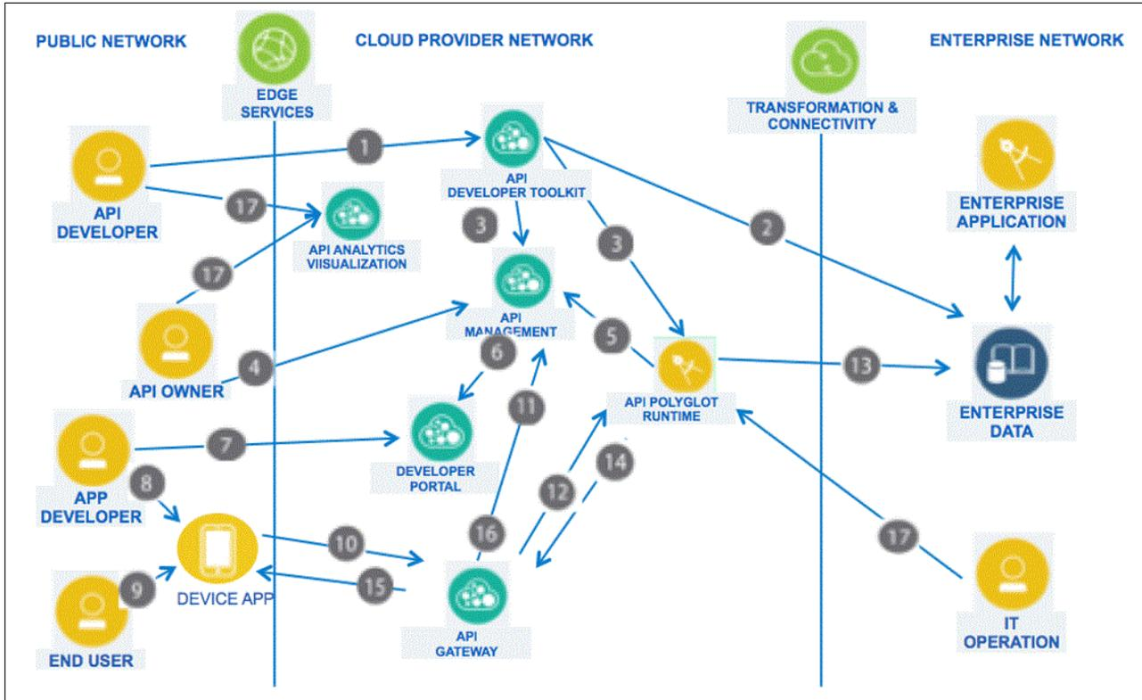
Figure 2-8 API management architectural components interaction
