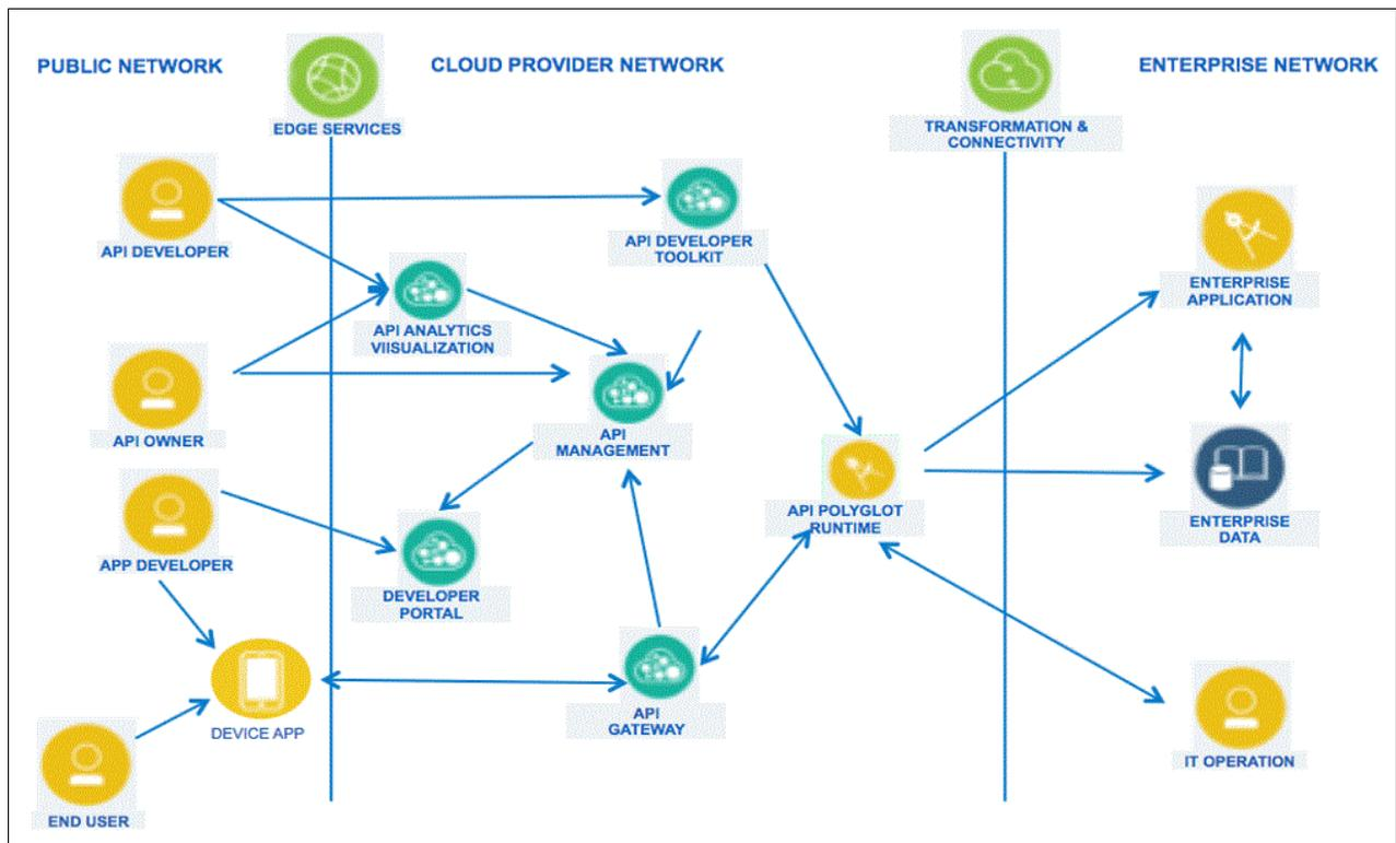
Figure 2-7 Components of API management platform
