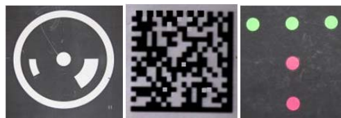
Figure 4.4 Three examples of coded targets used for point identification and camera calibration
