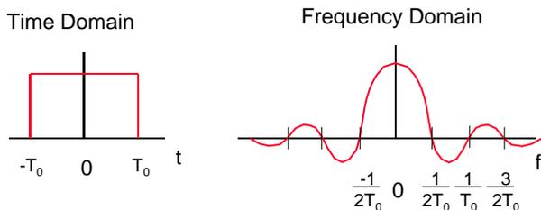
Looking at the effects from a different perspective we see the *edge effect* more clearly. Using this approach we can also see how to remove the edge effect by using a window that tapers to zero at the extremities.
