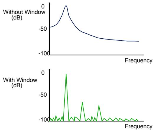
The windowing functions are typically developed from frequency domain requirements and a typical example is the Hanning Window, which is defined by the following equation :
