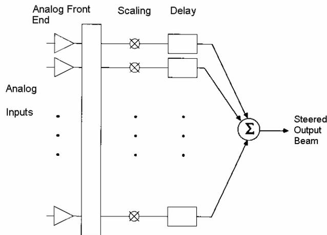
One of the limitations of time domain beamsteering is that one bank of delays can only steer the beam in one single direction. The solution is to use the fact that time delays in the time domain are equivalent to complex exponential multiplication in the frequency domain, using the following equation.
