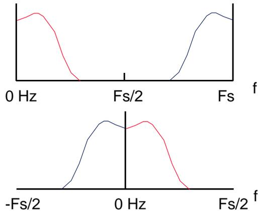
The first format is often used in baseband applications e.g. speech and system analysis, where as the second is more common in H.F. communication applications, where  $f_c$  is heterodyned down to D.C. The results are no different but sometimes make post processing easier.
