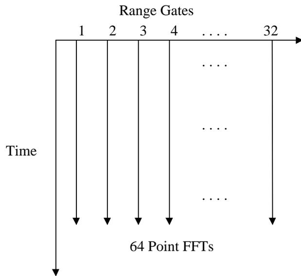
Range gate resolution (meters) = wavefront velocity \* sample rate
