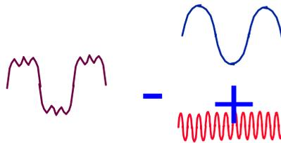
Signals can be transformed between the time and the frequency domain through various transforms. The signals can be processed within these domains and each process in one domain has a corollary in the other, as shown :
