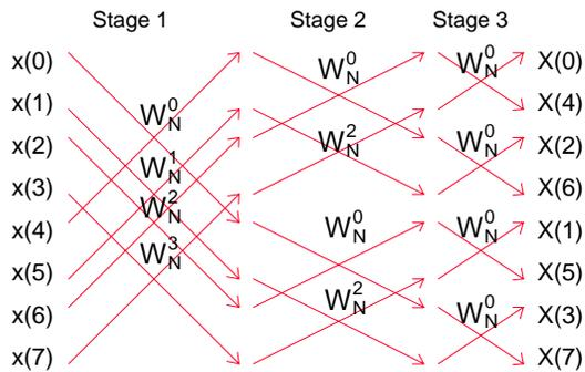
The  $W_N$  values are the coefficients of the FFT and are often referred to as *twiddle factors*. The twiddle factors are essentially the complex exponential values, according to the following equations.
