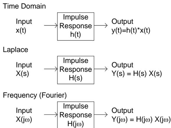
The most important process translation between the time and frequency domain is that convolution in the time domain is the equivalent to multiplication in the frequency domain and V.V.
