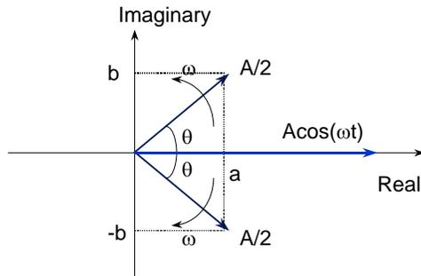
Phasors rotate in two directions and have the following characteristics. Positively rotating phasors rotate anti-clockwise and represent positive frequencies, whilst negatively rotating phasors rotate clockwise and represent negative frequencies.
