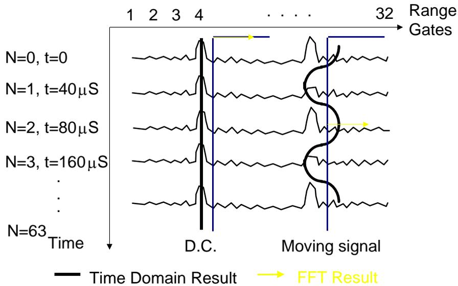
The sinusoidal result seen above is due to the phase of the returned pulses being modified by moving target. The D.C. signal is generated by the stationary target (the house). The moving signal is generated by the moving target (aeroplane). The magnitude of the FFT gives the size of the target, the FFT bin gives the speed of the target.
