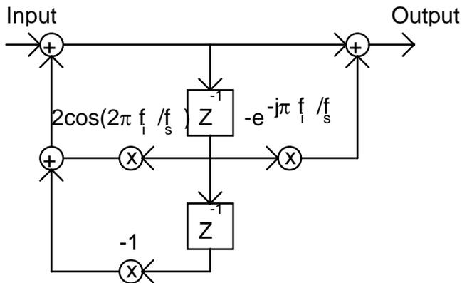
This filter does not maintain the complex (phase) information but the Goertzel filter is often used to detect particular individual frequencies, a common application is the detection of DTMF tones. This algorithm is very efficient, when compared with the regular FFT, especially when the requirement is only to detect a few individual frequencies.
