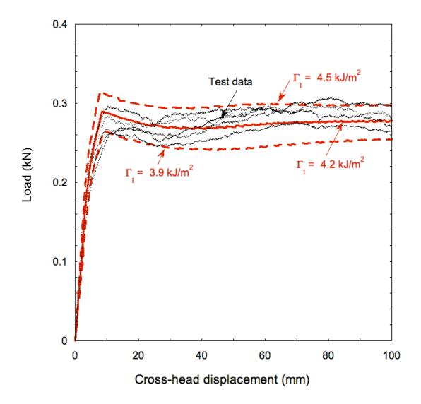
Figure 5 Fit between the DCB experimental load-displacement data and the numerical predictions of a cohesive-zone model, showing upper and lower bounds for the fit. The toughness for the adhesive was determined to be  $4.2 \pm 0.3 \text{ kJm}^{-2}$ .
