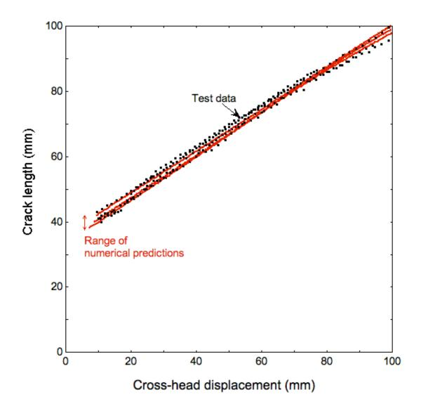
Figure 6 Fit between the experimental crack length *versus* cross-head displacement data and the numerical predictions for quasi-static crack growth in the DCB geometry. The numerical predictions are based on a cohesive model with a mode-I toughness of  $4.2 \pm 0.3$  kJm<sup>-2</sup> and a cohesive strength of  $24 \pm 3$  MPa.
