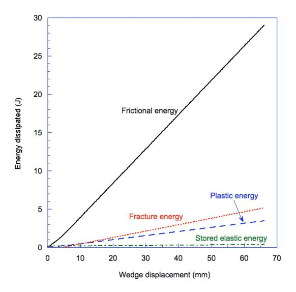
Figure 11 The results of a numerical calculation for a quasi-static wedge test with a coefficient of friction equal to 0.32. The plots show how the elastic energy stored in the geometry, the plastic energy dissipated, the fracture energy dissipated and the frictional energy dissipated vary with wedge displacement.
