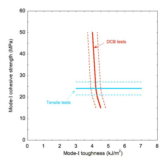
Figure 3 A plot showing the ranges of values for the mode-I toughness and normal cohesive strength values that give an acceptable agreement between the numerical and experimental results for the DCB geometry and tensile test geometry.
