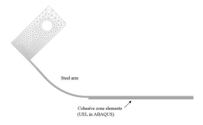
Figure 2 Configuration of the DCB geometry used for the numerical simulations.
