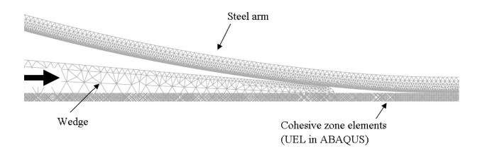
Figure 10 A static ABAQUS/Standard 2D model was used to simulate the wedge tests. Owing to the symmetry of geometry, only half of the specimen was simulated. The calculation was performed by forcing the wedge along the interface between the steel coupons. Contact elements were placed along the surfaces of the wedge and adherends. This figure shows the curvature of the steel arm after fracture.
