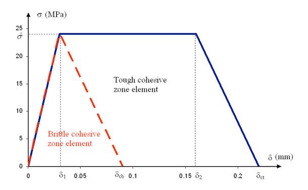
Figure 7 A comparison between the two traction-separation laws used for quasistatic and for dynamic fracture. The cohesive strength,  $\hat{\sigma}$ , was fixed at  $24 \pm 3$  MPa for both laws. The toughness for the "tough" (quasi-static) elements was fixed at  $4.2 \pm 0.3$  kJm<sup>-2</sup> The toughness for the "brittle" (dynamic) elements was found to be equal to  $1.05 \pm 0.05$  kJm<sup>-2</sup>.
