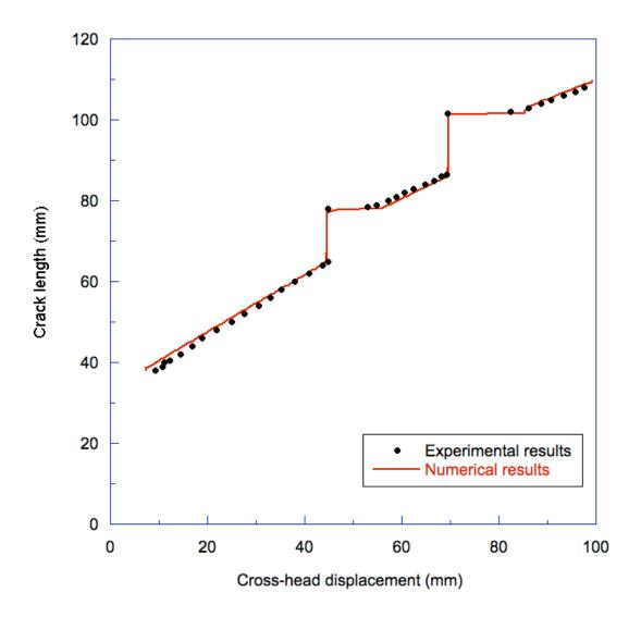
Figure 9 Comparison between the experimental data for the variation in crack length with cross-head displacement and the numerical predictions from a cohesive-zone model for the DCB geometry in which dynamic fracture occurred at an applied displacement rate of 150 mm/s.
