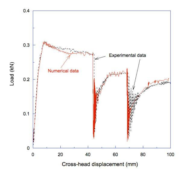
Figure 8 Fit between the experimental load-displacement data for the DCB specimens at a loading rate of 150 mm/s in which dynamic fracture occurred, and the numerical predictions of the two-part cohesive-zone model.
