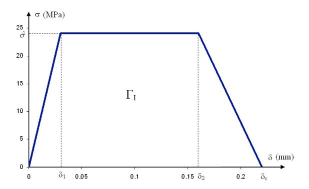
Figure 1 An example of the trapezoidal mode-I traction-separation law used for quasi-static fracture of the adhesive layer.
