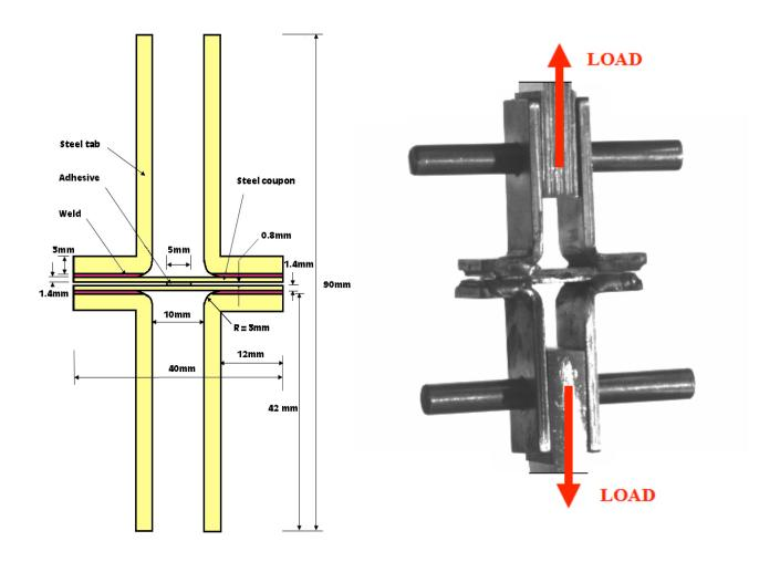
Figure 4 Configuration of the tensile test specimen used to evaluate the cohesive strength of the adhesive system. Two steel coupons are bonded in the middle by the adhesive. These coupons are bonded to thick steel tabs that transmit the load.
