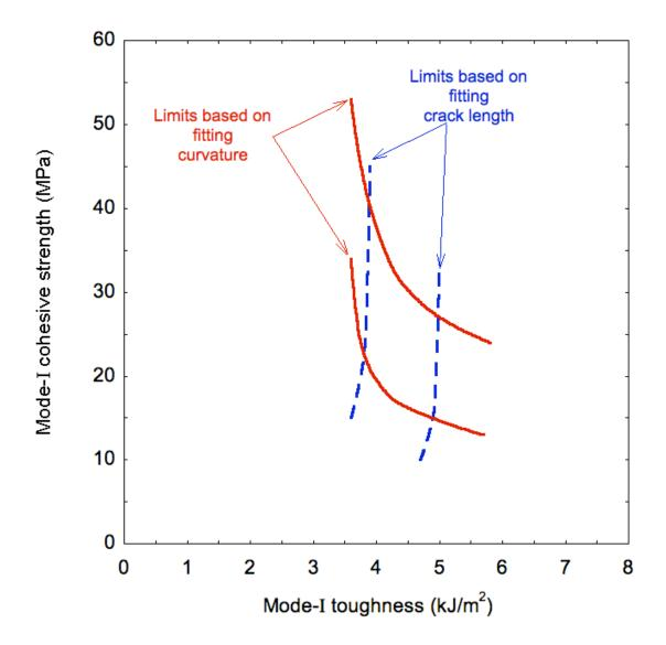
Figure 13 A plot showing the ranges of values for the mode-I toughness and cohesive strength values that give an acceptable agreement between the results of numerical calculations, and the two experimental measurements that could be obtained from the wedge test.
