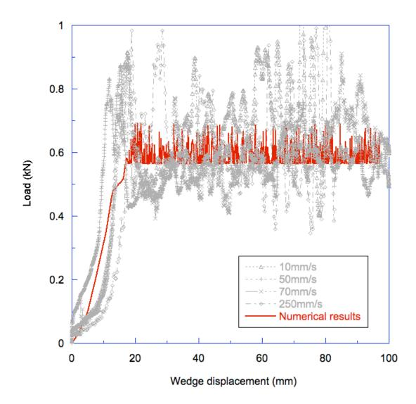
Figure 12 A comparison between the reaction load on the wedge computed for the quasi-static tests with a coefficient of friction equal to 0.32, and loads measured during quasi-static tests.
