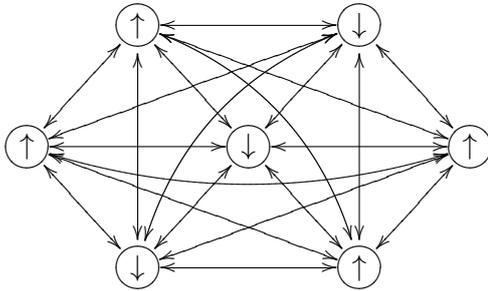
**Figure 8.1:** Illustration of an exemplary Hopfield network. The arrows  $\uparrow$  and  $\downarrow$  mark the binary "spin". Due to the completely linked neurons the layers cannot be separated, which means that a Hopfield network simply includes a set of neurons.
