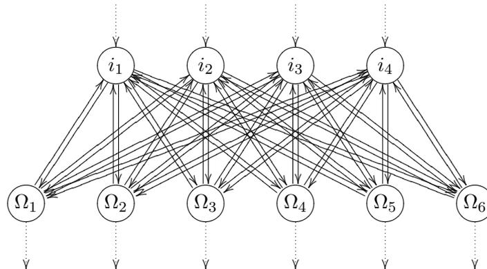
**Figure 11.1:** Simplified illustration of the ART network structure. Top: the input layer, bottom: the recognition layer. In this illustration the lateral inhibition of the recognition layer and the control neurons are omitted.
