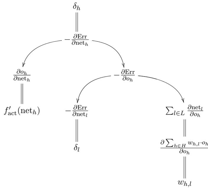
**Figure 5.12:** Graphical representation of the equations (by equal signs) and chain rule splittings (by arrows) in the framework of the backpropagation derivation. The leaves of the tree reflect the final results from the generalization of  $\delta$ , which are framed in the derivation.
