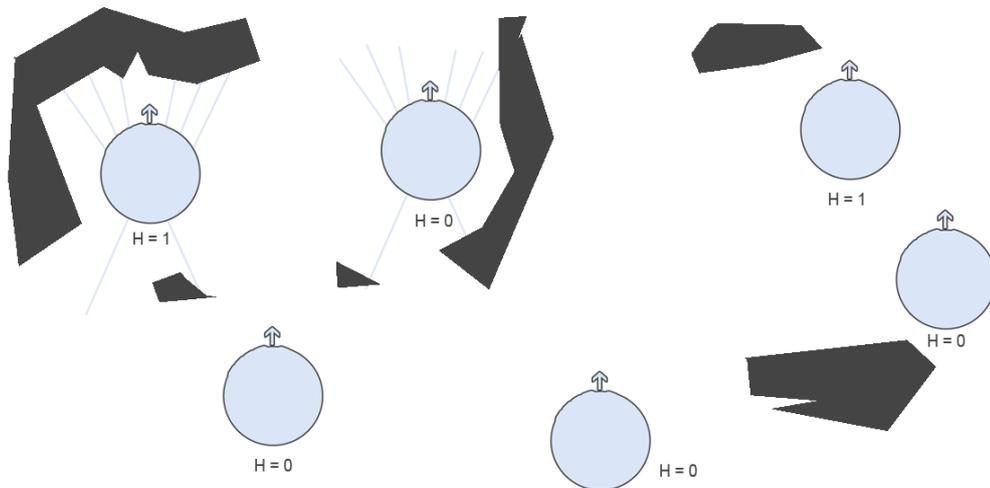
**Figure 1.2:** The robot is positioned in a landscape that provides sensor values for different situations. We add the desired output values  $H$  and so receive our learning samples. The directions in which the sensors are oriented are exemplarily applied to two robots.
