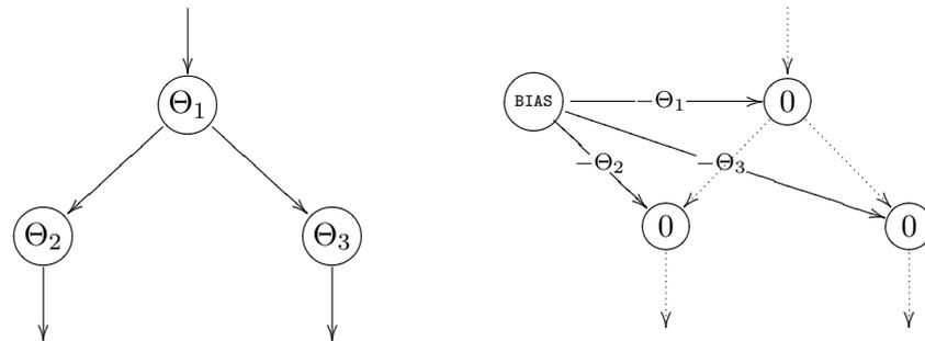
**Figure 3.9:** Two equivalent neural networks, one without bias neuron on the left, one with bias neuron on the right. The neuron threshold values can be found in the neurons, the connecting weights at the connections. Furthermore, I omitted the weights of the already existing connections (represented by dotted lines on the right side).
