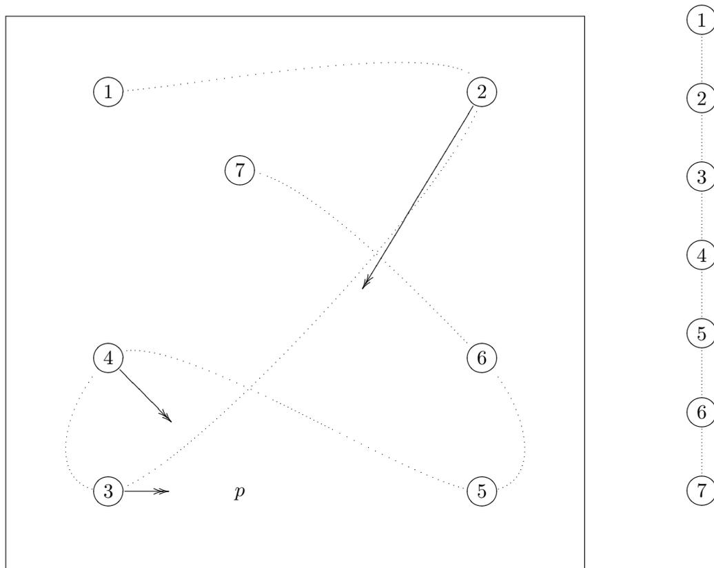
**Figure 10.4:** Illustration of the two-dimensional input space (left) and the one-dimensional topology space (right) of a self-organizing map. Neuron 3 is the winner neuron since it is closest to  $p$ . In the topology, the neurons 2 and 4 are the neighbors of 3. The arrows mark the movement of the winner neuron and its neighbors towards the training sample  $p$ .
