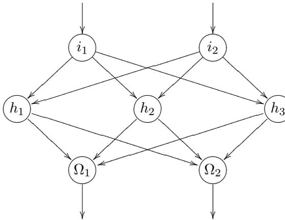
**Definition 3.10** (Feedforward network with shortcut connections). Similar to the feedforward network, but the connections may not only be directed towards the next layer but also towards any other subsequent layer.
