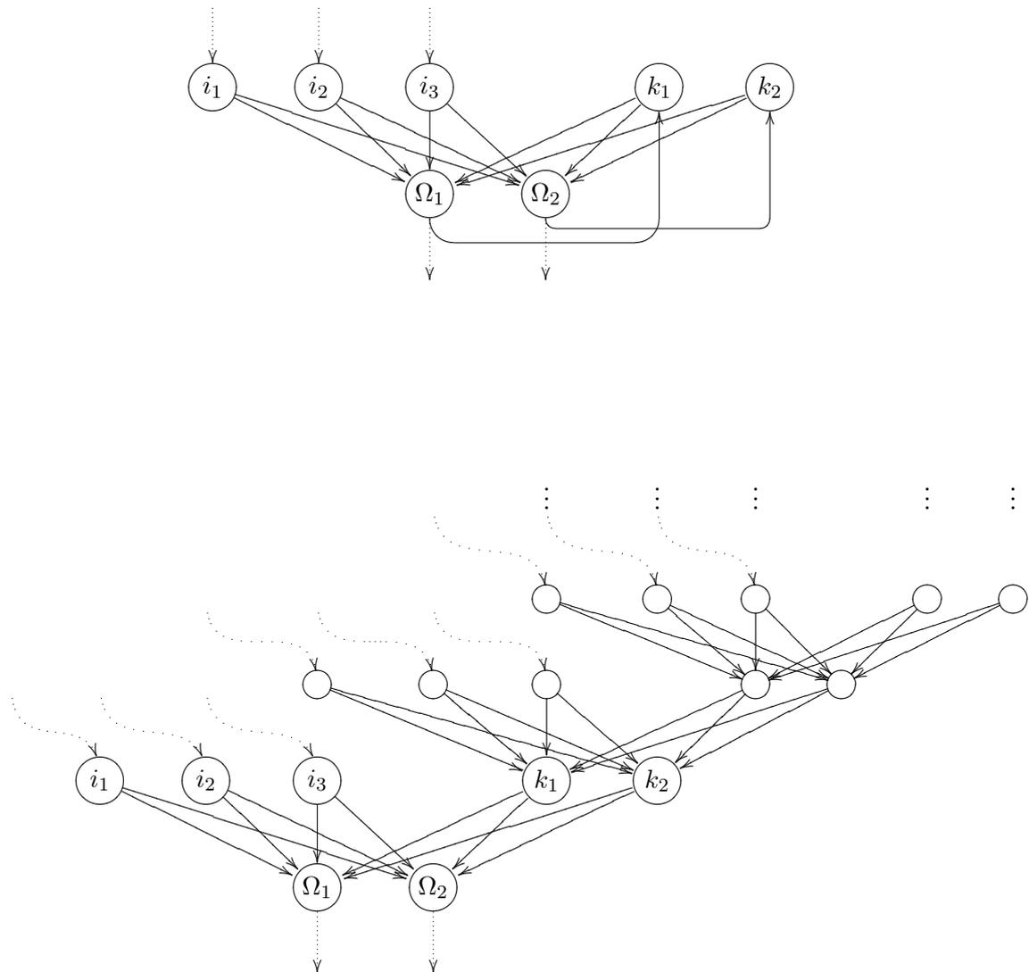
**Figure 7.4:** Illustration of the unfolding in time with a small exemplary recurrent MLP. **Top:** The recurrent MLP. **Bottom:** The unfolded network. For reasons of clarity, I only added names to the lowest part of the unfolded network. Dotted arrows leading into the network mark the inputs. Dotted arrows leading out of the network mark the outputs. Each "network copy" represents a time step of the network with the most recent time step being at the bottom.
