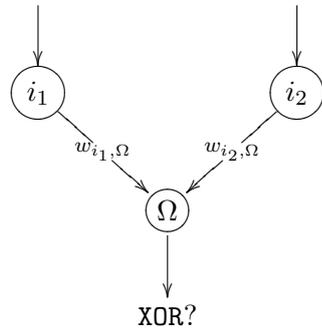
**Figure 5.6:** Sketch of a singlelayer perceptron that shall represent the XOR function - which is impossible.
