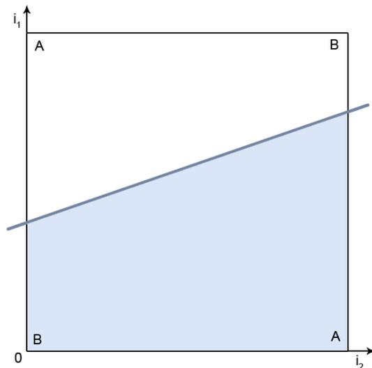
**Figure 5.7:** Linear separation of  $n = 2$  inputs of the input neurons  $i_1$  and  $i_2$  by a 1-dimensional straight line. A and B show the corners belonging to the sets of the XOR function that are to be separated.
