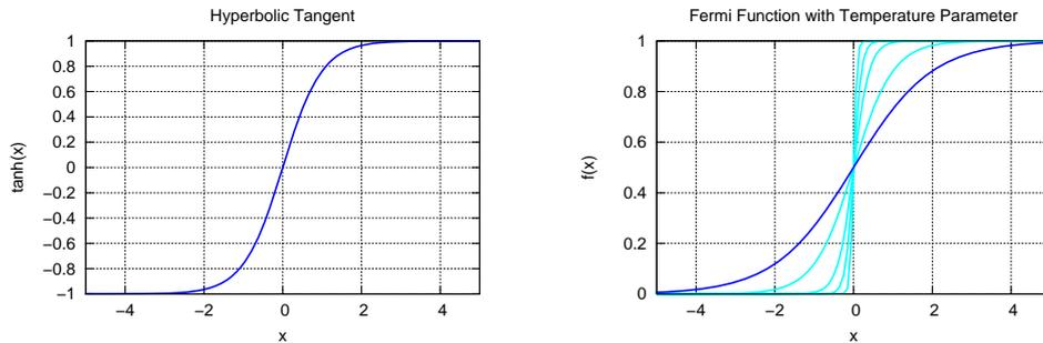
**Figure 5.14:** As a reminder the illustration of the hyperbolic tangent (left) and the Fermi function (right). The Fermi function was expanded by a temperature parameter. The original Fermi function is thereby represented by dark colors, the temperature parameter of the modified Fermi functions are, ordered ascending by steepness,  $\frac{1}{2}$ ,  $\frac{1}{5}$ ,  $\frac{1}{10}$  and  $\frac{1}{25}$ .
