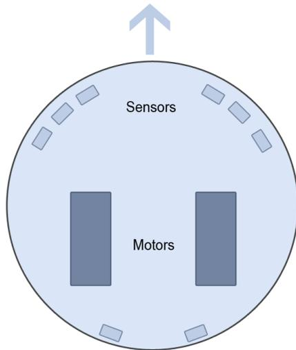
**Figure 1.1:** A small robot with eight sensors and two motors. The arrow indicates the driving direction.
