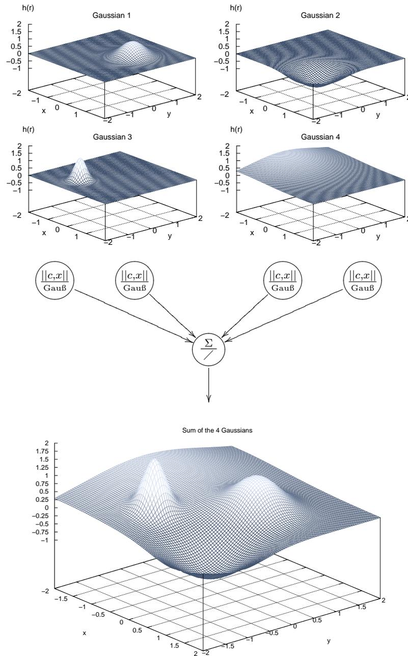
**Figure 6.5:** Four different Gaussian bells in two-dimensional space generated by means of RBF neurons are added by an output neuron of the RBF network. Once again  $r = \sqrt{x^2 + y^2}$  applies for the distance. The heights  $w$ , widths  $\sigma$  and centers  $c = (x, y)$  are:  $w_1 = 1, \sigma_1 = 0.4, c_1 = (0.5, 0.5)$ ,  $w_2 = -1, \sigma_2 = 0.6, c_2 = (1.15, -1.15)$ ,  $w_3 = 1.5, \sigma_3 = 0.2, c_3 = (-0.5, -1)$ ,  $w_4 = 0.8, \sigma_4 = 1.4, c_4 = (-2, 0)$ .
