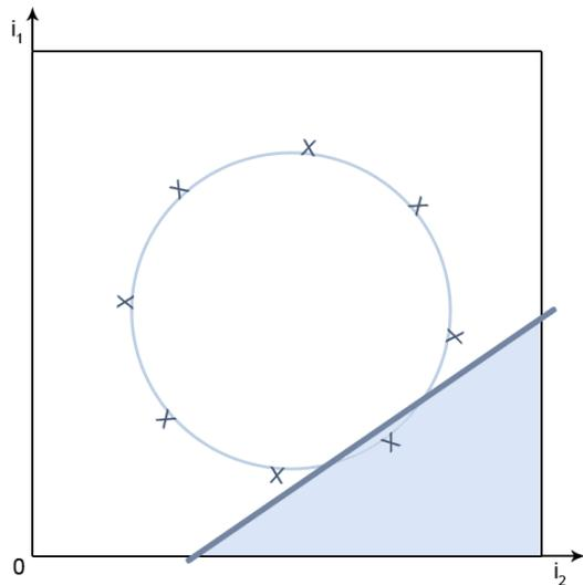
**Figure 5.15:** Illustration of the functionality of 8-2-8 network encoding. The marked points represent the vectors of the inner neuron activation associated to the samples. As you can see, it is possible to find inner activation formations so that each point can be separated from the rest of the points by a straight line. The illustration shows an exemplary separation of one point.
