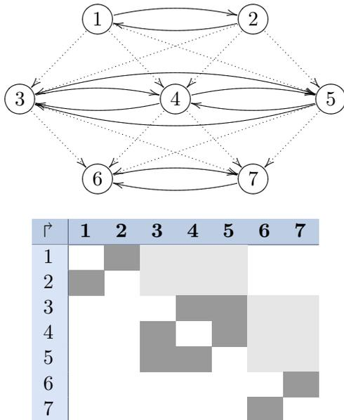
**Figure 3.7:** A network similar to a feedforward network with laterally recurrent neurons. The direct recurrences are represented by solid lines. Here, recurrences only exist within the layer. In the Hinton diagram, filled squares are concentrated around the diagonal in the height of the feedforward blocks, but the diagonal is left uncovered.
