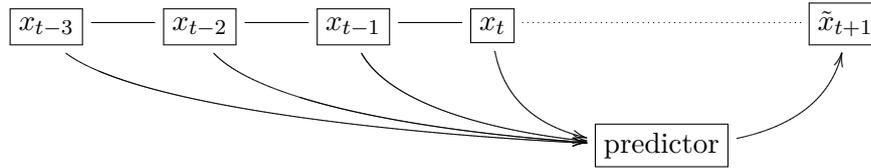
**Figure B.2:** Representation of the one-step-ahead prediction. It is tried to calculate the future value from a series of past values. The predicting element (in this case a neural network) is referred to as predictor.
