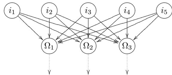
Certainly, the existence of several output neurons  $\Omega_1, \Omega_2, \dots, \Omega_n$  does not considerably change the concept of the perceptron (fig. 5.3): A perceptron with several output neurons can also be regarded as several different perceptrons with the same input.
