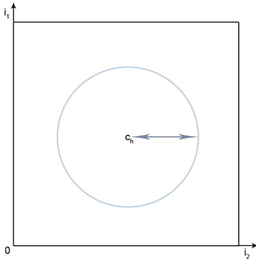
**Figure 6.2:** Let  $c_h$  be the center of an RBF neuron  $h$ . Then the activation function  $f_{act_h}$  is radially symmetric around  $c_h$ .
