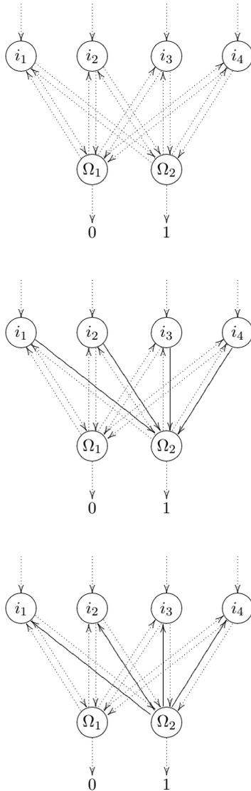
**Figure 11.2:** Simplified illustration of the two-piece training of an ART network: The trained weights are represented by solid lines. Let us assume that a pattern has been entered into the network and that the numbers mark the outputs. **Top:** We can see that  $\Omega_2$  is the winner neuron. **Middle:** So the weights are trained towards the winner neuron and (**below**) the weights of the winner neuron are trained towards the input layer.
