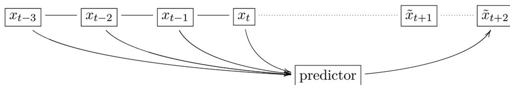
**Figure B.4:** Representation of the direct two-step-ahead prediction. Here, the second time step is predicted directly, the first one is omitted. Technically, it does not differ from a one-step-ahead prediction.
