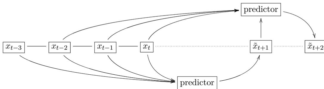
**Figure B.3:** Representation of the two-step-ahead prediction. Attempt to predict the second future value out of a past value series by means of a second predictor and the involvement of an already predicted value.
