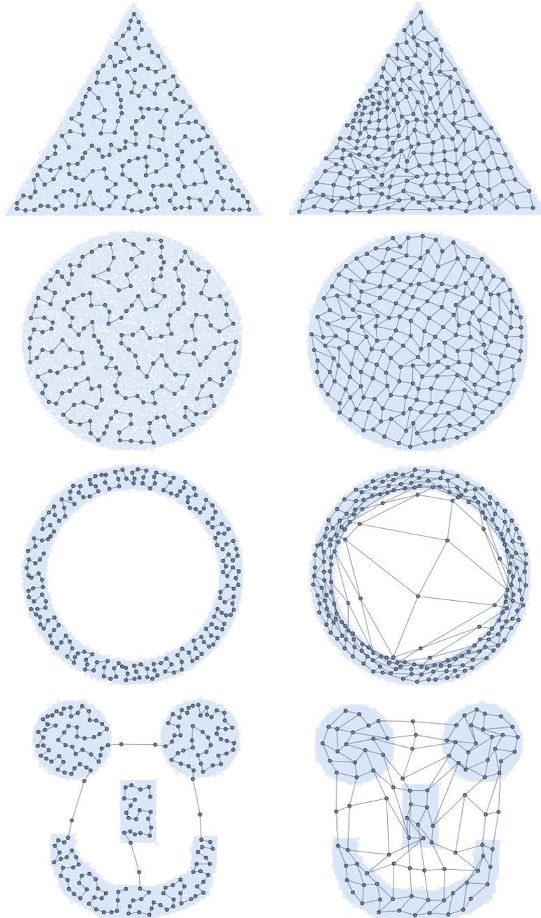
**Figure 10.6:** End states of one-dimensional (left column) and two-dimensional (right column) SOMs on different input spaces. 200 neurons were used for the one-dimensional topology,  $10 \times 10$  neurons for the two-dimensional topology and 80.000 input patterns for all maps.
