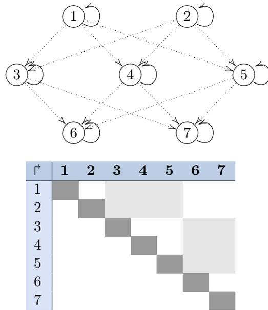
**Figure 3.5:** A network similar to a feedforward network with directly recurrent neurons. The direct recurrences are represented by solid lines and exactly correspond to the diagonal in the Hinton diagram matrix.
