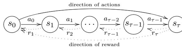
**Figure C.9:** Actions are performed until the desired target situation is achieved. Attention should be paid to numbering: Rewards are numbered beginning with 1, actions and situations beginning with 0 (This has simply been adopted as a convention).
