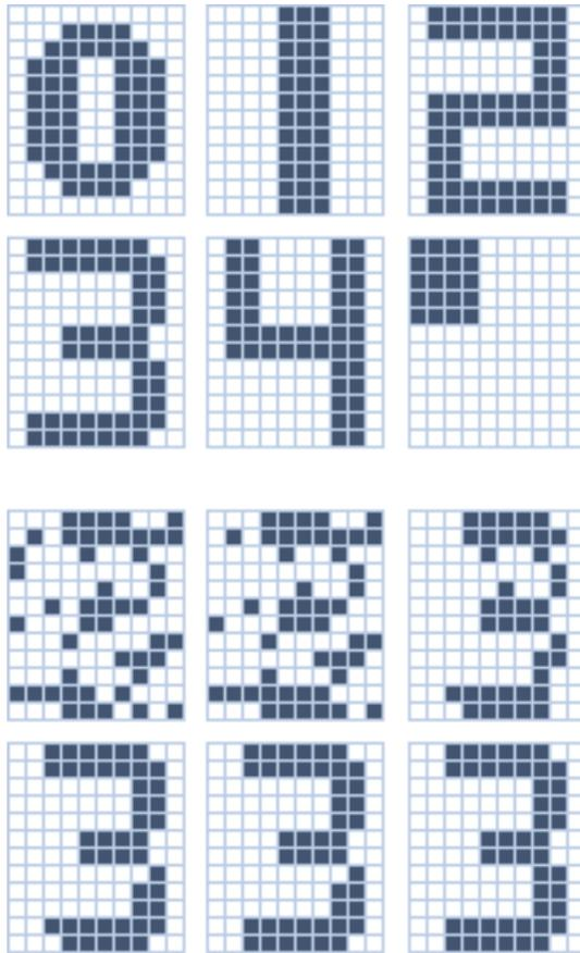
**Figure 8.3:** Illustration of the convergence of an exemplary Hopfield network. Each of the pictures has  $10 \times 12 = 120$  binary pixels. In the Hopfield network each pixel corresponds to one neuron. The upper illustration shows the training samples, the lower shows the convergence of a heavily noisy 3 to the corresponding training sample.
