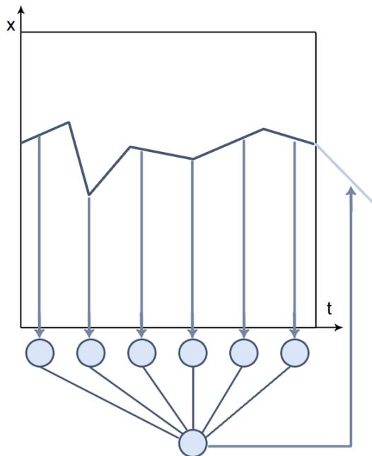
**Figure B.1:** A function  $x$  that depends on the time is sampled at discrete time steps (time discretized), this means that the result is a time series. The sampled values are entered into a neural network (in this example an SLP) which shall learn to predict the future values of the time series.
