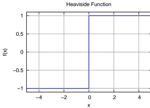
**Figure 8.2:** Illustration of the binary threshold function.
