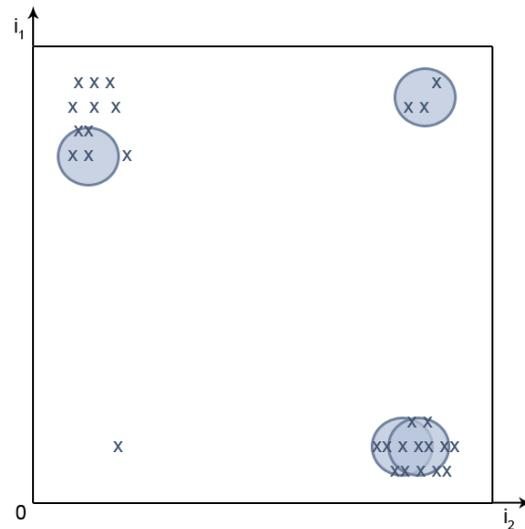
**Figure 6.8:** Example of an uneven coverage of a two-dimensional input space by applying radial basis functions. The widths were fixedly selected, the centers of the neurons were randomly distributed throughout the training patterns. This distribution can certainly lead to slightly unrepresentative results, which can be seen at the single data point down to the left.
