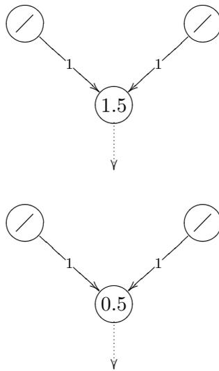
**Figure 5.4:** Two singlelayer perceptrons for Boolean functions. The upper singlelayer perceptron realizes an AND, the lower one realizes an OR. The activation function of the information processing neuron is the binary threshold function. Where available, the threshold values are written into the neurons.
