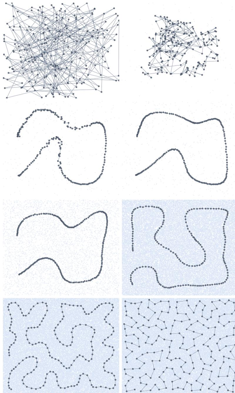
**Figure 10.5:** Behavior of a SOM with one-dimensional topology ( $G = 1$ ) after the input of 0, 100, 300, 500, 5000, 50000, 70000 and 80000 randomly distributed input patterns  $p \in \mathbb{R}^2$ . During the training  $\eta$  decreased from 1.0 to 0.1, the  $\sigma$  parameter of the Gauss function decreased from 10.0 to 0.2.
