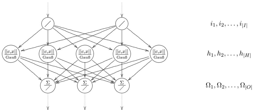
**Figure 6.1:** An exemplary RBF network with two input neurons, five hidden neurons and three output neurons. The connections to the hidden neurons are not weighted, they only transmit the input. Right of the illustration you can find the names of the neurons, which coincide with the names of the MLP neurons: Input neurons are called  $i$ , hidden neurons are called  $h$  and output neurons are called  $\Omega$ . The associated sets are referred to as  $I$ ,  $H$  and  $O$ .
