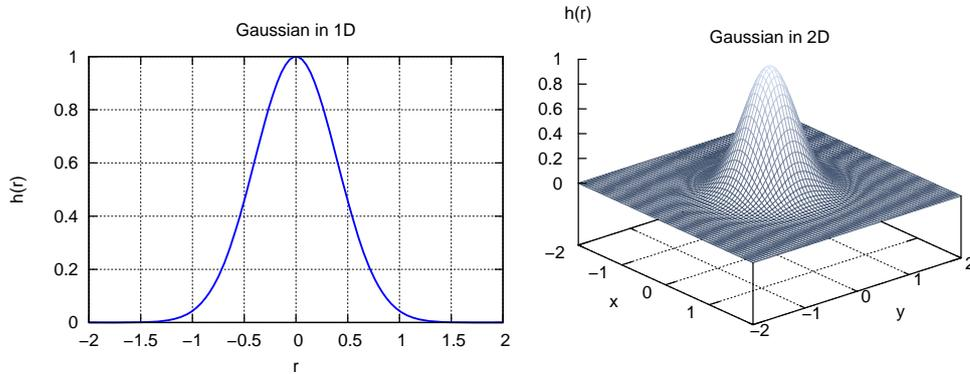
**Figure 6.3:** Two individual one- or two-dimensional Gaussian bells. In both cases  $\sigma = 0.4$  holds and the centers of the Gaussian bells lie in the coordinate origin. The distance  $r$  to the center  $(0, 0)$  is simply calculated according to the Pythagorean theorem:  $r = \sqrt{x^2 + y^2}$ .
