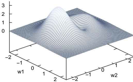
**Figure 5.5:** Exemplary error surface of a neural network with two trainable connections  $w_1$  and  $w_2$ . Generally, neural networks have more than two connections, but this would have made the illustration too complex. And most of the time the error surface is too craggy, which complicates the search for the minimum.
