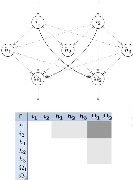
**Figure 3.4:** A feedforward network with short-cut connections, which are represented by solid lines. On the right side of the feedforward blocks new connections have been added to the Hinton diagram.
