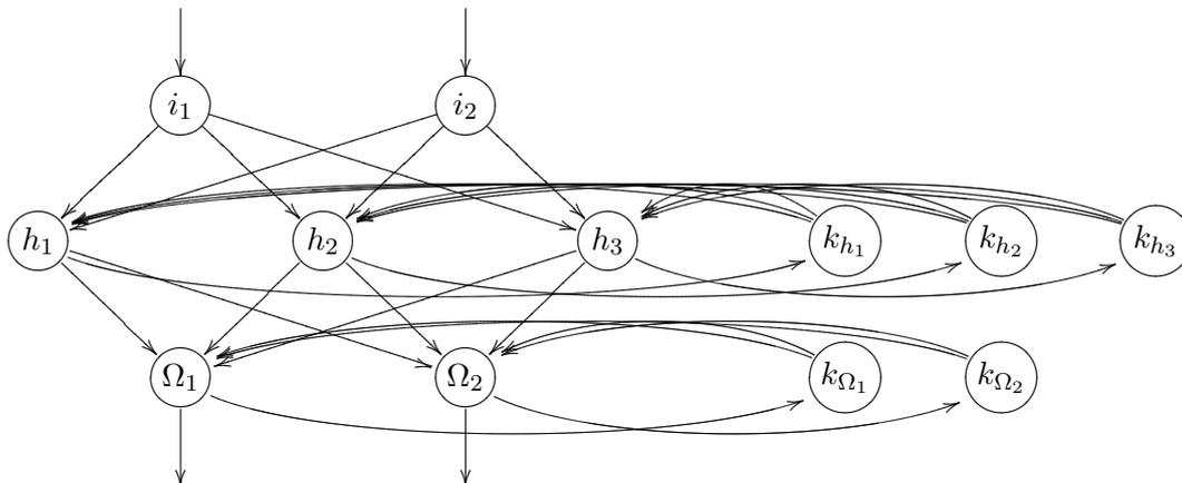
**Figure 7.3:** Illustration of an Elman network. The entire information processing part of the network exists, in a way, twice. The output of each neuron (except for the output of the input neurons) is buffered and reentered into the associated layer. For the reason of clarity I named the context neurons on the basis of their models in the actual network, but it is not mandatory to do so.
