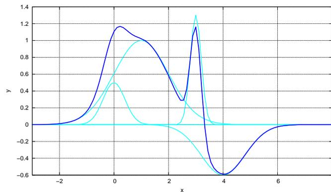
**Figure 6.4:** Four different Gaussian bells in one-dimensional space generated by means of RBF neurons are added by an output neuron of the RBF network. The Gaussian bells have different heights, widths and positions. Their centers  $c_1, c_2, \dots, c_4$  are located at 0, 1, 3, 4, the widths  $\sigma_1, \sigma_2, \dots, \sigma_4$  at 0.4, 1, 0.2, 0.8. You can see a two-dimensional example in fig. 6.5 on the following page.
