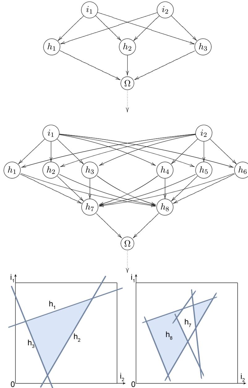
**Figure 5.10:** We know that an SLP represents a straight line. With 2 trainable weight layers, several straight lines can be combined to form convex polygons (above). By using 3 trainable weight layers several polygons can be formed into arbitrary sets (below).
