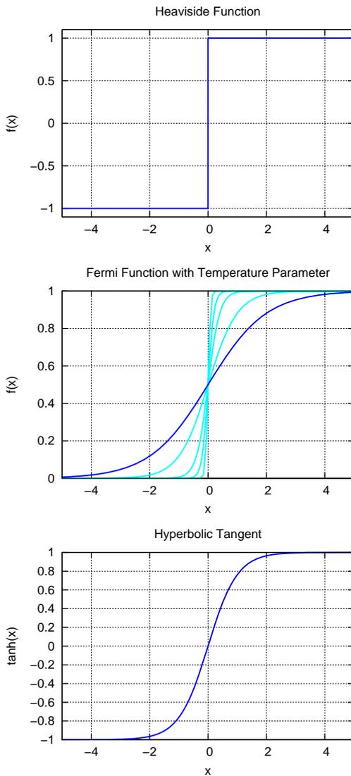
**Figure 3.2:** Various popular activation functions, from top to bottom: Heaviside or binary threshold function, Fermi function, hyperbolic tangent. The Fermi function was expanded by a temperature parameter. The original Fermi function is represented by dark colors, the temperature parameters of the modified Fermi functions are, ordered ascending by steepness,  $\frac{1}{2}$ ,  $\frac{1}{5}$ ,  $\frac{1}{10}$  und  $\frac{1}{25}$ .
