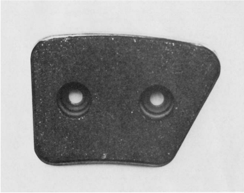
FIGURE 6 Typical caliper brake pad of sintered material for heavy aircraft brakes. (Note contour of the pad to place lining material toward the outer periphery of the disk.) (Courtesy Friction Products, Medina, OH.)
