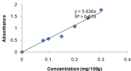
Figure 4. Standard Curve of Saponin Concentrations
