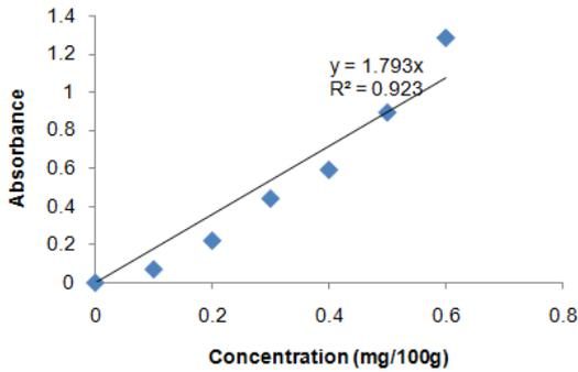
Figure 3. Standard Curve of Steroid Concentrations
