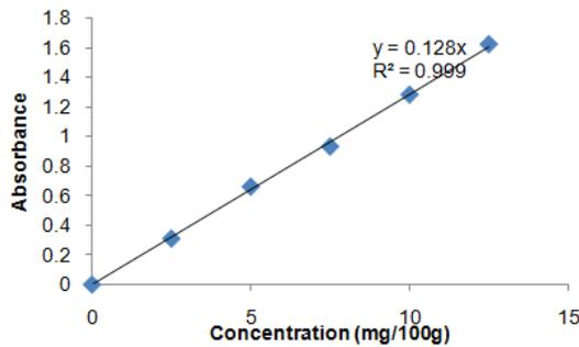
Figure 6. Standard Curve of Phytate Concentrations
