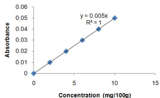
Figure 2. Standard Curve of Glycosidic Cyanide Concentration
