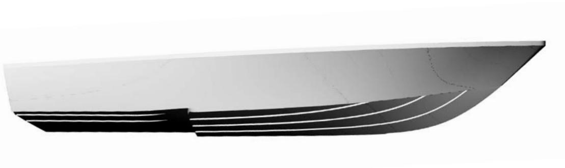
*Fig. 1.4 Delta 29 SW with a Transverse Step*
