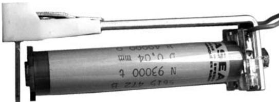
FIGURE 2.36 Elongated coil of a highly sensitive clapper armature relay with winding, containing 93,000 turns of wire with a diameter of 0.04 mm (resistance of 40 k \Omega ).
