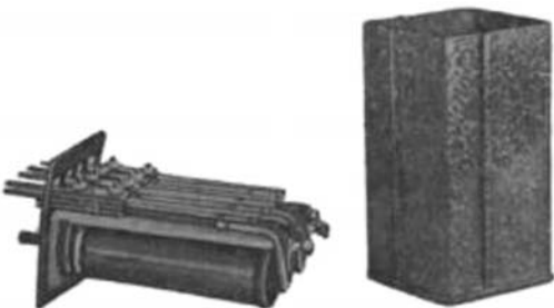
FIGURE 1.21 Eriksson relay, produced by the “Krasnaya Zarya” plant until 1925.
