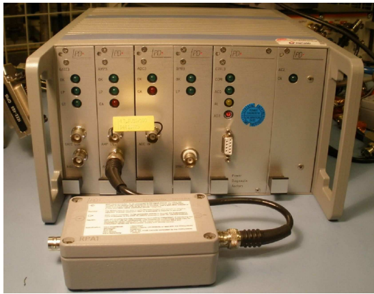
FIGURE 10.1: The ICM PD-pulse measurement instrument: the main unit is in the background, with its input connected to a preamplifier in the foreground.
