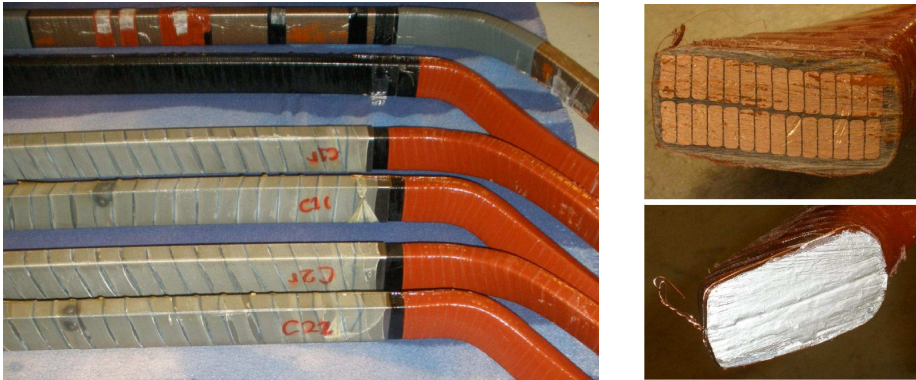
FIGURE 18.1: Left: all six stator-bars, showing half the slot-section and part of the end; in the background are the two bars without metal plates, for material measurements. Right: end-view showing strands before (top) and after (bottom) connecting with conductive paint.
