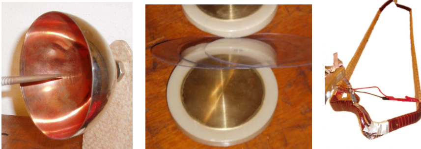
FIGURE 17.1: PD test-objects. Left to right: point-hemisphere, cavity (shown with the electrodes and insulating disks separated), stator coil
