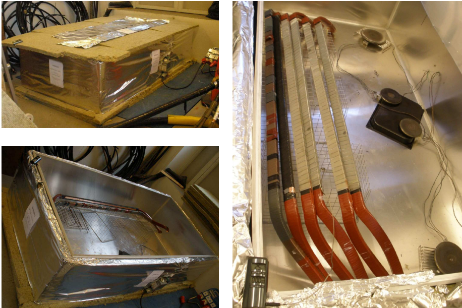
FIGURE 18.3: The large laboratory-oven for thermal aging. On the left, with and without the lid and its insulation. On the right, four normal bars and two material-sample bars are in place, and heater elements are visible at the right.
