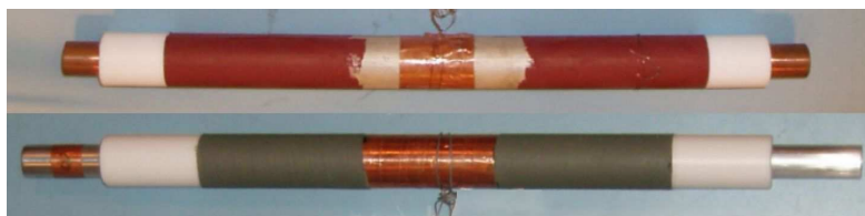
FIGURE 19.3: PTFE tubes with gradings using paint (top) and tape (bottom).
