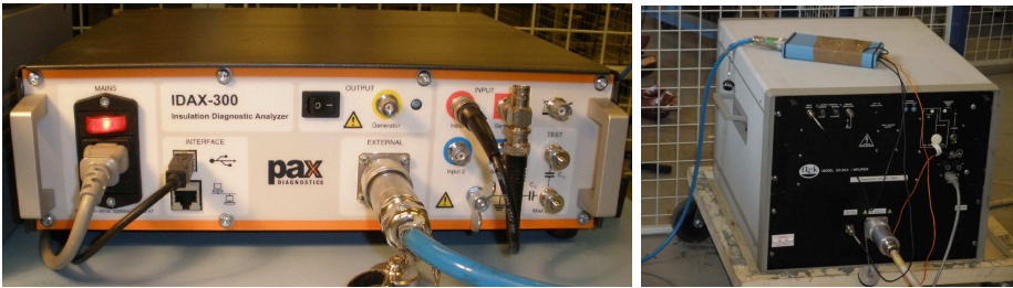
FIGURE 9.1: The IDAX 300 DS-instrument (left) and its HVU (right).
