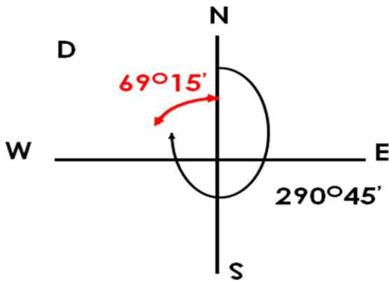
**Solution :** Line PD lies in 4th quadrant. Quadrant Bearing bearing of PD = N 69° 15' W
