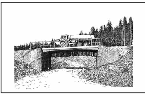
**T beam and slab bridge:**
