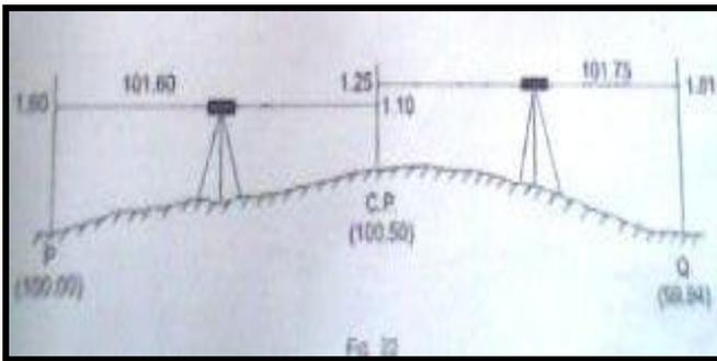
The elevation of change point = Elevation of P + Back sight at P – Fore sight at change point (C.P)
