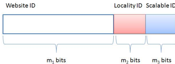
Figure 4.1: Peer ID structure in D-ring of PetalUp-CDN.
