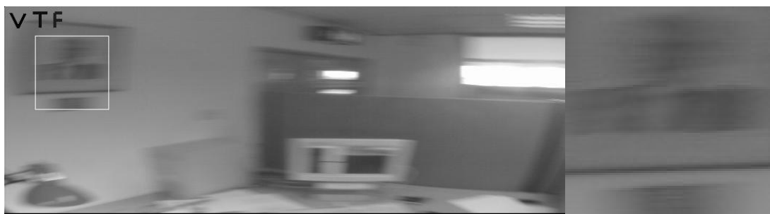
Figure 4.1: Substantial motion blur due to 2.6 rad/s camera rotation, with 100x100 pixel enlargement
