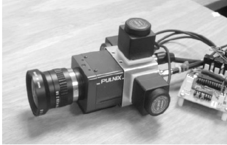
Figure 4.5: Rate gyroscopes affixed to camera
