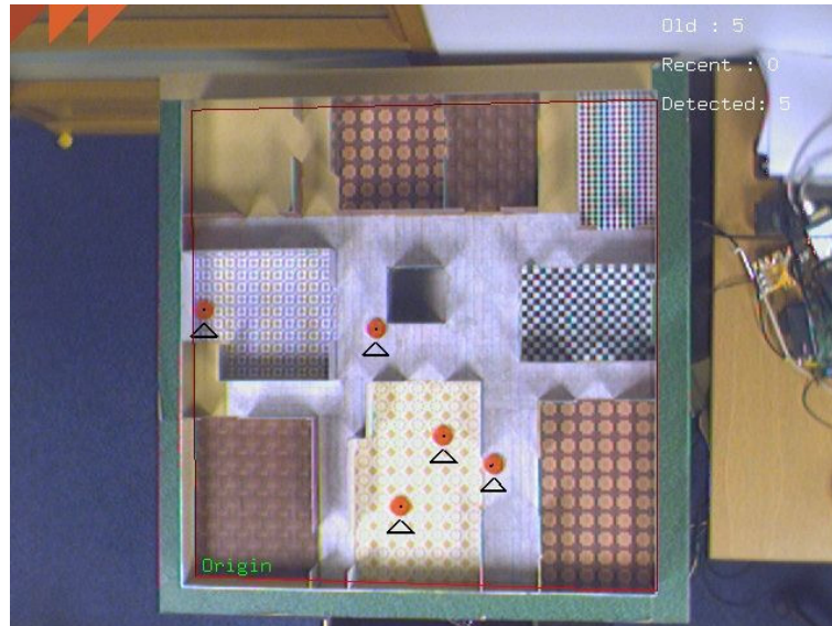
Figure 6.9: Token detection. Tokens are recognisable by their colour and shape in the feed (shown here) from an overhead camera. Colour templates, shown in the top left, can be selected in the image to calibrate the system.
