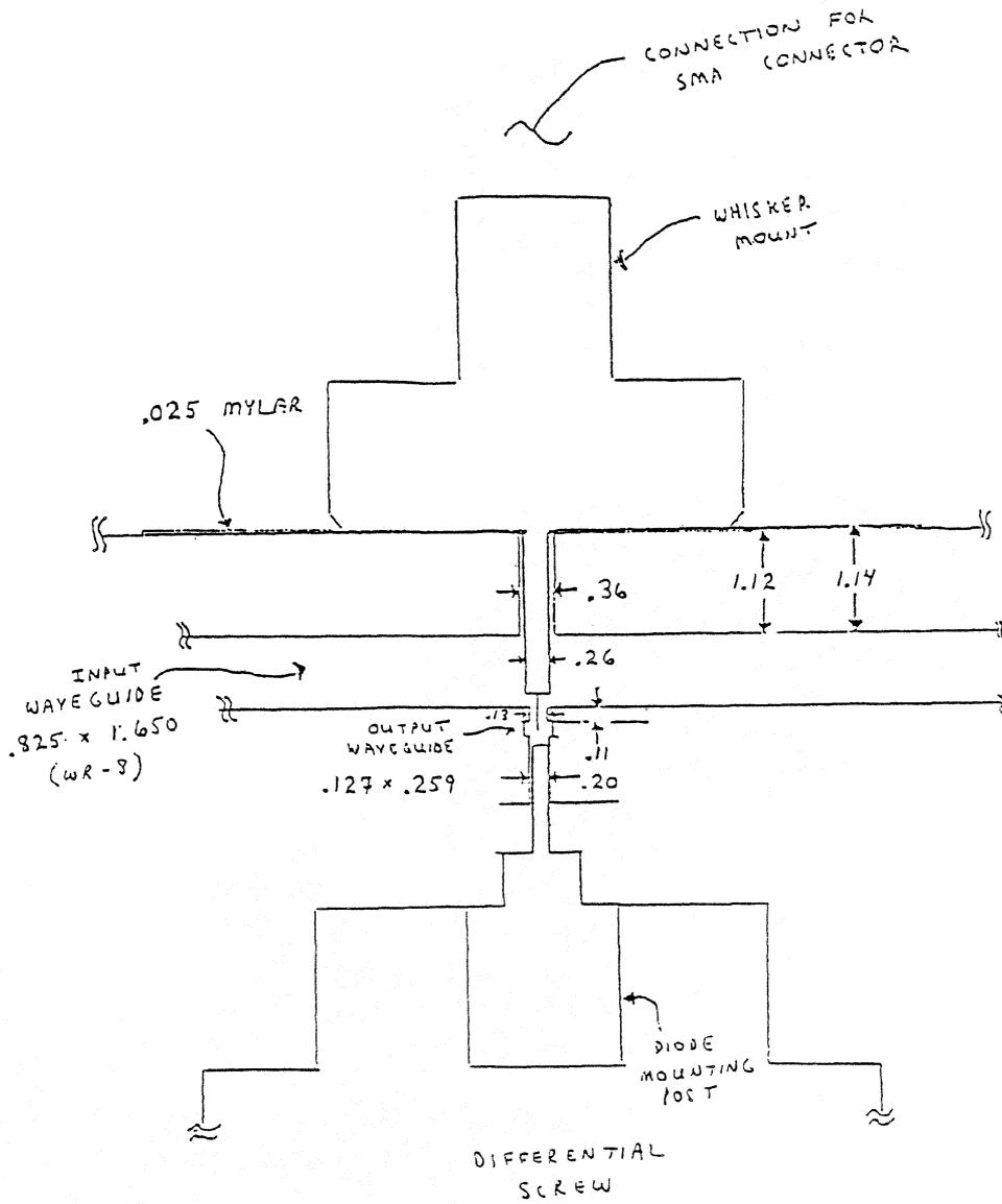
Figure 1: Layout and dimensions of the quintupler for 600-720 GHz. The dimensions are in millimeters.
