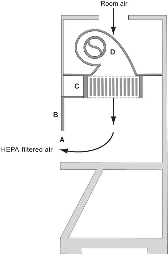
**Figure 10.** A modified containment cabinet or Class I BSC can be used for labeling infectious microorganisms with  $I^{125}$ . (A) arm holes; (B) Lexan<sup>®</sup> hinged doors; (C) exhaust charcoal filter; (D) exhaust HEPA filter; (E) filter housing with required connection to building exhaust (see also Figure 13).
