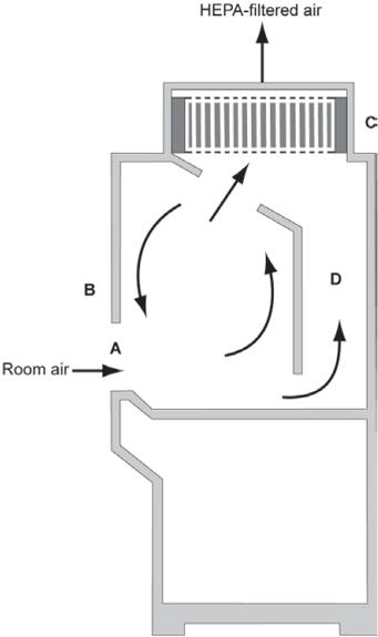
**Figure 3. The Class II, Type A1 BSC** (A) front opening; (B) sash; (C) exhaust HEPA filter; (D) supply HEPA filter; (E) common plenum; (F) blower.
