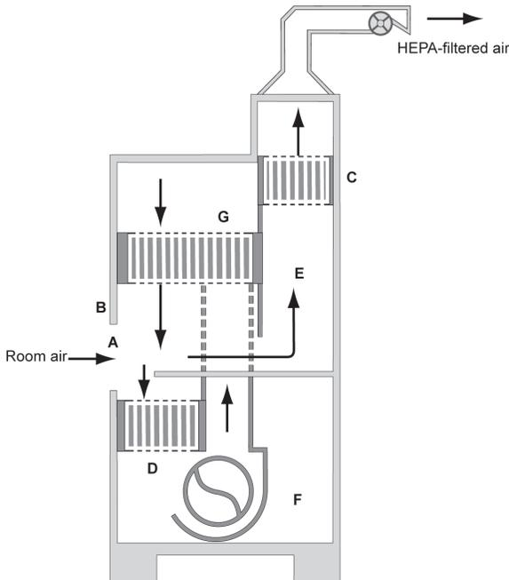
**Figure 5B. The Class II, Type B1 BSC (bench top design)** (A) front opening; (B) sash; (C) exhaust HEPA filter; (D) supply plenum; (E) supply HEPA filter; (F) blower; (G) negative pressure exhaust plenum. *Note:* The cabinet exhaust needs to be hard connected to the building exhaust system.
