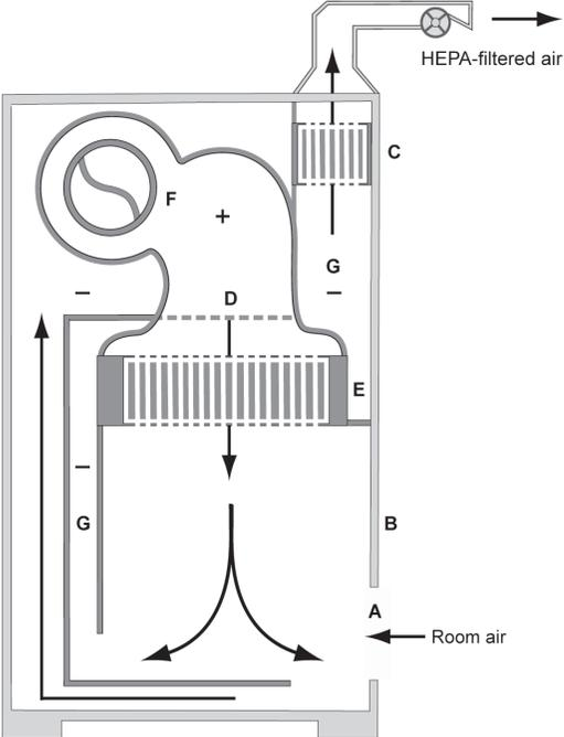
**Figure 6. The Class II, Type B2 BSC** (A) front opening; (B) sash; (C) exhaust HEPA filter; (D) supply HEPA filter; (E) negative pressure exhaust plenum. *Note:* The carbon filter in the exhaust system is not shown. The cabinet needs to be hard connected to the building exhaust system.
