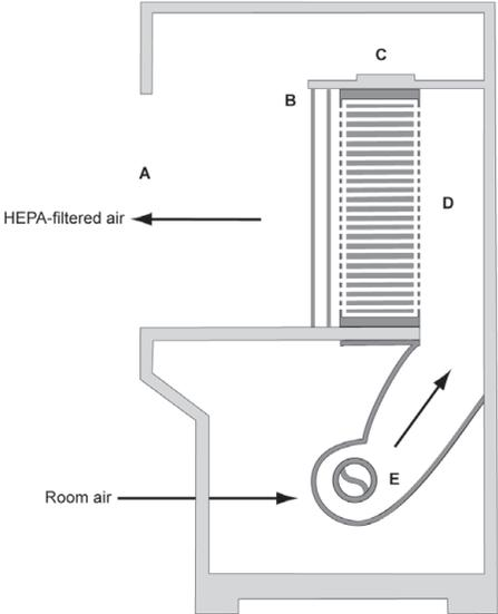
**Figure 9B. The vertical laminar flow “clean bench”** (A) front opening; (B) sash; (C) supply HEPA filter; (D) blower. *Note:* Some vertical flow clean benches have recirculated air through front and/or rear perforated grilles.
