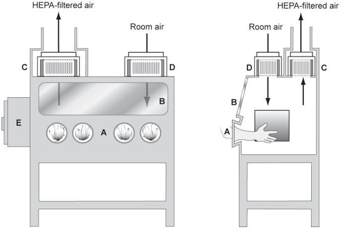
**Figure 9A. The horizontal laminar flow “clean bench”** (A) front opening; (B) supply grille; (C) supply HEPA filter; (D) supply plenum; (E) blower.
