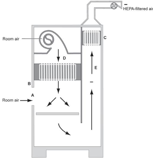
**Figure 7. The tabletop model of a Class II, Type A2 BSC** (A) front opening; (B) sash; (C) exhaust HEPA filter; (D) supply HEPA filter; (E) positive pressure common plenum; (F) negative pressure plenum. The Class II Type A2 BSC is not equivalent to what was formerly called a Class II Type B3 unless it is connected to the laboratory exhaust system. *Note:* The A2 BSC should be canopy connected to the exhaust system.
