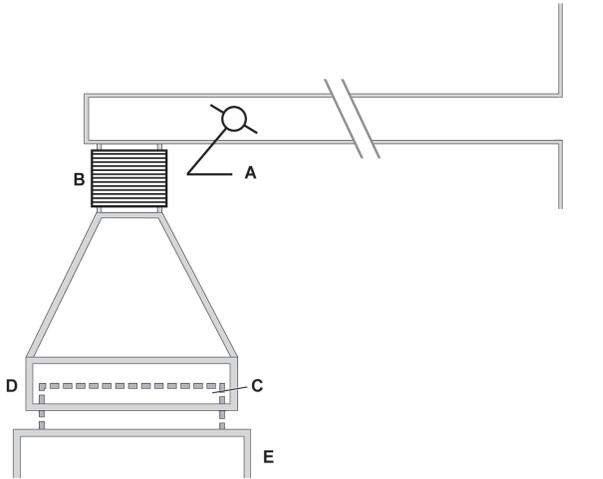
**Figure 5A. The Class II, Type B1 BSC (classic design)** (A) front opening; (B) sash; (C) exhaust HEPA filter; (D) supply HEPA filter; (E) negative pressure dedicated exhaust plenum; (F) blower; (G) additional HEPA filter for supply air. *Note:* The cabinet exhaust needs to be hard connected to the building exhaust system.
