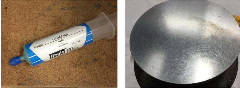
Figure 8.  $1\mu\text{m}$  diamond compound (a, left), scratches from diamond pads significantly affected surface quality (b, right)
