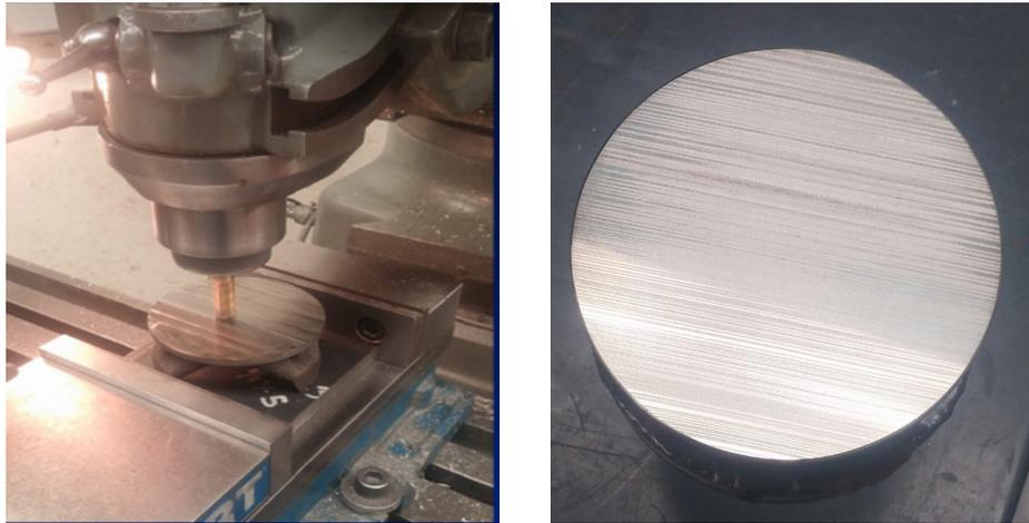
Figure 2: Titanium mirror milled flat to reduce time spent on grinding (a, left), final machined titanium mirror (b, right)
