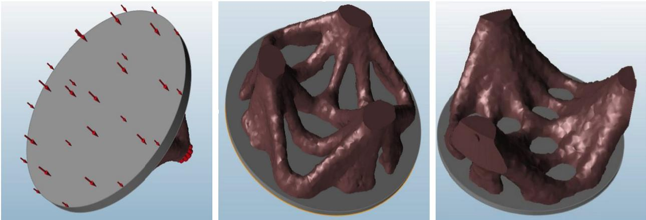
Figure 1. Applied loads and forces (a, left) in Altair Hyperworks to model top mount (b, center) and side mount (c, right)
