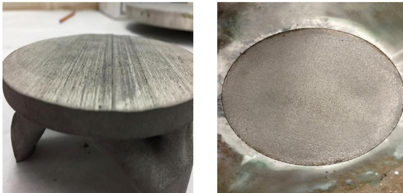
Figure 4. Original DMLS aluminum mirror (a, left), EBM titanium mirror post HIP with visible porosity (b, right)
