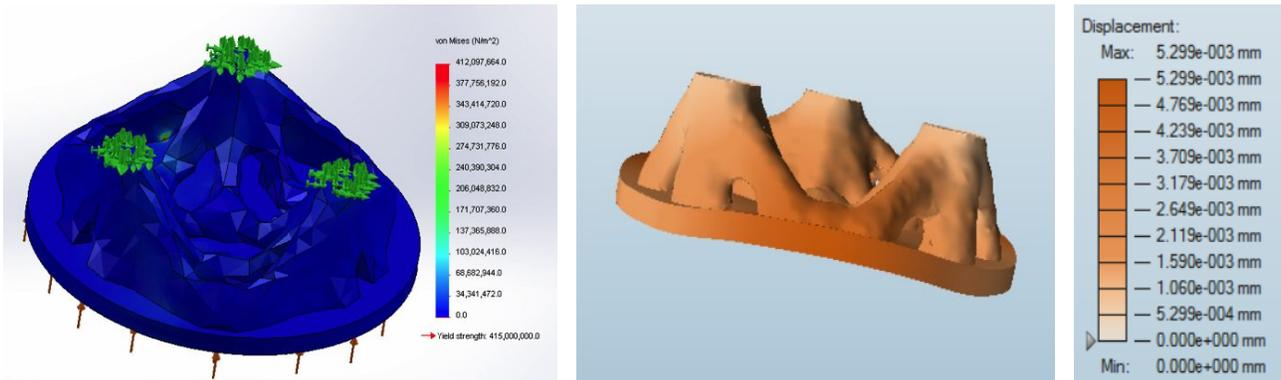
Figure 10. SolidWorks top mount titanium von mises stress analysis (a, left), top mount displacement analysis using 250N radial pressure point forces (b, right)
