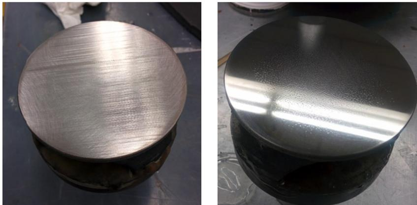
Figure 7. Titanium polishing progression:  $30\mu\text{m}$  diamond embedded pad (a, left), best surface finish (b, right)
