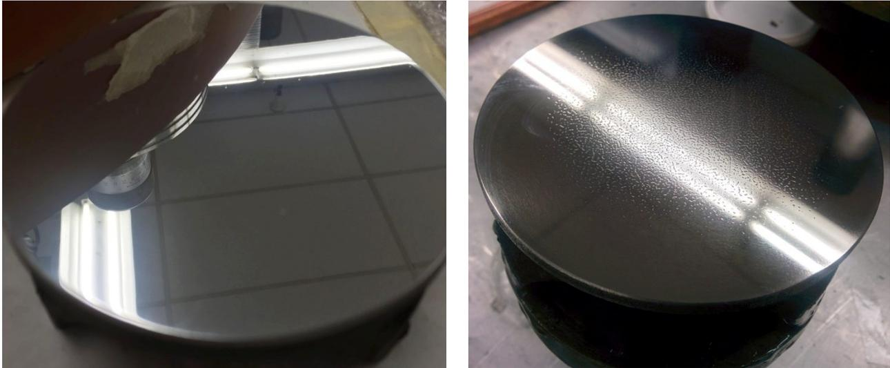
Figure 13. Final aluminum mirror surface finish (a, left), final titanium mirror surface finish (b, right)
