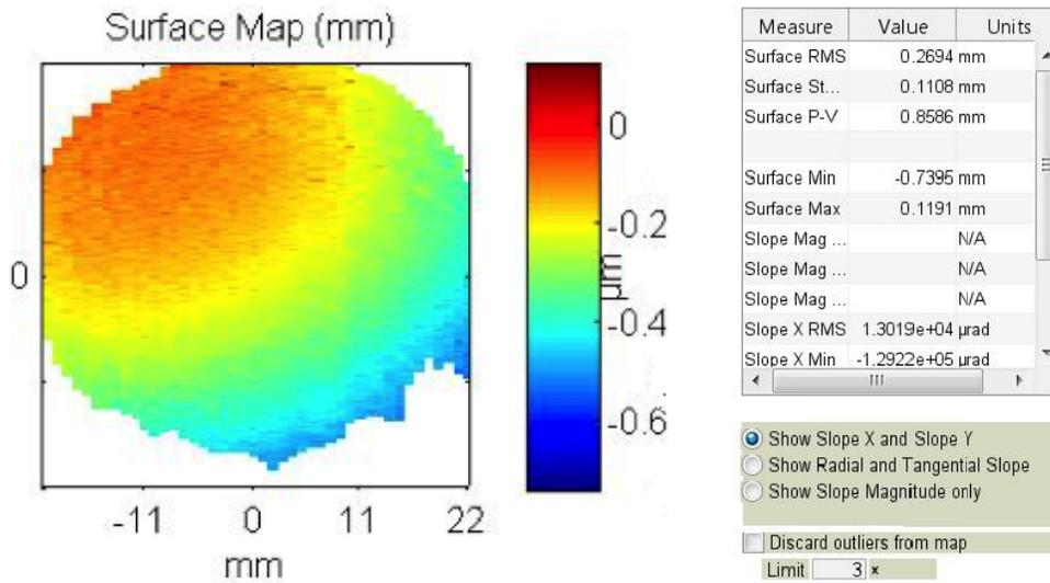
Figure 3. Surface data as seen in SAGUARO GUI<sup>[1]</sup> (Please, note that only some parts of the mirror were scanned due to metrology hardware limitations.)
