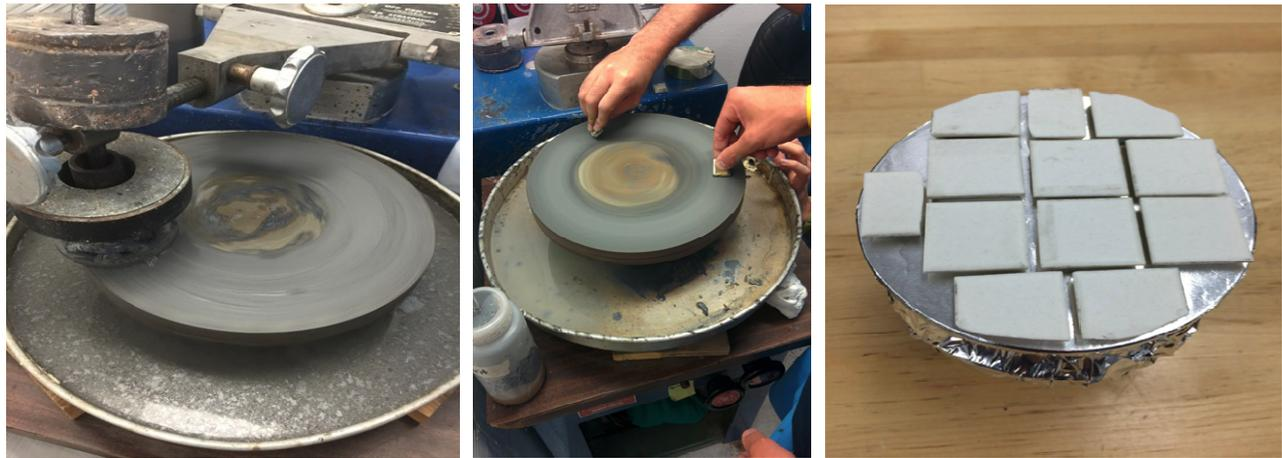
Figure 6. Grinding aluminum mirror flat (a, left), beveling ceramic tiles (b, center), completed ceramic grind tool (c, right)
