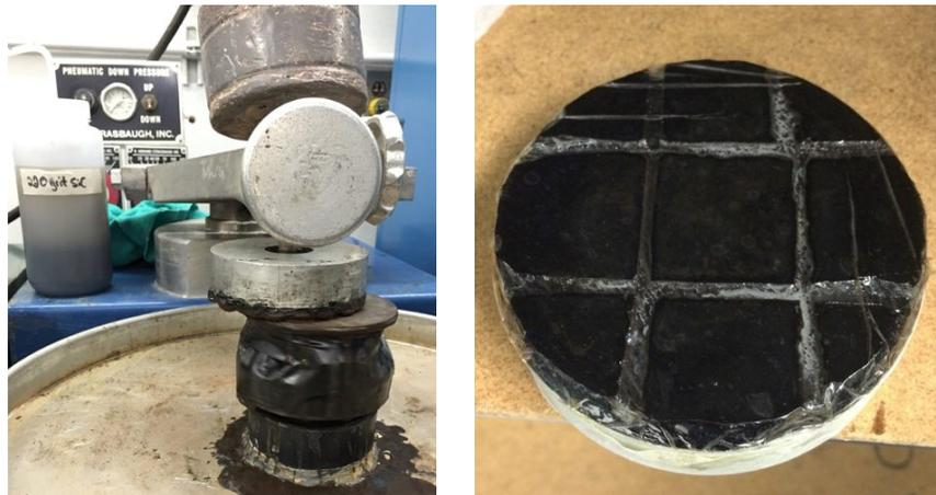
Figure 5. Grinding spindle and SiC grit (a, left), completed pitch grinding tool (b, right),
