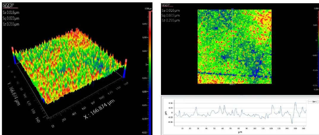
Figure 12. ZYGO interferometer 3D surface view of aluminum mirror (a, left), surface data from aluminum mirror (b, right)
