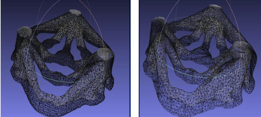
Figure 14. MeshLab faces reduction: 59,300 faces (a, left), MeshLab 20,000 faces (b, right)
