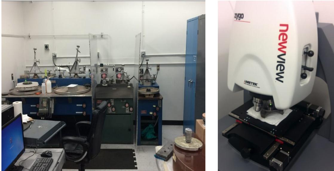
Figure 11. Optomechanics grinding and polishing lab setup (a, left), ZYGO interferometer used for analysis testing (b, right)
