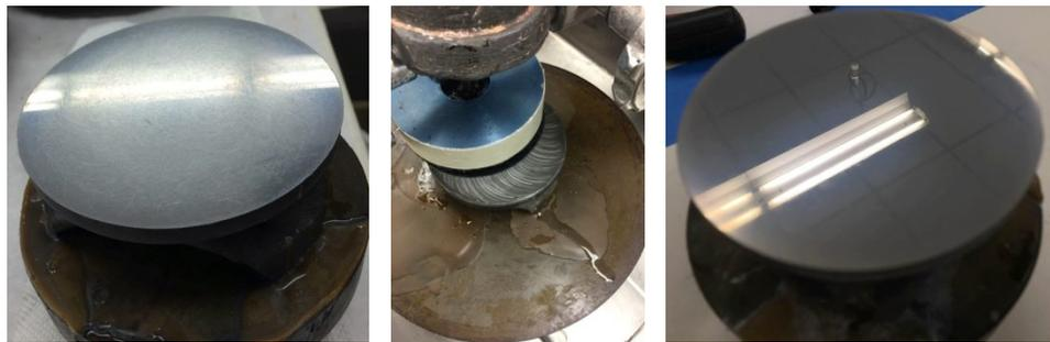
Figure 9. Aluminum polishing progression:  $3\mu\text{m}$  compound (a, left), polishing  $0.25\mu\text{m}$  (b, center), best finish (c, right)
