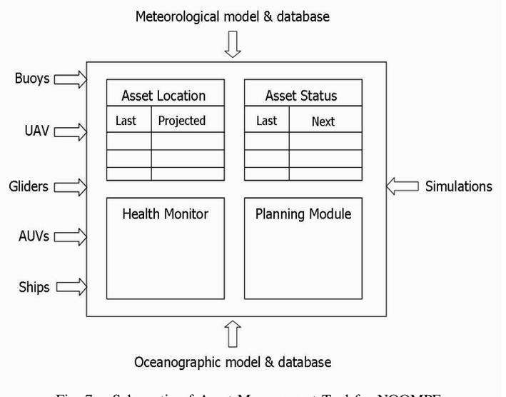
Fig. 7. Schematic of Asset Management Tool for NOOMPF.
