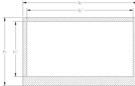
**Figure 66** – Calculus model for the Moment of Inertia ( $I$ )
