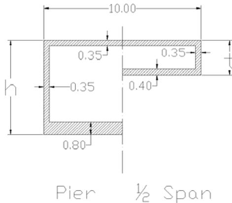
**Figure 59** – Cross in the Pier and  $\frac{1}{2}$  Span sections [m]
