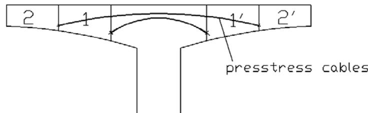
**Figure 3** – Scheme of the cantilever method starting from a pier
