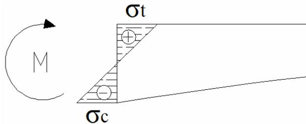
**Figure 79** – Diagram of Tensions in the pier section
