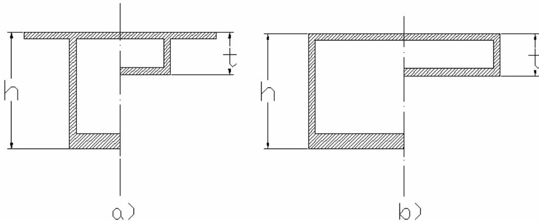
**Figure 2** – Box girder section at the pier section and at mid span, respectively.
