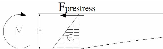
**Figure 80** – Calculus model for the prestressing force – Diagram of Tensions desired
