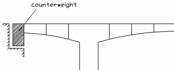
**Figure 6** – Construction of a deck using the cantilever method and a counterweight on the opposite side
