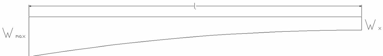
**Figure 81** – Variables for the calculation of the volume of prestress tendons ( $V_t$ )
