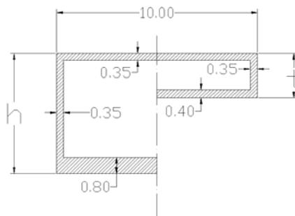
**Figure 70** – Cross in the Pier and  $\frac{1}{2}$  Span sections [m]
