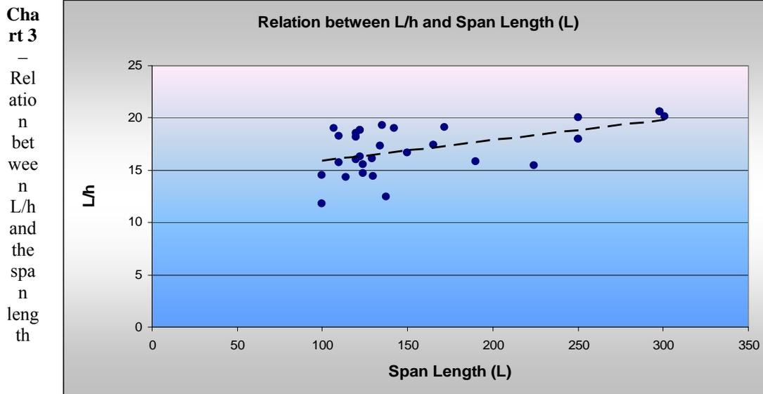
A closer look at **Chart 3** allows us to know that almost all the  $L/h$  values are between 15 and 20. From the trendline traced we can also see that the longer the span gets, the closer  $L/h$  is to 20. The highest  $L/h$  value is 23.7 – *Deutzer Bridge*, **Figure 41** – and the lowest is 12 – *Avignon Bridge*, **Figure 38**.
