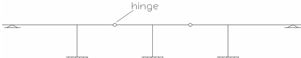
**Figure 7** – Bridge built with the cantilever Method using a central hinge
