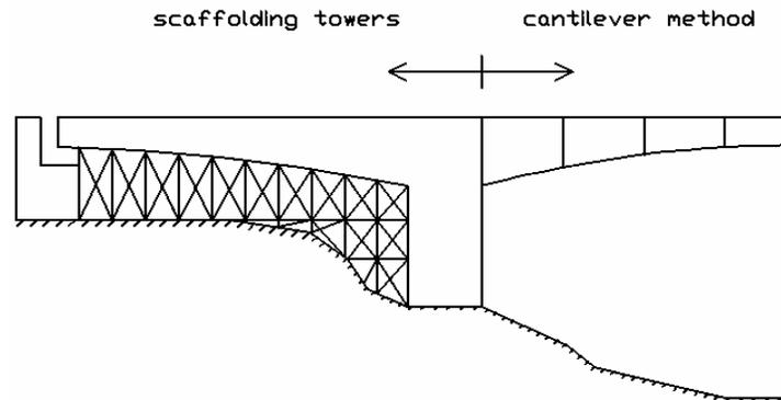
**Figure 5** – Construction of a deck using the cantilever method and scaffolding towers
