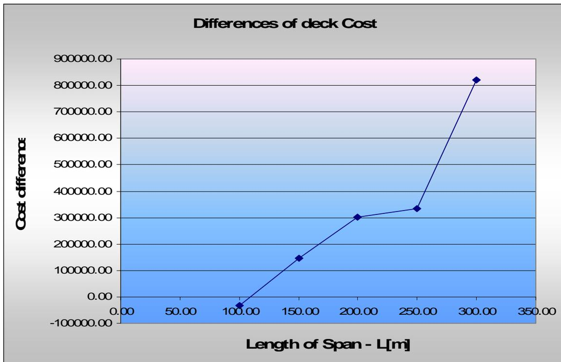
**Chart 7** – Variation of the deck cost differences according to the length of span
