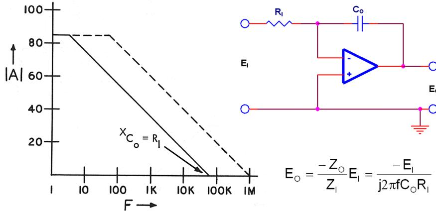
**Figure 46. Integrator Circuit**
