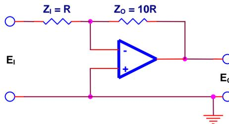
**Figure 30. Amplifier Circuit Using a Real Operational Amplifier**
