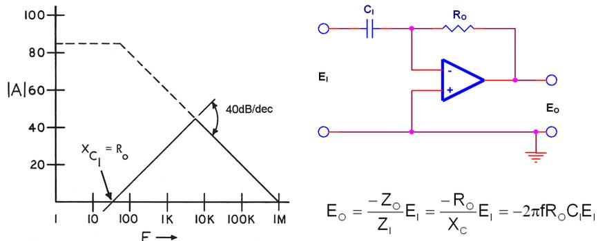
**Figure 43. Differentiator Circuit**
