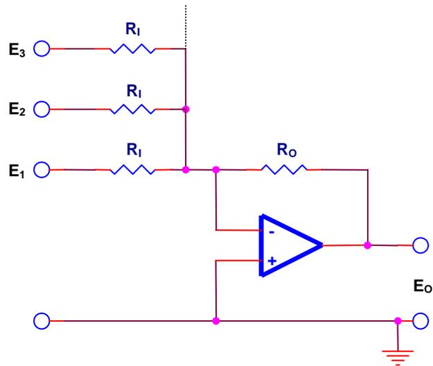
$$E_o = -\frac{R_o}{R_1}(E_1 + E_2 + E_3 + \dots)$$
