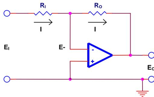
Let the voltage at the inverting input be  $E_-$  and the open loop operational amplifier gain be  $A$  (ideally,  $A = \infty$ ).
