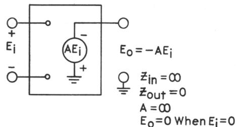
**Figure 9. Equivalent Circuit of the Ideal Operational Amplifier**
