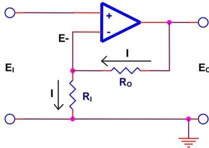
Let the voltage at the inverting input with respect to the non-inverting input be  $E_-$  and the gain of the operational amplifier be  $A$  (ideally,  $A = \infty$ ).
