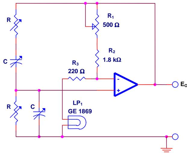
$$f_o = \frac{1}{2\pi RC}, 100 \text{ to } 6000 \text{ Hz}$$
