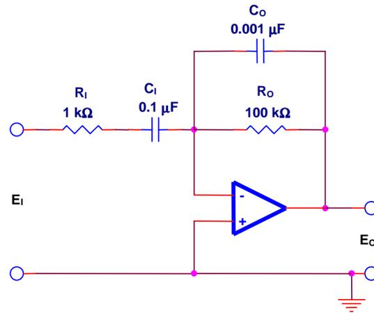
$$R_1 C_1 = R_o C_o \text{ drift compensating resistor}$$
