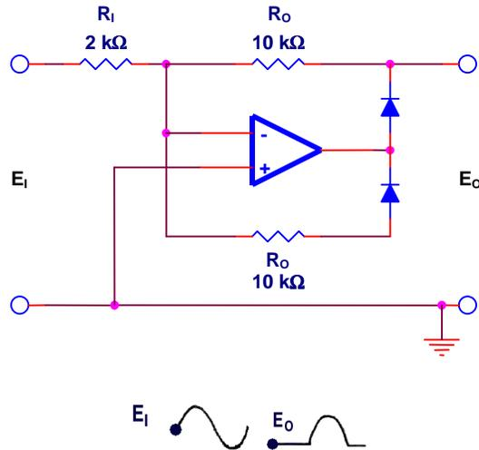
$$E_o \text{ peak} = \frac{-R_o}{R_i} E_i \text{ peak} = -5E_i \text{ peak}$$
