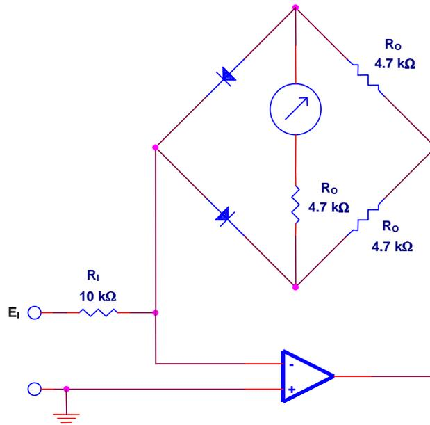
$$I_{\text{meter}} = \frac{E_i}{3R_1} = \frac{E_i}{30} \text{ mA}$$
