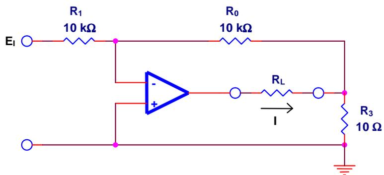
$$\frac{I}{E_1} = \frac{-R_0}{R_1 R_3} = -100 \text{ mA / Volt}$$
