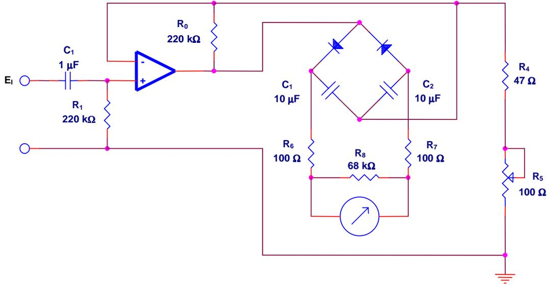
$$\text{Meter reading} = \frac{0.9E_1}{R_4 + R_5} \text{ (rms)}$$
