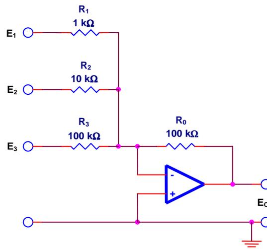
$$E_O = \left( \frac{R_0}{R_1} E_1 + \frac{R_0}{R_2} E_2 + \frac{R_0}{R_3} E_3 \right) = -100(100E_1 + 10E_2 + E_3)$$
