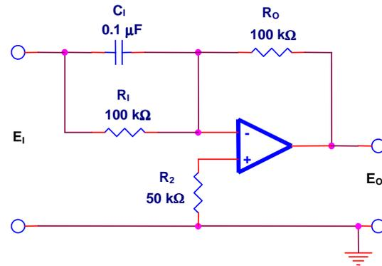
$$E_o = \frac{-R_o E_i}{R_1} - R_o C_1 \frac{dE_i}{dt}$$
