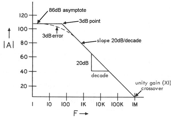
**Figure 33. Sketching the Bode Plot Approximation for Figure 32**
