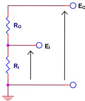
**Figure 16. Non-Inverting Amplifier Analyzed as a Voltage Divider**
