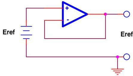
Prevent damage to standard cells induced by drawing current from them with low impedance (20 K $\Omega$  / Volt) measuring devices. See section on Buffers and Isolators for gain error. Offset adjustments should not be made with standard cell connected.
