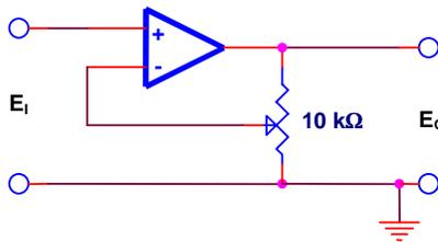
Equivalent to replacing both resistors in the non-inverting amplifier. Observe common mode voltage limit.
