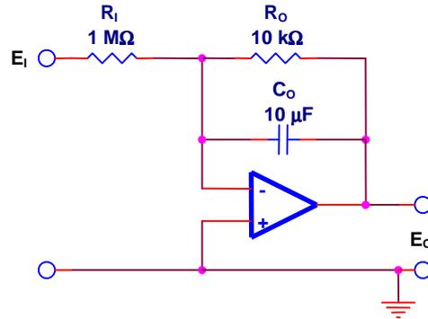
$$E_o = \frac{-R_o}{R_1} \frac{E_i}{1 + R_o C_o P} = \frac{-10E_i}{10 + P}$$
