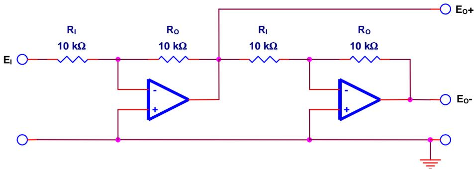
By using  $E_{O-}$  terminal at the reference, a p-p swing of  $4E_i$  is obtainable at  $E_{O+}$ , i.e. a usable swing greater than the power supply voltage rails. A fully differential operational amplifier provides this function in a single package, and is therefore the preferable design solution.
