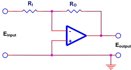
$$\frac{E_{\text{output}}}{E_{\text{input}}} = -\frac{R_O}{R_I}$$
