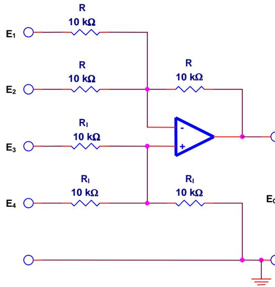
As an adder-subtractor, unused inputs should be grounded.
