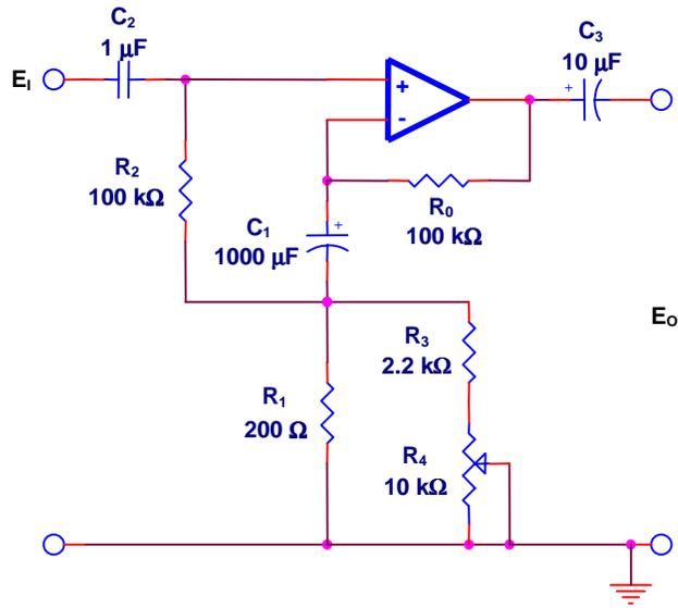
Completely developed AC amplifier with high  $Z_{in}$  and double rolloff rate and gain trim.
