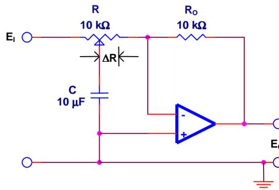
Non-integrating type. Constant inverting unity gain. Maximum lag for R centered for  $\Delta = \frac{1}{2}$  where  $0 \leq \Delta \leq 1$  is the log setting.
