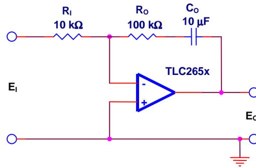
$$E_o = \frac{-R_o E_i}{R_1} - \frac{1}{C_o R_1} E_i dt$$
