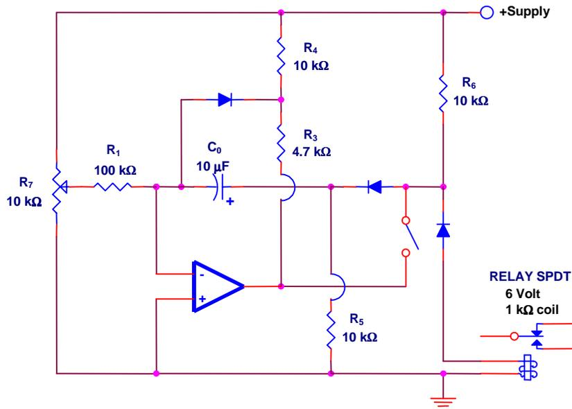
$$\text{Delay} = \frac{R_1 C_0}{2K_1}$$
