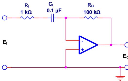
$$\text{High frequency cutoff: } F_o = \frac{1}{2\pi R_i C_i} = 0.6 \text{ kHz}$$
