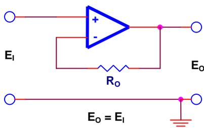
**Figure 13. Feedback Resistor Added to the Voltage Follower**
