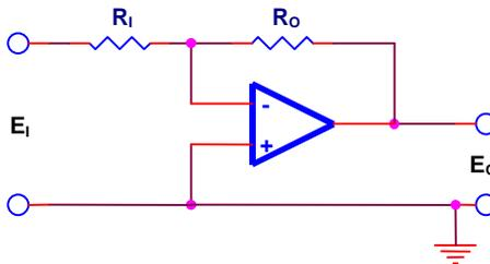
**Figure 29. Equivalent Circuit of a Real Operational Amplifier**
