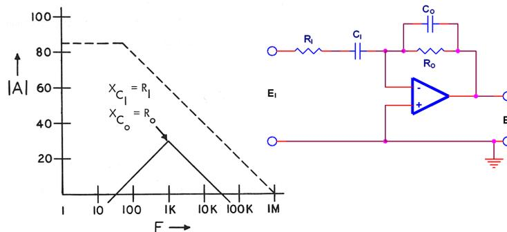
Figure 45. Differentiator With “Double Stop”
