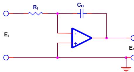
$$E_o = \frac{-Z_o}{Z_i} E_i = \frac{-E_i}{R_i C_o p} = -\frac{1}{R_i C_o} E_i dt$$
