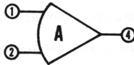
These numbers in the circles referred to pin numbers of old op amps, which were potted modules instead of integrated circuits. Many references to these numbers were made in the text, and these have been changed, of course.
