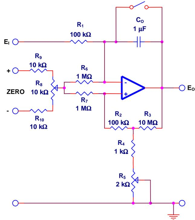
1. With input open and regeneration control  $R_5$  in approximate center of its range, open reset switch and adjust zero control,  $R_8$ , until output remains at zero.
