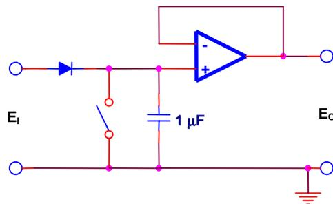
Peak value memory. Use low leakage capacitor.  $E_o = E_i$  maximum. Common mode input voltage must be observed.
