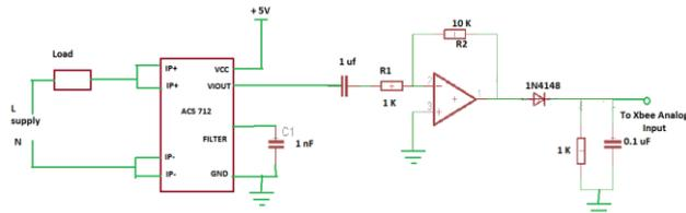
Fig.4 (b) Current Measurement using ACS712 Current sensor.
