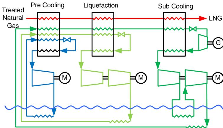
**Figure 14. A triple cycle mixed refrigerant cascade**
