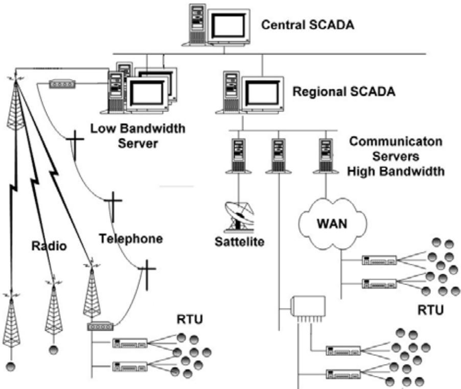
**Figure 32. SCADA system topology (typical)**
