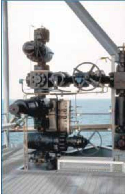
A typical Christmas tree, composed of a master gate valve, a pressure gauge, a wing valve, a swab valve and a choke is shown above. The
