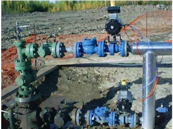
We differentiate between, dry completion (which is either onshore or on the deck of an offshore structure) and subsea completions below the surface. The wellhead structure, often called a Christmas tree, must allow for a number of operations relating to production and well workover. Well workover refers to various technologies for maintaining the well and improving its production capacity.
