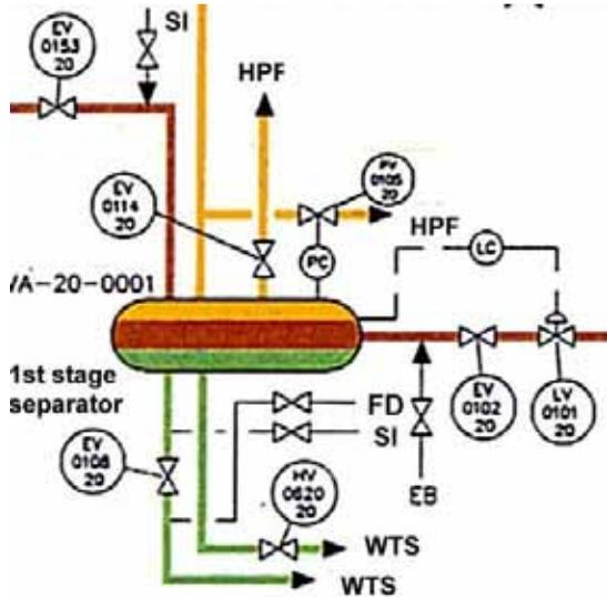
Emergency shutdown actions are defined in a cause-and-effect chart based on a HAZOP of the process. This study identifies possible malfunctions and how they should be handled.
