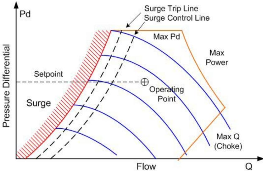
**Figure 8. Compressor state diagram**
