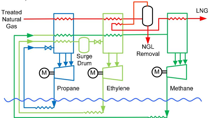
Figure 15. Optimized cascade process
