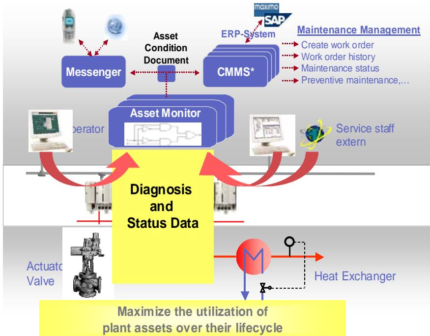
**Figure 34. Computerized maintenance management system**
