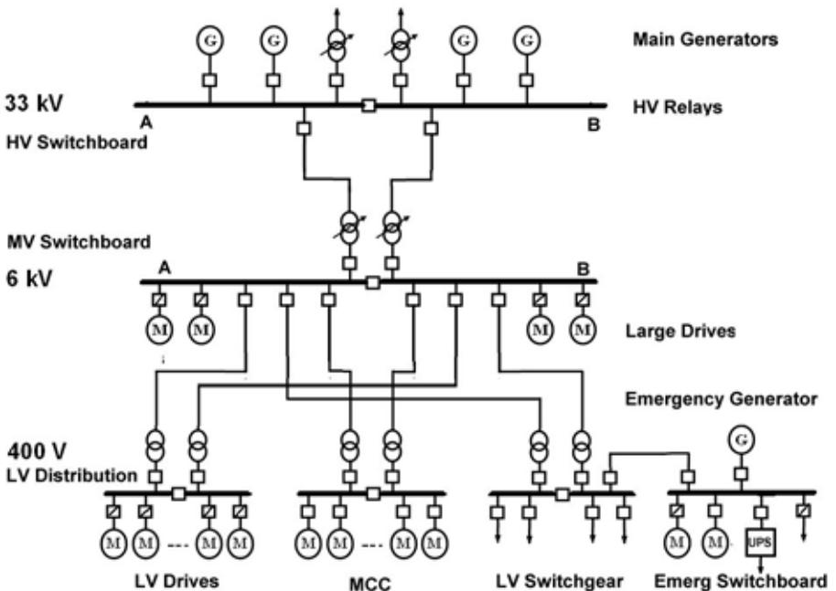
Figure 36. Electrical single line diagram
