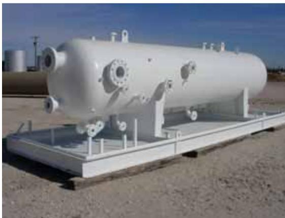
In gravity separation, the well flow is fed into a horizontal vessel. The retention period is typically five minutes, allowing gas to bubble out, water to settle at the bottom and oil to be taken out in the middle. The pressure is often reduced in several stages (high pressure separator, low pressure separator, etc.) to allow controlled separation of volatile components. A sudden pressure reduction might allow flash vaporization leading to instability and safety hazards.
