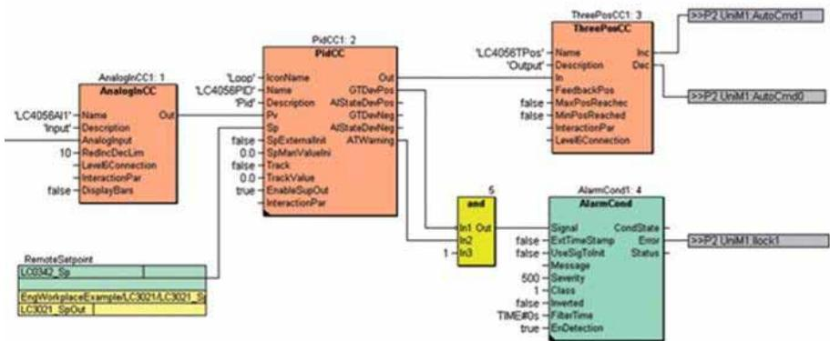
**Figure 31. Function blocks define the control**
