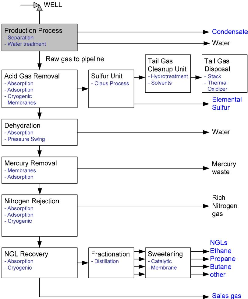
Figure 10. Typical gas plant
