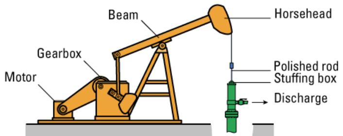
motor drives a reciprocating beam, connected to a polished rod passing into the tubing via a stuffing box. The sucker rod continues down to the oil level and is connected to a plunger with a valve.
