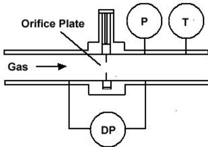
Orifice plates are sensitive to a buildup of residue and affect the edges of the hole. Larger new installations therefore prefer ultrasonic gas meters that work by sending multiple ultrasonic beams across the path and measure the Doppler effect.
