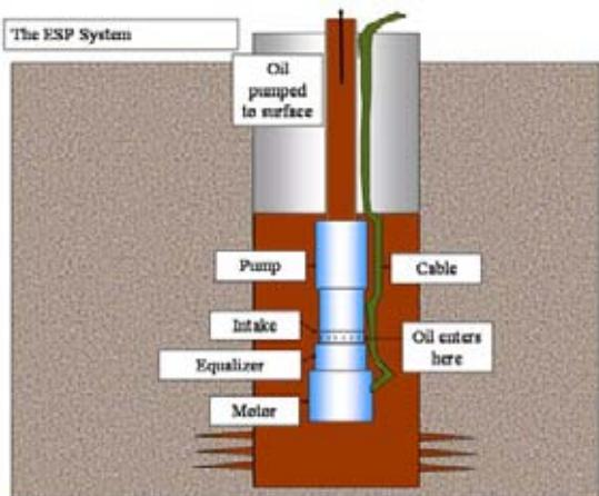
Installations down to 3.7 km with power up to 750 kW have been installed. At these depths and power ratings, medium voltage drives (up to 5kV) must be used.
