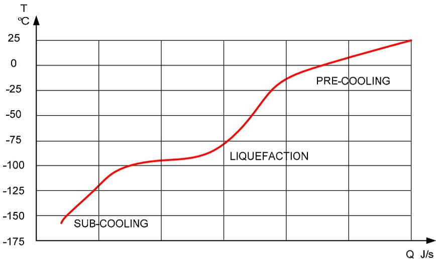
**Figure 13. LNG Q/T diagram**
