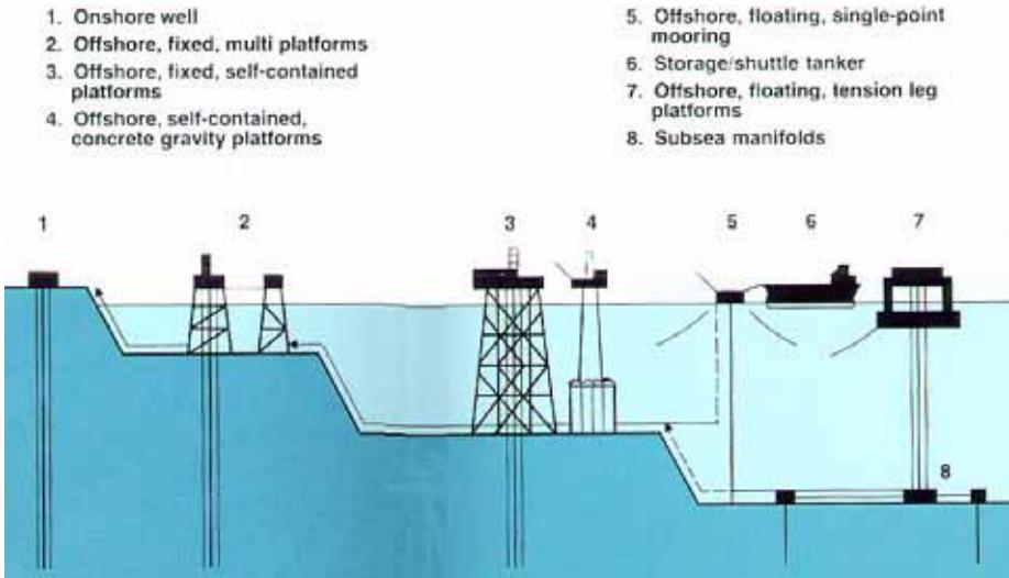
**Figure 1. Oil and gas production facilities**
