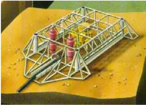
Control is from the surface, where a hydraulic power unit (HPU) provides power to the subsea installation via an **umbilical**. The umbilical is a composite cable containing tension wires, hydraulic pipes, electrical power, control and communication signals. A control pod with inert gas and/or oil protection contains control electronics, and operates most equipment via hydraulic switches. More complex subsea solutions may contain subsea separation/stabilization and electrical
