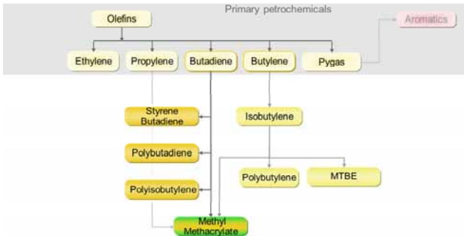
**Figure 29. Olefins – butadiene, butylene, and pygas, derivatives**
