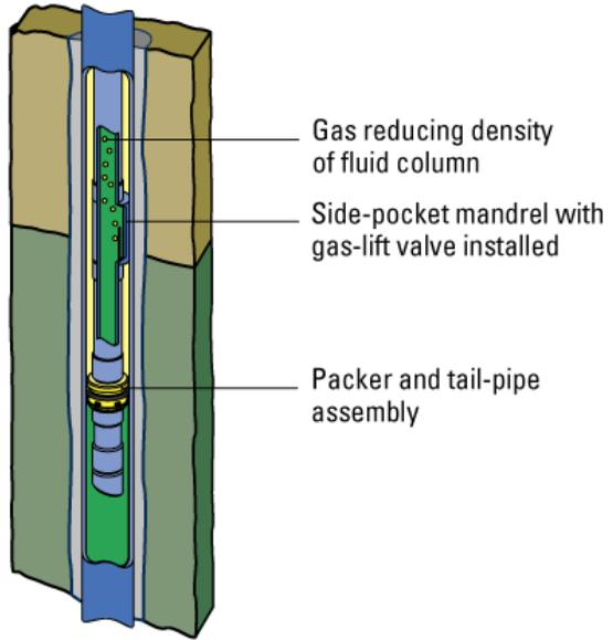
The valve will open at a set pressure to inject lift gas into the tubing. Several mandrels with valves set at different pressure ranges can be used to improve lifting and startup. III: Schlumberger oilfield glossary
