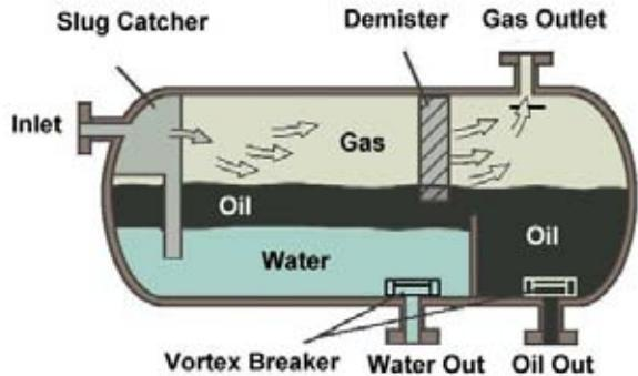
The retention period is typically 5 minutes, allowing gas to bubble out, water to settle at the bottom and oil to be taken out in the middle. In this platform the water cut (percentage water in the well flow) is almost 40%, which is quite high. In the first stage separator, the water content is typically reduced to less than 5%.
