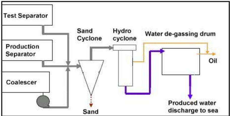
**Figure 6. Produced water treatment**
