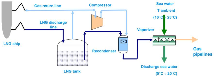
**Figure 18. LNG terminal process overview**
