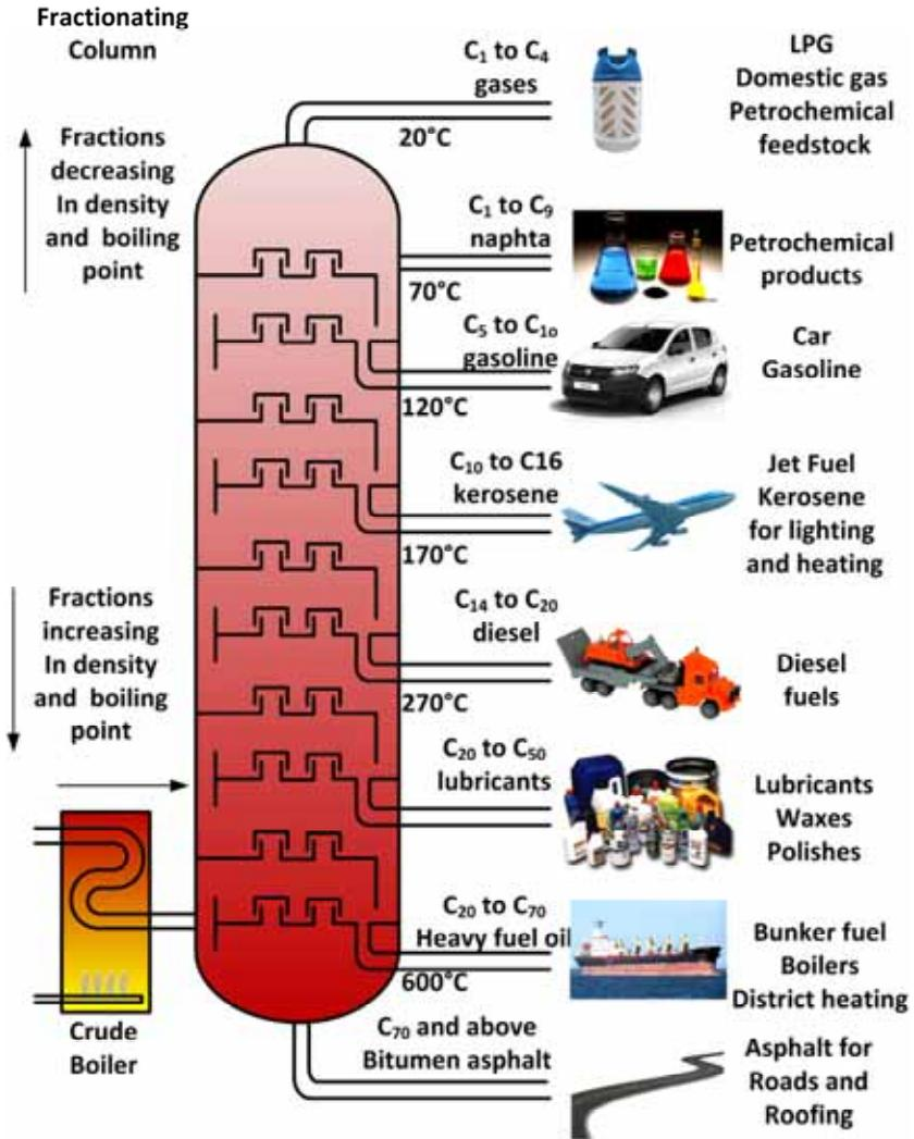
Figure 19. Fractionating continuous distillation, overview
