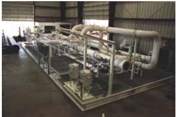
Typically, a metering installation consists of a number of meter runs so that one meter will not have to handle the full capacity range, and associated prover loops so that the meter accuracy can be tested and calibrated at regular intervals.
