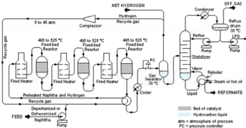
**Figure 21. Catalytic reformer** (Source: Wikipedia)
