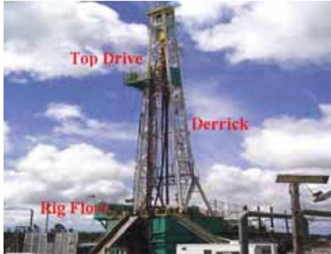
Earlier pictures of drillers and roughnecks working with rotary tables (bottom drives) are now replaced with top drive and semi-automated pipe handling on larger installations. The hydraulic or electric top drive hangs from the derrick crown and gives pressure and rotational torque to the drill string. The whole assembly is controlled by the drawworks. *Photo: Puna Geothermal Venture*
