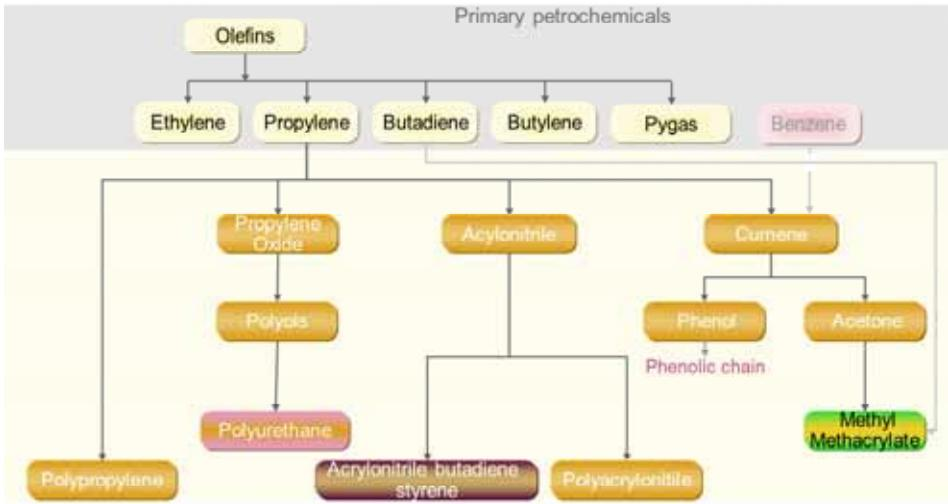
**Figure 28. Olefins – propylene, derivatives**
