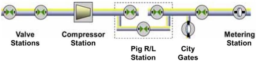
**Figure 11. Gas pipeline**
