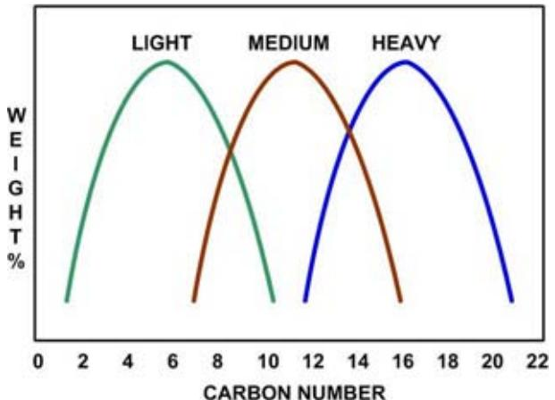
occurring 40 degrees API crude, fed to the distillation column at the refinery could come out of the still as 1.4 barrels of gasoline and naphtha (typically  $C_8H_{18}$ ), 0.6 barrels of kerosene (jet fuel  $C_{12-15}$ ), 0.7 barrels of diesel fuel (average  $C_{12}H_{26}$ ), 0.5 barrels of heavy distillate ( $C_{20-70}$ ), 0.3 barrels of lubricating stock, and 0.5 barrels of residue (bitumen, mainly poly-cyclic aromatics).
