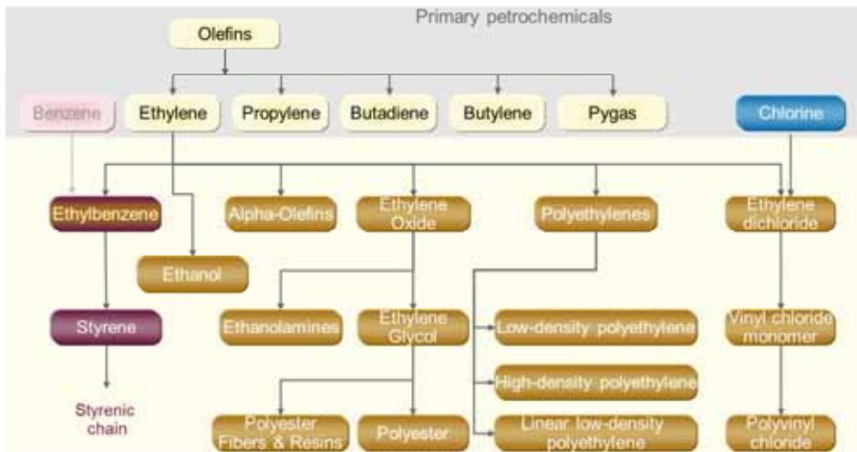
**Figure 27. Olefins – ethylene, derivatives**
