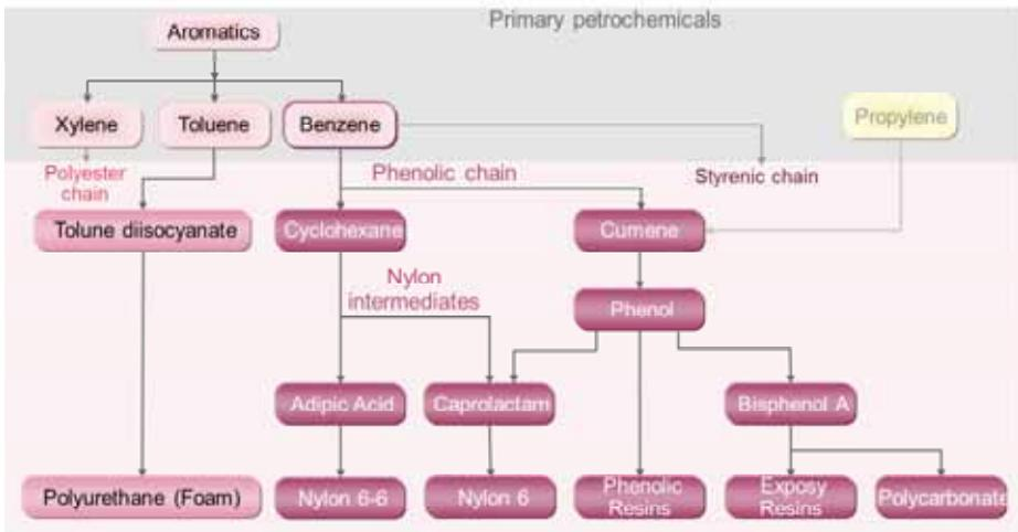
**Figure 25, Aromatics – toluene and benzene, polyurethane and phenolic chain**
