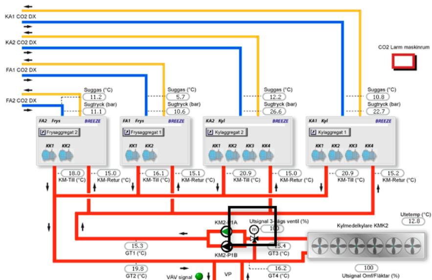
**Figure 6.13 - A picture from IWMAC of the machine room in TR1.**
