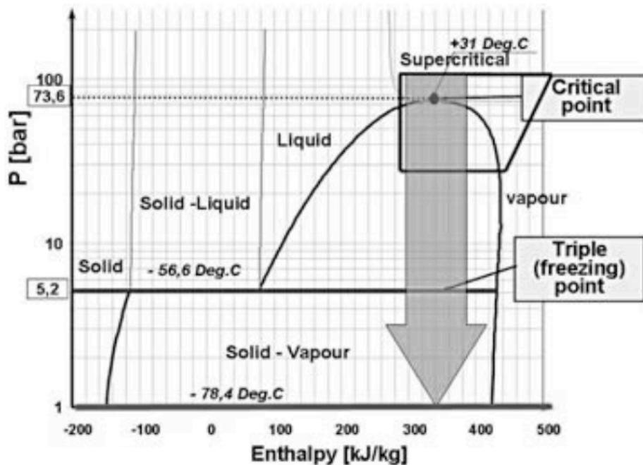
**Figure 4.7 - Phase change for CO<sub>2</sub> when solid ice is formed (GTZ Proklima, 2008).**
