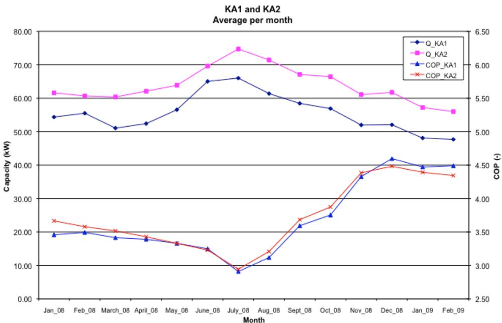
**Figure 6.7 - Monthly average of the cooling capacity and COP for the medium temperature units.**
