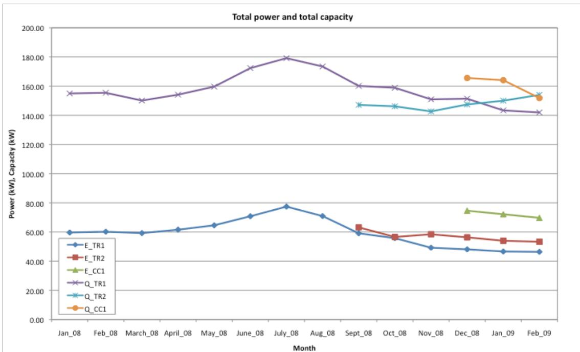
**Figure 7.4 - Total capacity and total compressor power consumption for all three systems**
