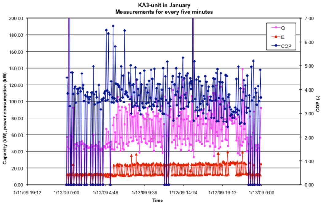
**Figure 6.17 - The power, capacity and COP of KA3-unit in January in TR2.**
