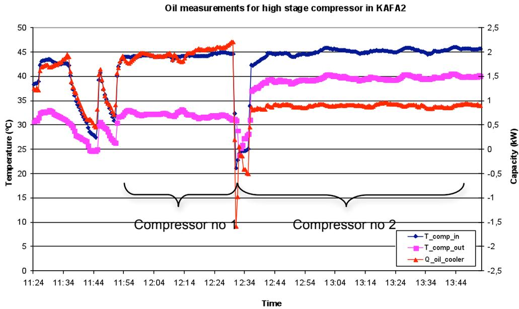
**Figure 5.6 - Temperature and calculated oil cooler capacity for two different compressors during a two-hour test**
