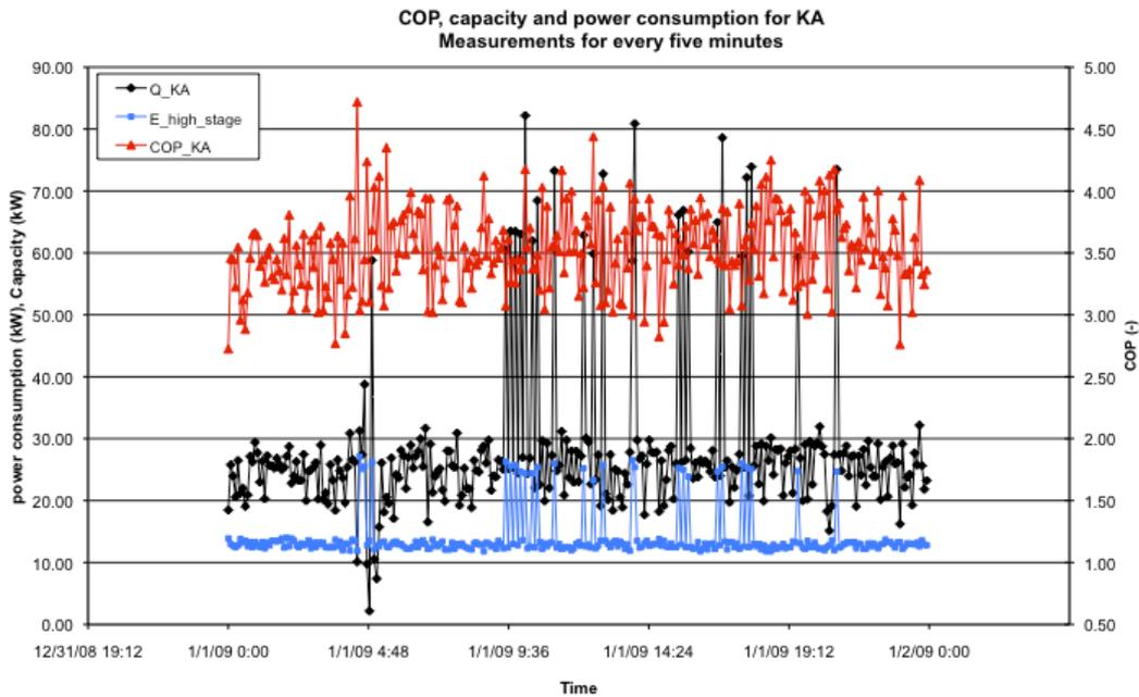
**Figure 6.24 - The power, capacity and COP for the chillers in KAFA-unit January in TR2.**
