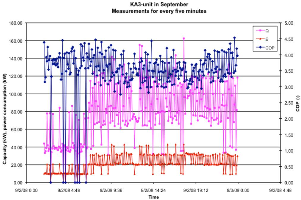
**Figure 6.16 - The power, capacity and COP of KA3-unit in September in TR2.**
