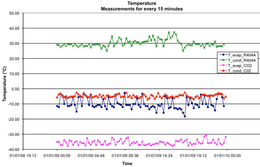
**Figure 6.27 - Temperature during 24 hours in January in CC1.**
