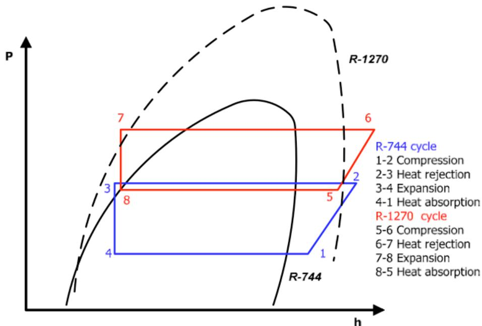
**Figure 4.4 - Log P-h diagram showing operation of cascade refrigeration system (Campbell et al., 2007).**
