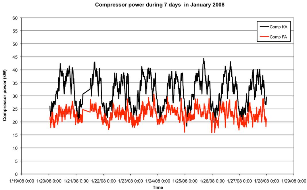
**Figure 6.2 - The total compressor power during 7 days in January in TR1**
