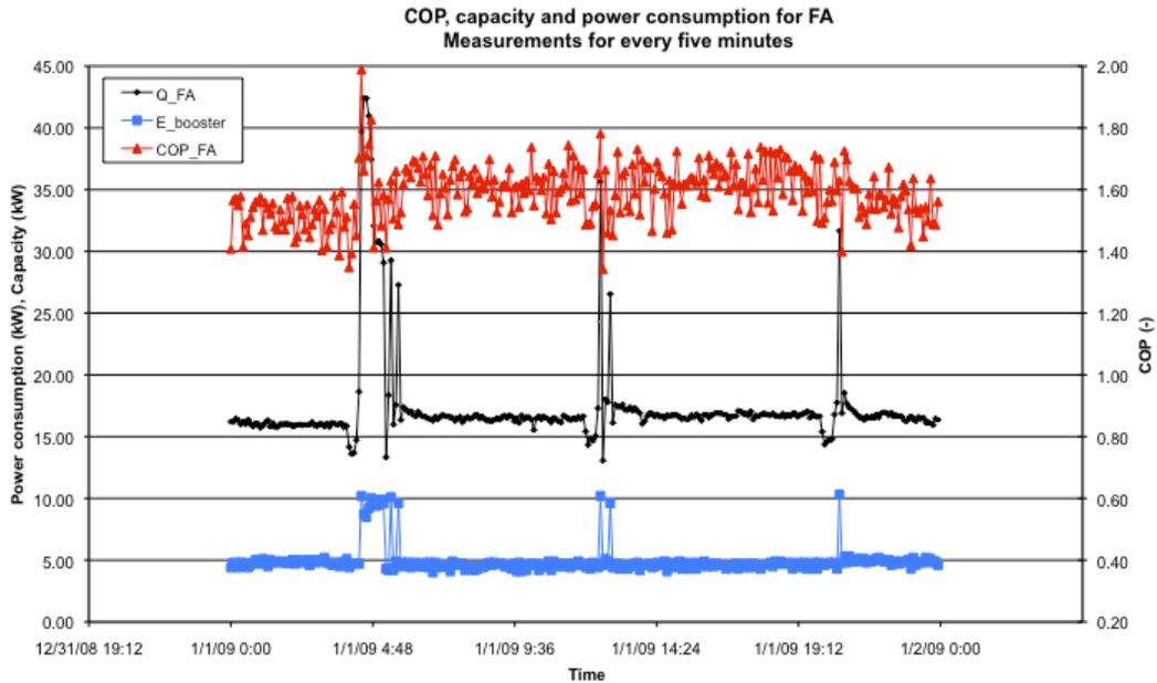
**Figure 6.25 - The power, capacity and COP for the freezers in KAFA-unit January in TR2.**
