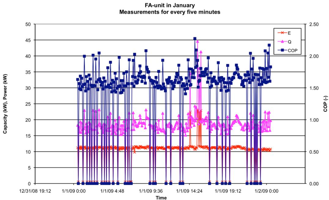
**Figure 6.10 - The power, capacity and COP of FA-unit in January in TR1**
