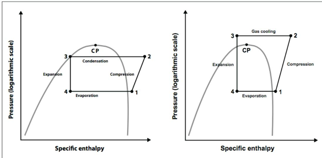
**Figure 4.5 - Basic subcritical and trans-critical refrigeration cycles (Danfoss, 2008).**
