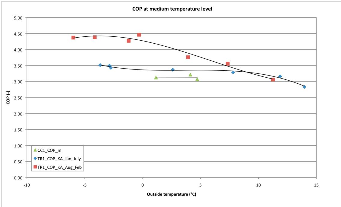
**Figure 7.8 - The COP at medium temperature level**
