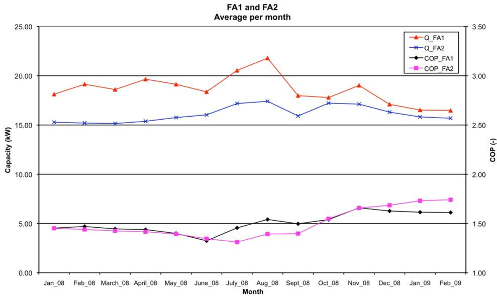
**Figure 6.6 - Monthly average of the cooling capacity and COP for the freezing units.**
