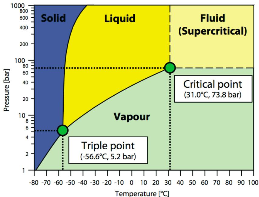
**Figure 4.1 - Phase diagram for carbon dioxide (Danfoss, 2008).**
