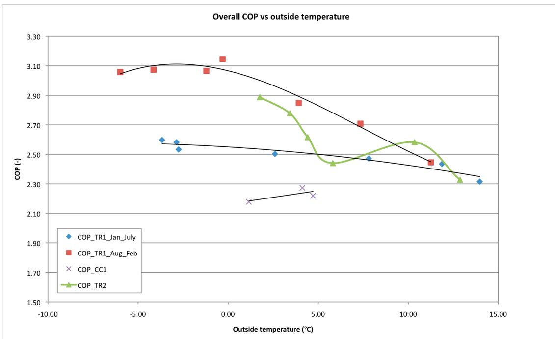
**Figure 7.6 – The relation between the overall COP and the outside temperature**
