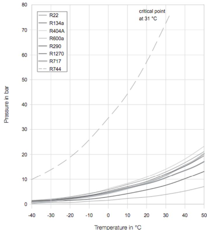
**Figure 4.2 - Temperature and pressure diagram showing the vapour pressure curve of some common refrigerant e.g carbon dioxide (R744) (GTZ Proklima, 2008).**
