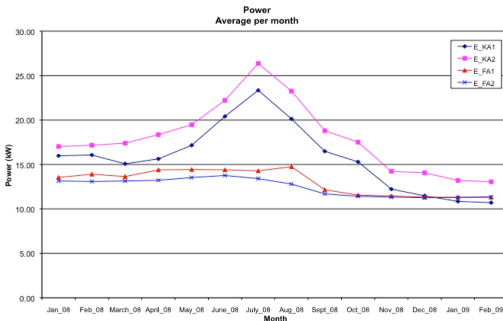
**Figure 6.1 - Monthly average of the compressor power for the four units in TR1.**
