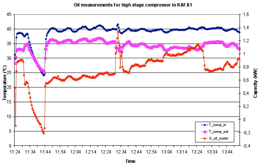
**Figure 5.7 - Temperature and calculated oil cooler capacity for one compressor during a two-hour test**
