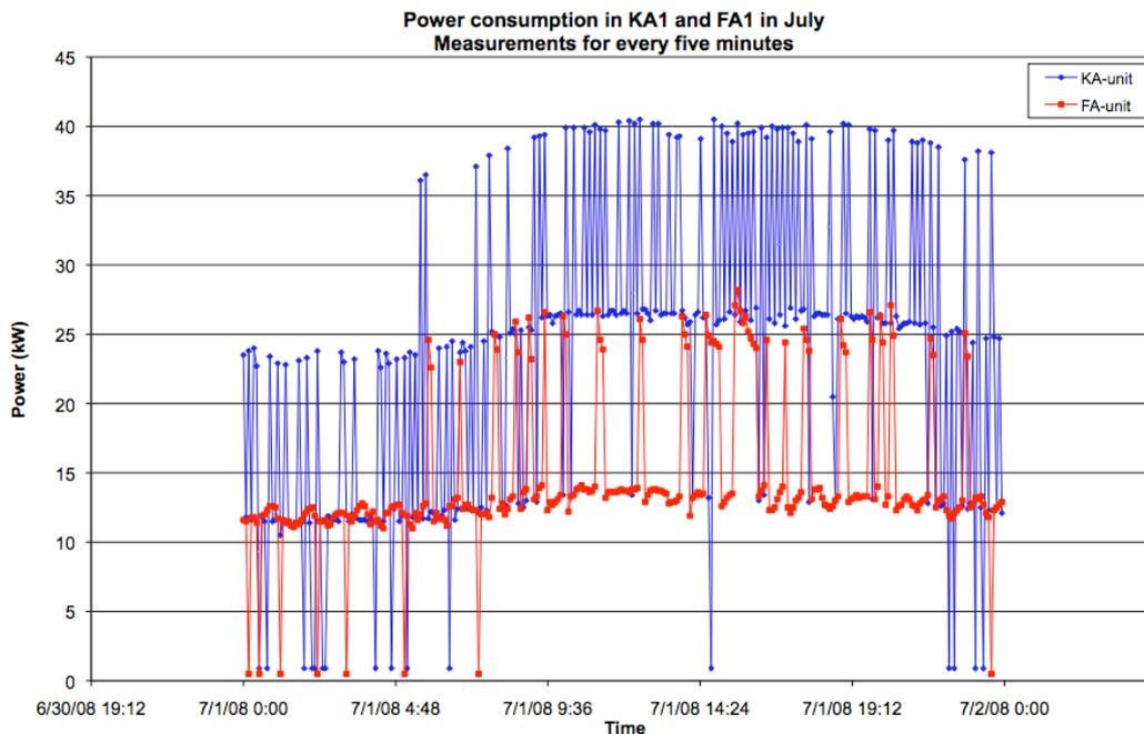
**Figure 6.5 - The compressor power for KA1 and FA1 in July in TR1**
