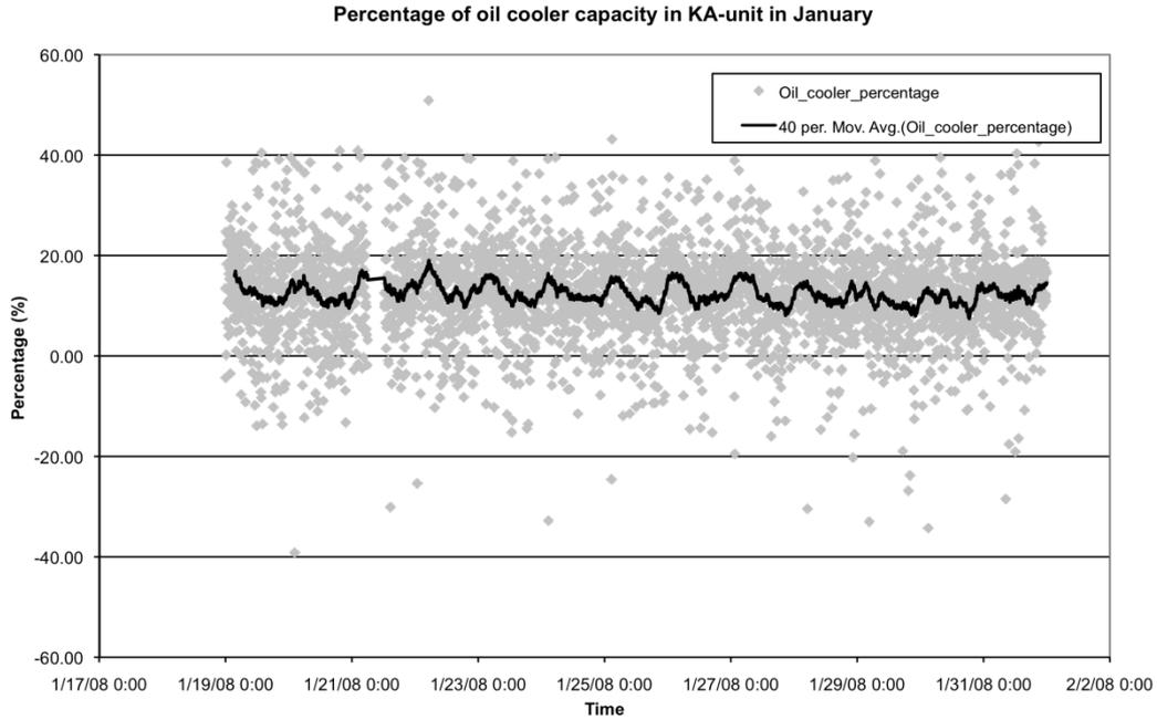
**Figure 5.8 - The oil cooler as a percentage of  $E_{el}$  for KA-unit in TR1 in January.**
