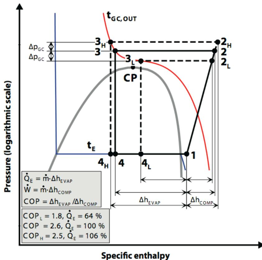
**Figure 4.6 - Log P-h diagram for carbon dioxide. Different gas cooling pressure results in different COP (Danfoss, 2008)**
