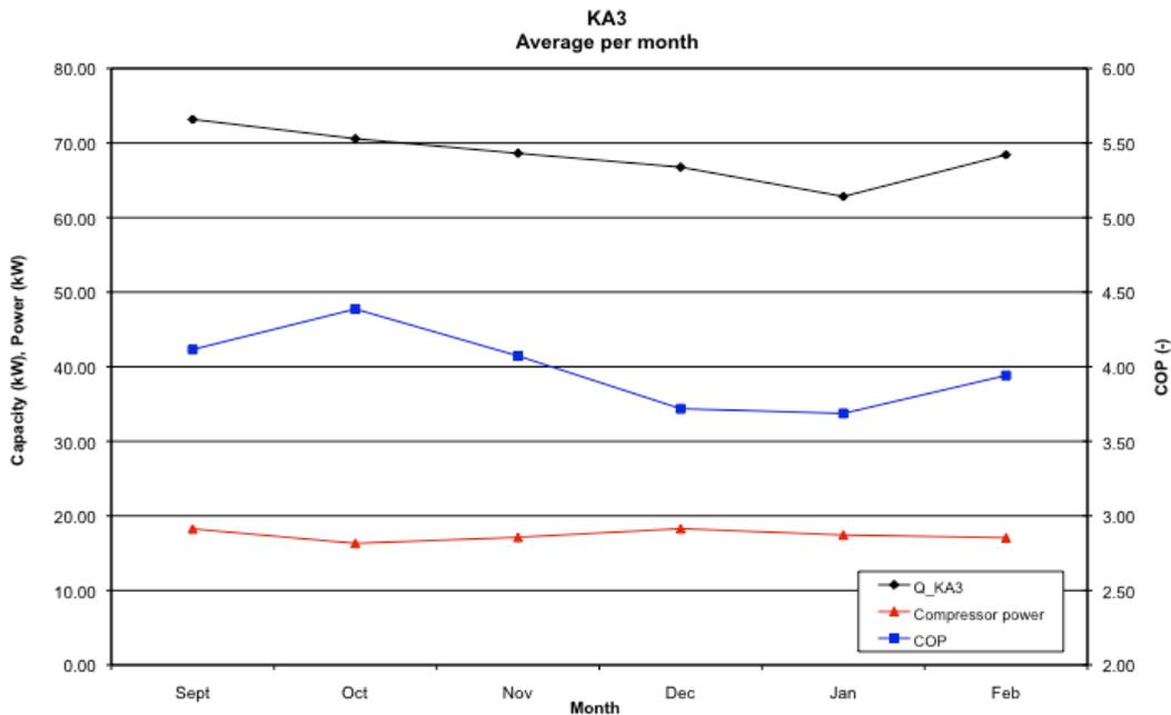
**Figure 6.15 - Monthly average of the COP, cooling capacity and compressor power for KA3-unit.**
