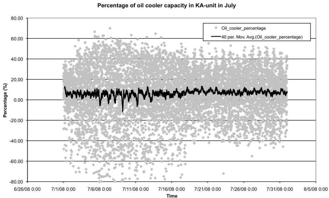
**Figure 5.9 - The oil cooler as a percentage of  $E_{el}$  for KA-unit TR1 in July.**
