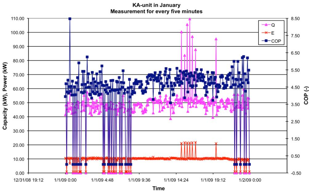
**Figure 6.8 - The power, capacity and COP of KA-unit in January in TR1**
