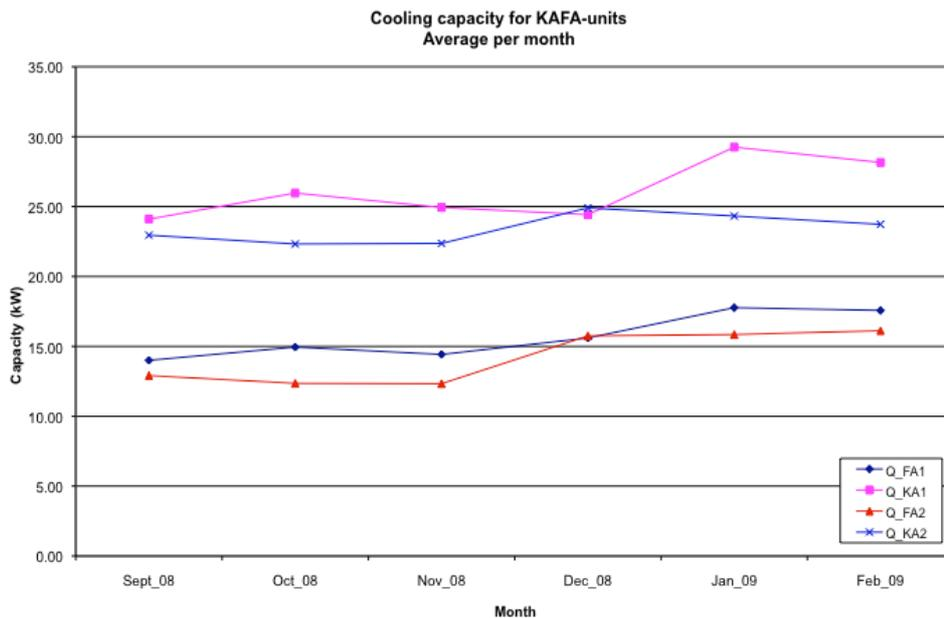
**Figure 6.20 - Monthly average of the cooling capacity in KAFA-units in TR2.**
