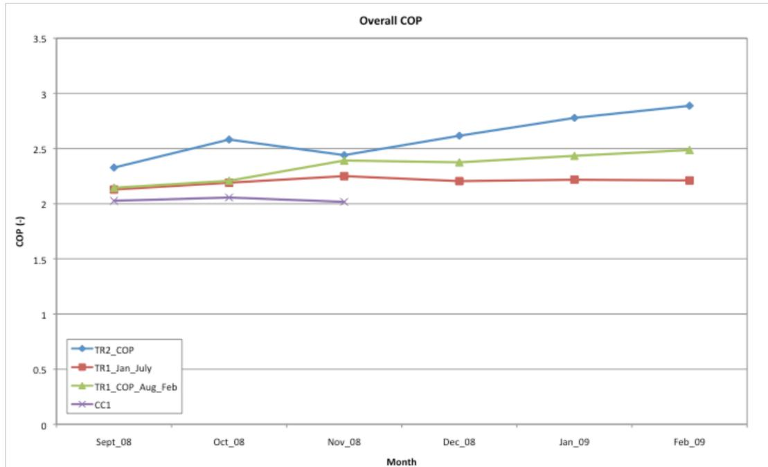
**Figure 7.10 – the overall COP if the supermarkets would have the same capacity and outside temperature conditions**
