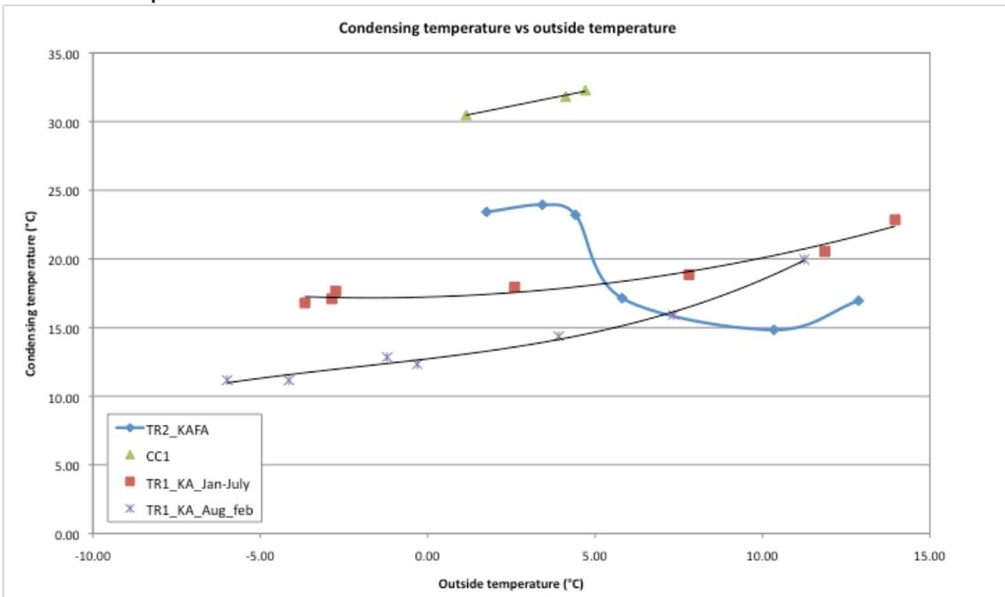
**Figure 7.3 – The relation between the condensing temperature and the outside temperature**
