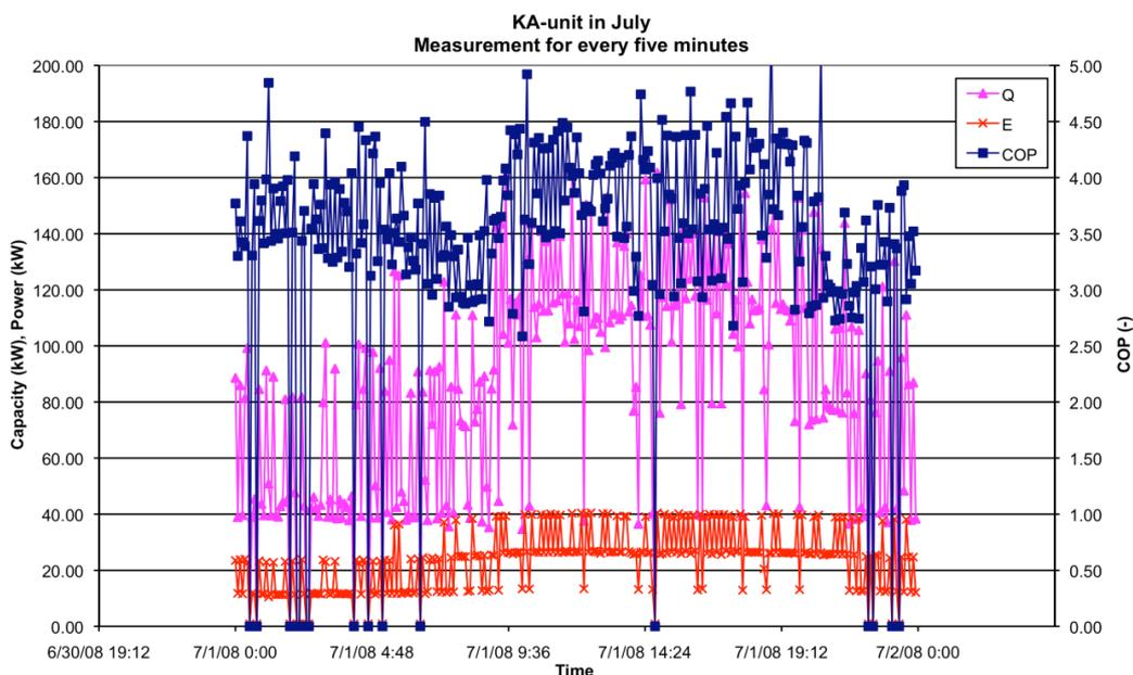
**Figure 6.9 - The power, capacity and COP of KA-unit in July in TR1**
