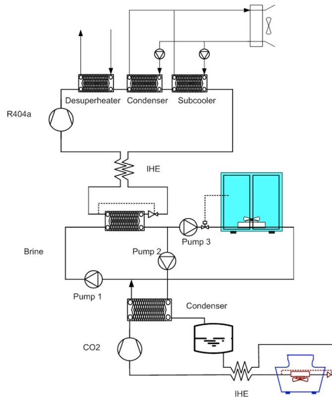
**Figure 5.10 - A Schematic diagram of cascade system 1.**
