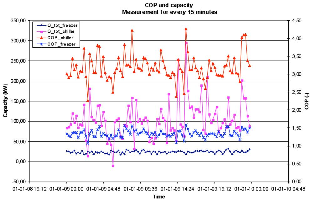
**Figure 6.26 - COP and capacity during 24 hours in January in CC1**
