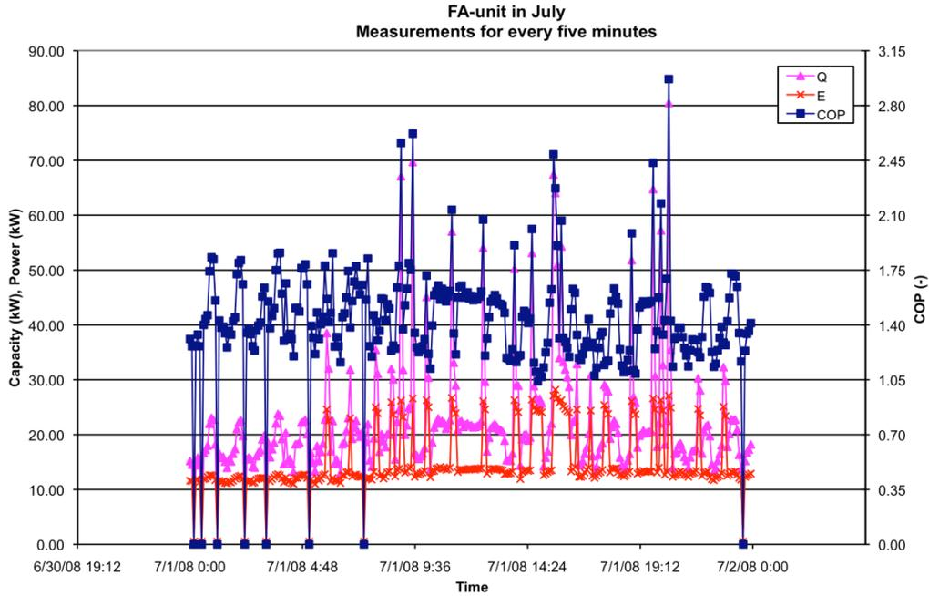
**Figure 6.11 - The power, capacity and COP of FA-unit in July in TR1**
