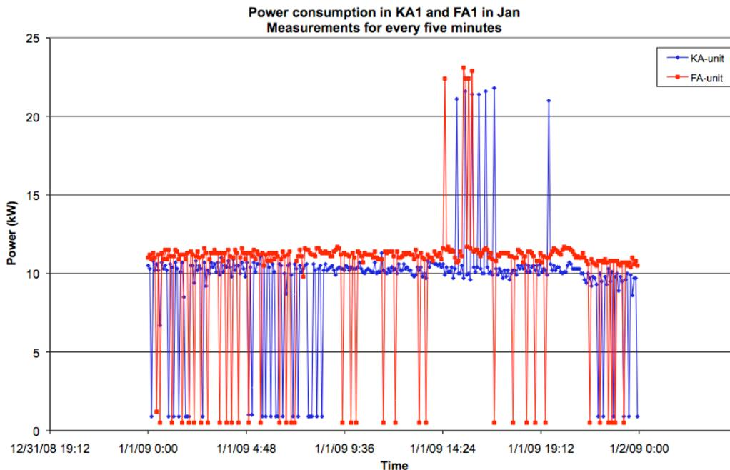
**Figure 6.4 - The compressor power for KA1 and FA1 in January in TR1.**
