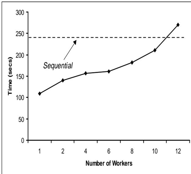
Figure 6: Performance of the verification system. For each worker participating in the computation the verifier picked  $I = 10\%$  of the submitted traces at random (in addition to the initialization and final states) and checked the correctness of each state transition against its locally reconstructed image. These results show that our approach represents an efficient method for verifying a worker’s supposed execution of a computational component.
