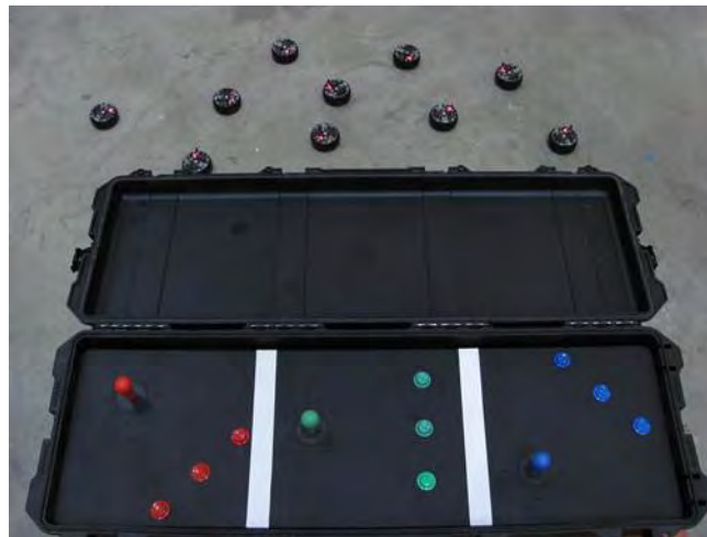
Fig. 8: User Interface for user control of the r-one “swarm”. The user can control a subset of the “swarm” and see how different behaviors work with a multi-robot system. Being able to control the r-one robots had a huge impact on attendees and drew a large crowd to the display.
