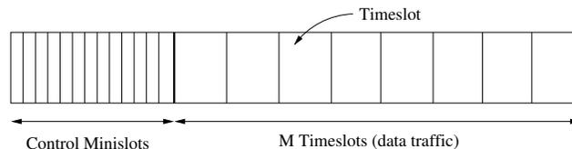
Fig. 1. Single Channel TDMA Frame Structure
