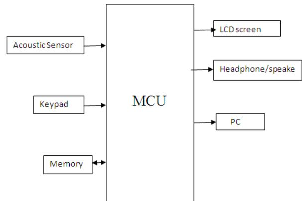
Fig 1: Basic Block diagram for digital stethoscope
