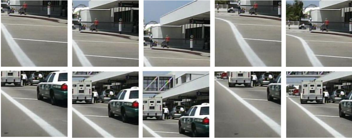
Fig. 2. Procedure for generating examples for training for the LFOV classifier: each of these examples is generated by positioning a pedestrian in the center of each cell of a 4x4 grid, in as many cell positions as possible.
