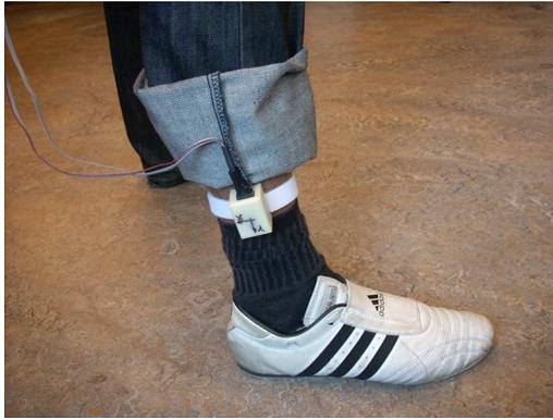
Fig. 9. IMU fixed to the ankle for gait analysis experiments.
