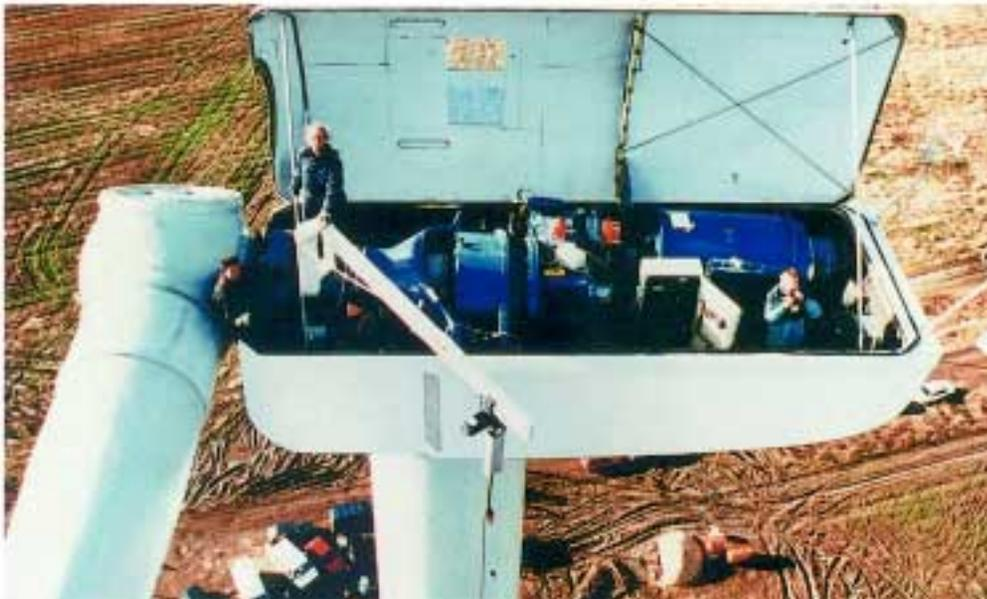
*FLENDER components in a drive of a wind power station*
