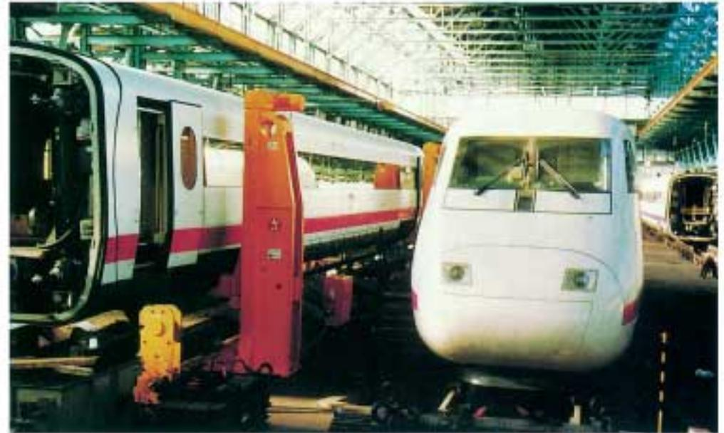
*MOTOX bevel geared motors driving lifting jacks for the maintenance of the ICE*
