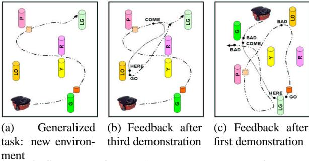
Figure 9: Structure of the environment and course of task execution during practice and feedback
