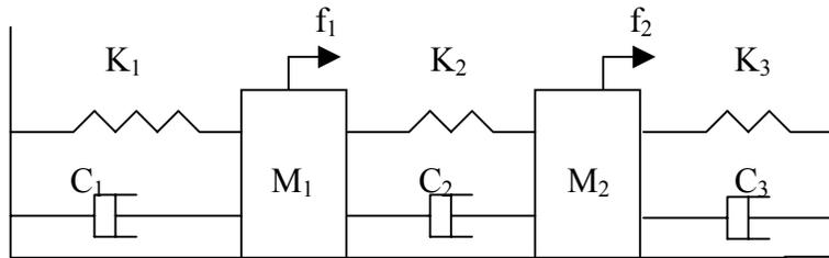
Derive the governing differential equation of motion and solve for the eigen values and the eigen vectors.
