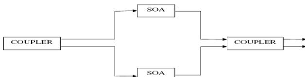
Fig 3.1 Optical logic using MZI switch
