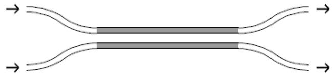
Fig 1.3 Directional Coupler Switch
