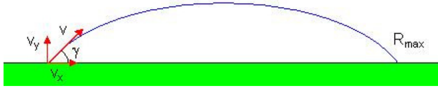
Figure 5: Trajectory plot of projectile with no air resistance i , where v is the launch velocity, and the angle of release is represented by the angle \gamma
