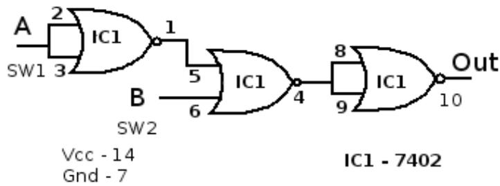
5. Solution with pinout below. It is optional to label Vcc and Gnd on the diagram. Most often for a chip, the Vcc is the upper most right pin and the Gnd is the bottom left, however the chip pinout should always be consulted.
