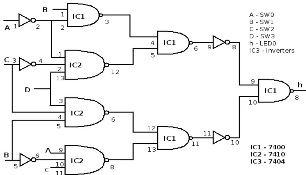
7. As the logic kit does not contain a four input NAND gate, combinations of three and two input NANDs are used. The following justification shows that this is indeed a correct implementation.
