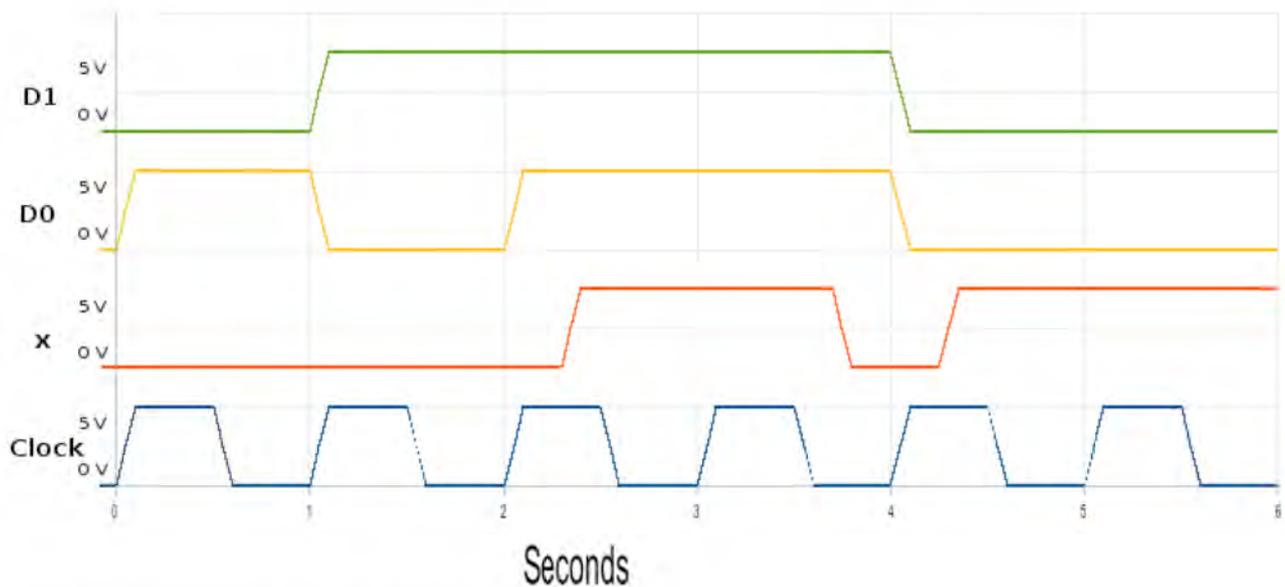
Exhibit 8.2.b: Timing diagram for four state counter
