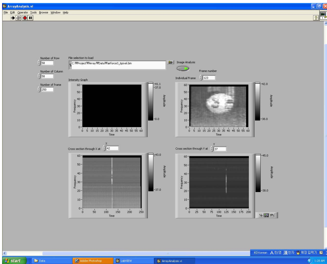
Figure 2.6 Parallel OCT analysis program in Labview. Detailed description about this program is in Appendix A.
