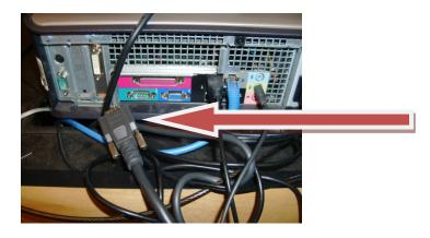
Plug the gray VGA cable back into the computer:
