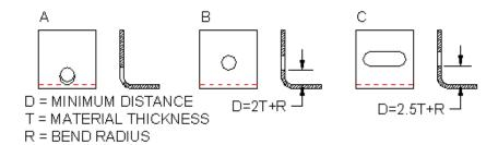
Form height to thickness ratio – To determine the minimum form height for sheet metal use the following formula: D = 2.5T + R (see below) The height can be less but it required secondary operations and is far more costly.
