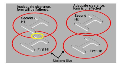
**Nibbling large radii** – When a large radius is required on a turret part the radius is made by making several hits with a flat tool. The angle and position of the tool changes as it moves around the edge simulating a large radius. The radius edge will have a "scalloped" look, tiny points formed where one flat is transitioned to another. The scalloped feature is pictured below. After deburring it is hardly perceivable, but still there.
