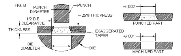
**Hole diameter to thickness ratio** – For most materials hole diameter should not be less than material thickness. As tensile strength increases the punch diameter must also increase.
