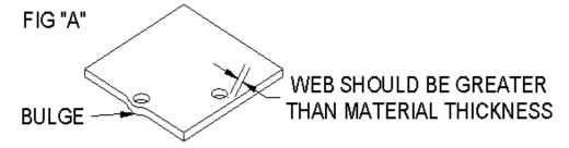
**Hole taper** – When a hole is punched it does not have a constant radius through the entire thickness of the part. The cross section of a punched hole is shown below. The taper in the bottom side of the hole is relative to the die clearance. Die clearance is the difference between the punch diameter and die diameter. It is usually about 10% of the material thickness. To get a constant diameter through the entire material thickness the part must be drilled, a far more costly operation.
