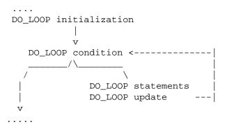
Because XAIF can preserve and exploit high level control structures such as DO\_LOOP, we want to *remove* the initialization and update statement so they can be placed in the special 'xaif:ForLoop' construct. More importantly, xaif2whirl also depends on this transformation.
