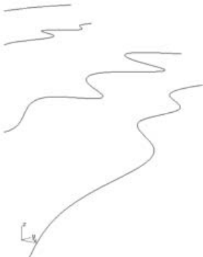
Contours lofted create strange horizontal bumps.
