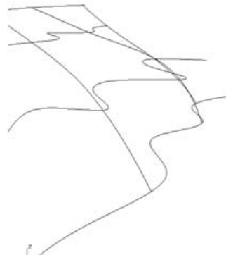
The same contours have regulating perpendicular lines added to them, NetworkSrf is used, and there are no bumps.
