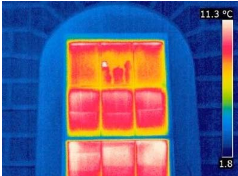
Image 6 Thermal Imaging of Single Glazed Window – Listed Building
