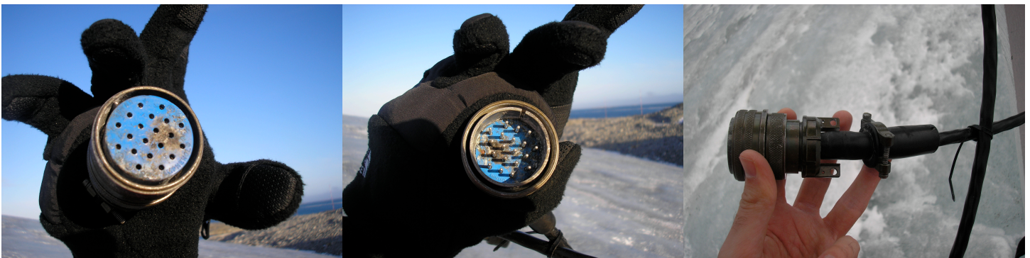
Figure 4 – The connectors at JB2. (a) Burn marks on the downhill connector. (b) Burn marks (and a missing pin) on the uphill connector. (c) Improper weatherproofing of the uphill connector.
