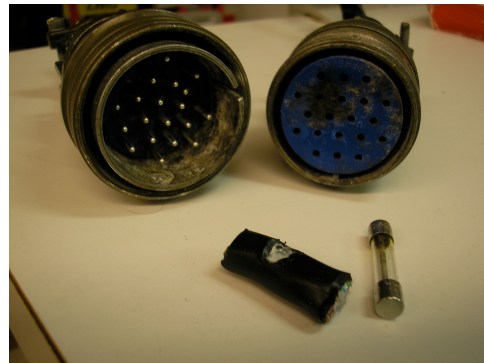
Figure 10 – The elements that caused the Antenna/Receiver system to fail.
