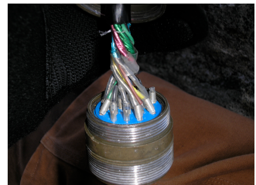
Figure 5 – The twisting damage exhibited on one of the JB1 connectors.
