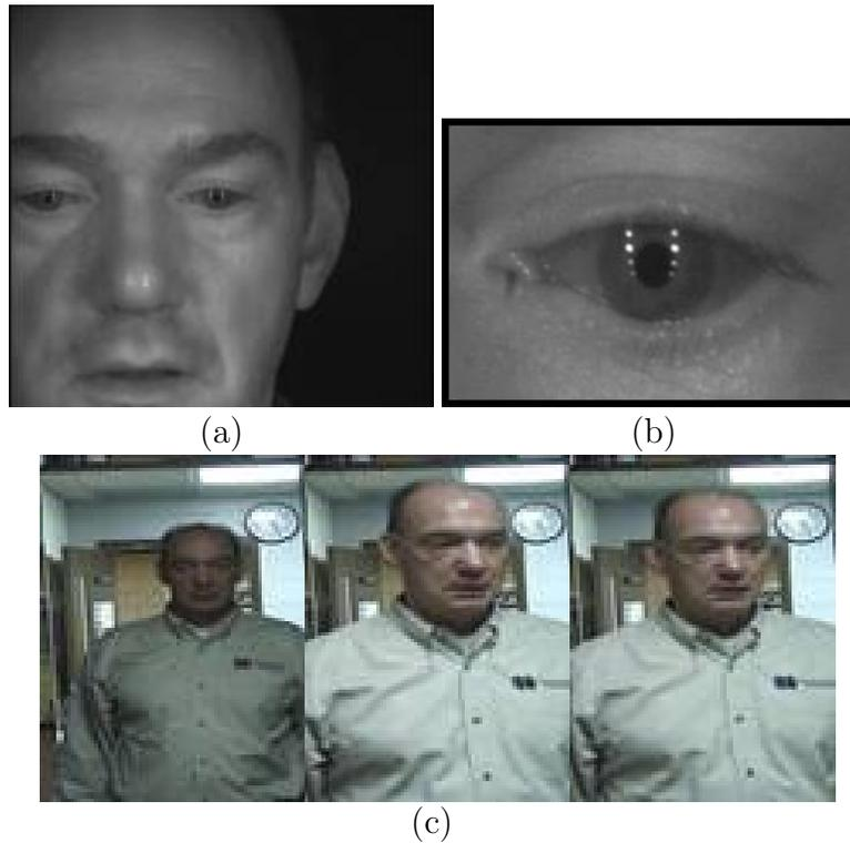
**Fig. 1.** Example of imagery collected as a subject walks through the portal. The image in (a) is a full 2,000 by 2,000 pixel NIR frame acquired by the IoM and (b) is the left ocular region from the frame in (a). There are approximately 120 pixels across the iris in (a) and (b). The images in (c) are three frames from an HD video sequence of a subject walking through the portal.
