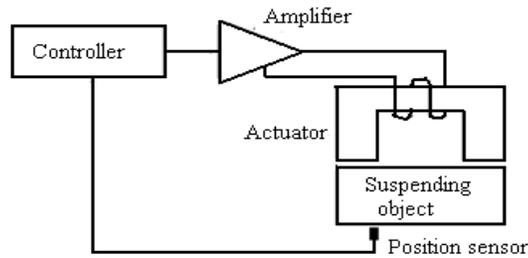
Figure 3. Basic block diagram of DC Electromagnetic levitation system
