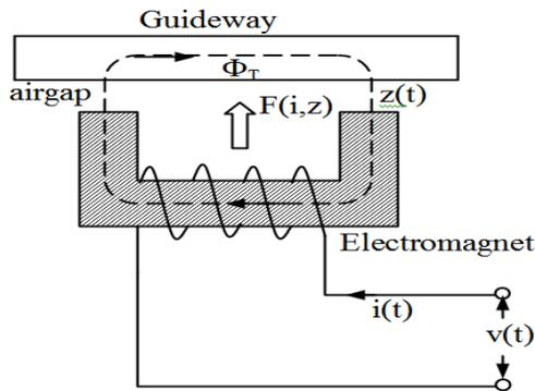
Figure 2. Simplified diagram of DC electromagnetic levitation system (inverted model)
