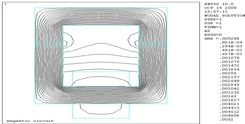
Figure 7. Flux pattern of U-U structure for 5mm air-gap
