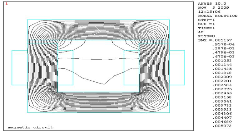
Figure 8. Flux pattern of U-I structure with two coils (upper side) for 5mm air-gap
