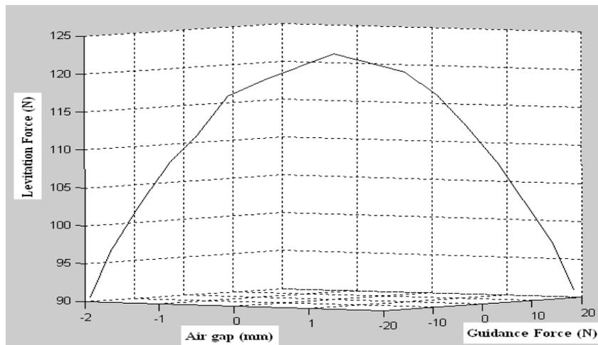
Figure 22. Levitation and guidance force vs. shifted distance (3D) for U-I structure
