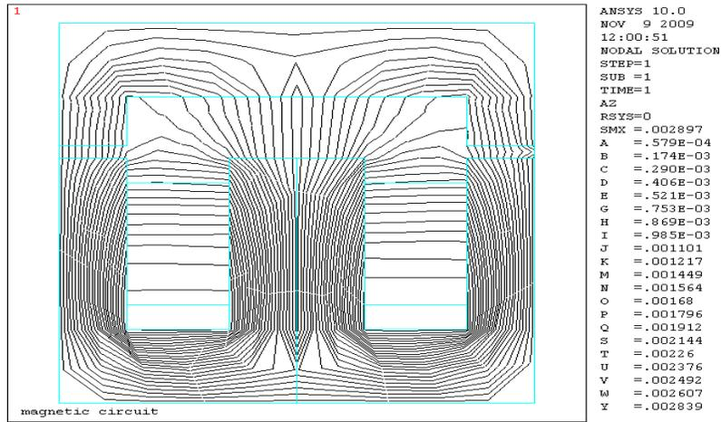
Figure 11. Flux pattern of E-U structure with single coil for 5mm air-gap
