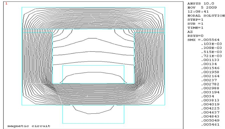
Figure 6. Flux pattern of U-I structure for 5mm air-gap
