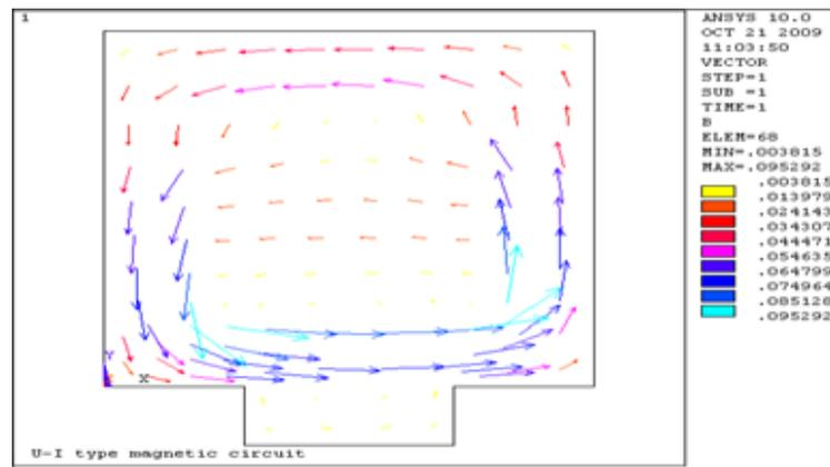
Figure 16. Flux density for U-I structure for 20 mm air-gap
