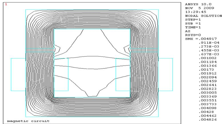
Figure 9. Flux pattern of U-U structure with two coils (upper side) for 5mm air-gap
