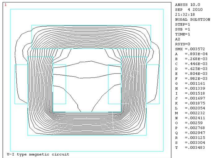
Figure 18. Flux for U-I structure where  $z=10$  mm,  $x=5$  mm (+ve shifting)
