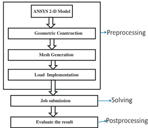
Figure 5. Flow chart for ANSYS simulation
