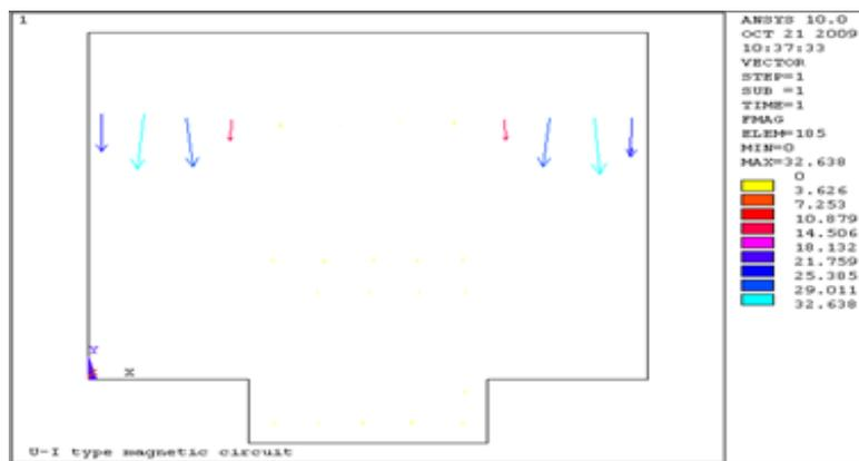
Figure 13. Force for U-I structure for 5 mm air-gap
