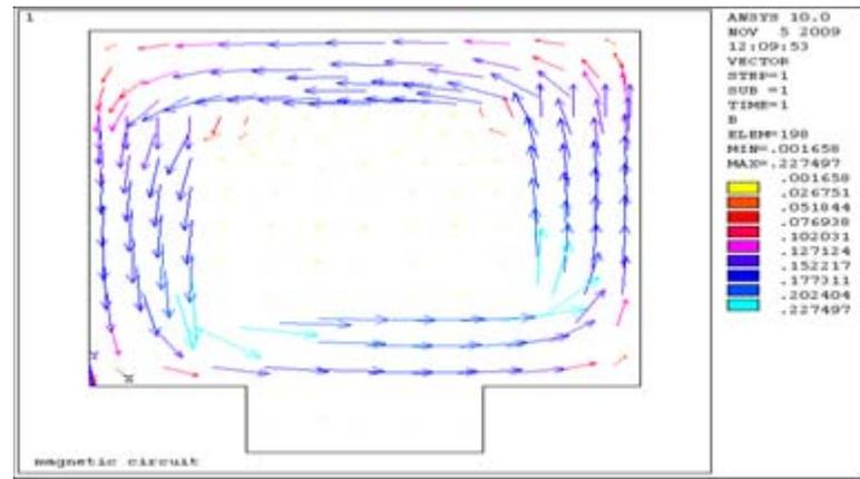
Figure 15. Flux density for U-I structure for 5 mm air-gap
