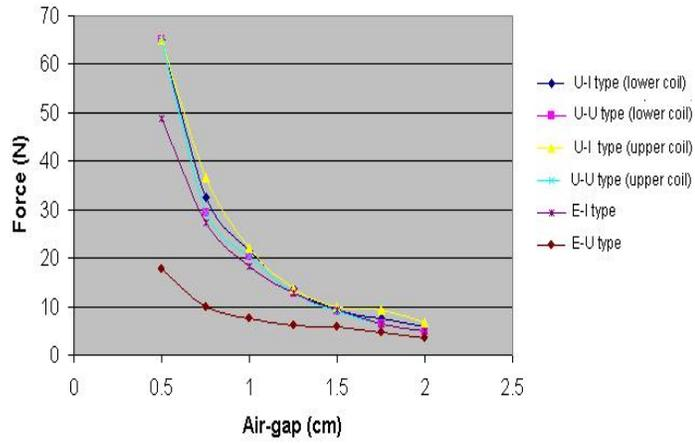
Figure 20. Force vs. air gap curve for different structures for different air-gap.
