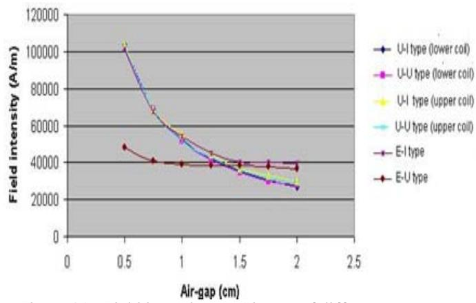
Figure 21. Field intensity vs. Air-gap of different structures
