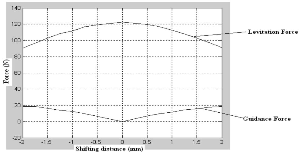
Figure 23. Levitation and guidance force vs. shifted distance (2D) for U-I structure
