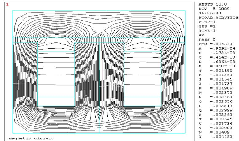
Figure 10. Flux pattern of E-I structure with single coil for 5mm air-gap
