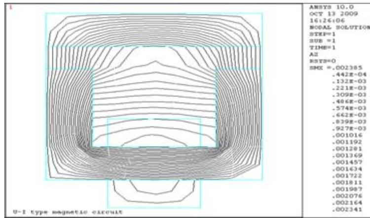
Figure 12. Flux pattern of U-I structure for 20 mm air-gap
