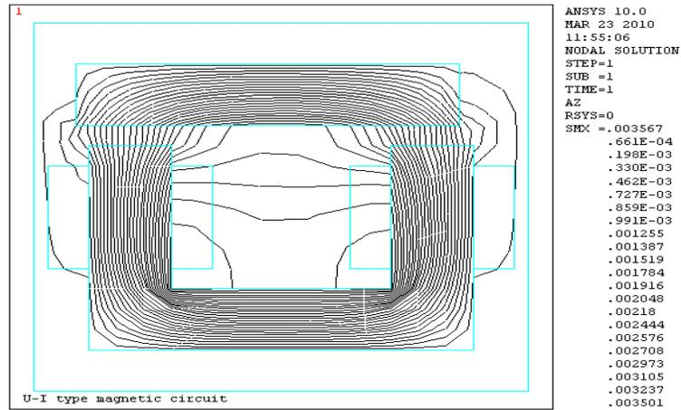
Figure 17. Flux for U-I structure where  $z=10$  mm,  $x=5$  mm (-ve shifting)
