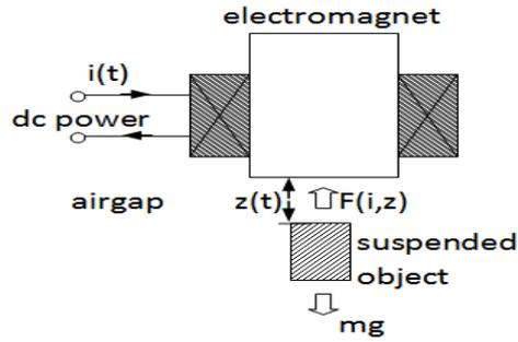
Figure 1. Simplified diagram of DC electromagnetic levitation system
