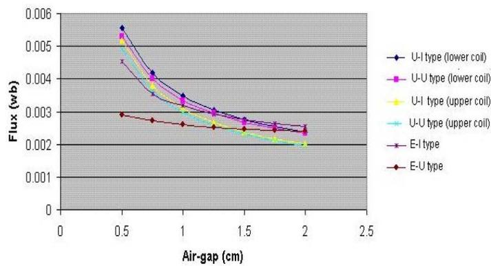
Figure 19. Flux vs. air gap curve for different structures for different air-gap
