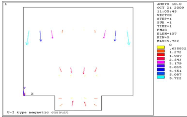
Figure 14. Force for U-I structure for 20 mm air-gap
