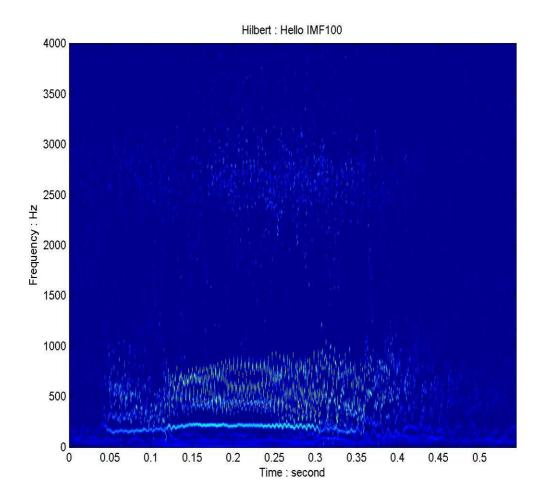
**Figure 17:** The Hilbert spectrum from the Ensemble EMD with added noise. The Mode mixing has disappeared. There are no transition gaps and all basic frequency traces are continuous in the time-frequency space.
