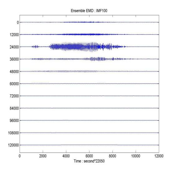
**Figure 15:** The IMFs (C1 to C11, from the top blue curve to the bottom blue curve, respectively) of digitalized sound "Hello" from the Ensemble EMD with added noise. The Mode mixing has all but disappeared. Each IMF component has consistent amplitudes and scales.
