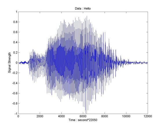
Figure 13: Digitalized sound of the word, 'Hello', at 22,050 Hz.
