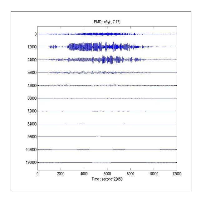
**Figure 14:** The IMFs (C1 to C11, from the top blue curve to the bottom blue curve, respectively) of digitalized sound "Hello" from the EMD without added noise. The Mode mixing has caused the second and third components to intersperse with sections of data having highly disparate amplitudes and scales.
