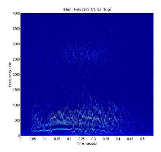
**Figure 16:** The Hilbert spectrum from the original EMD without added noise. The Mode mixing has caused numerous transition gaps, and rendered the time-frequency traces fragmented.
