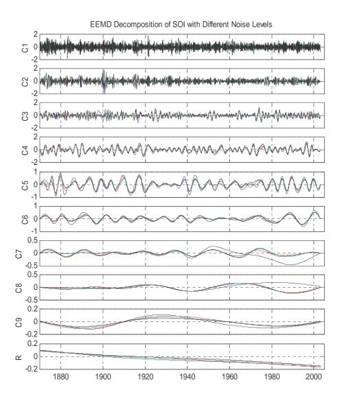
**Figure 11:** EEMD decompositions of SOI with added noise. Blue line corresponds is the standard decomposition using EMD without any added noise. Red, green, and black lines correspond to EEMD decompositions with added noise of standard deviation of 0.1, 0.2, and 0.4, respectively. The ensemble number for each case is 100.
