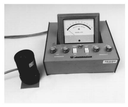
Figure 20.11 Reflectance meter (photovolt).
