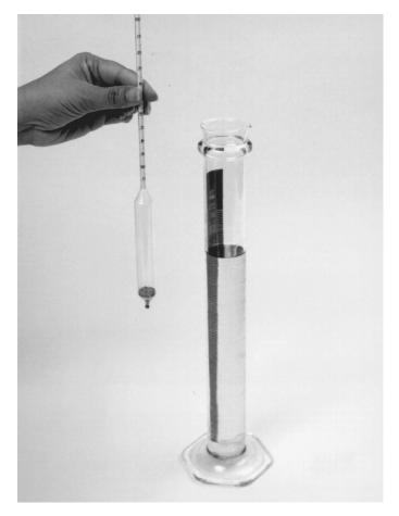
Figure 20.6 Hydrometer.
