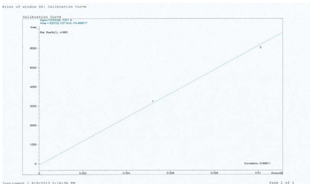
Figure 7. Calibration curve of alpha copane
